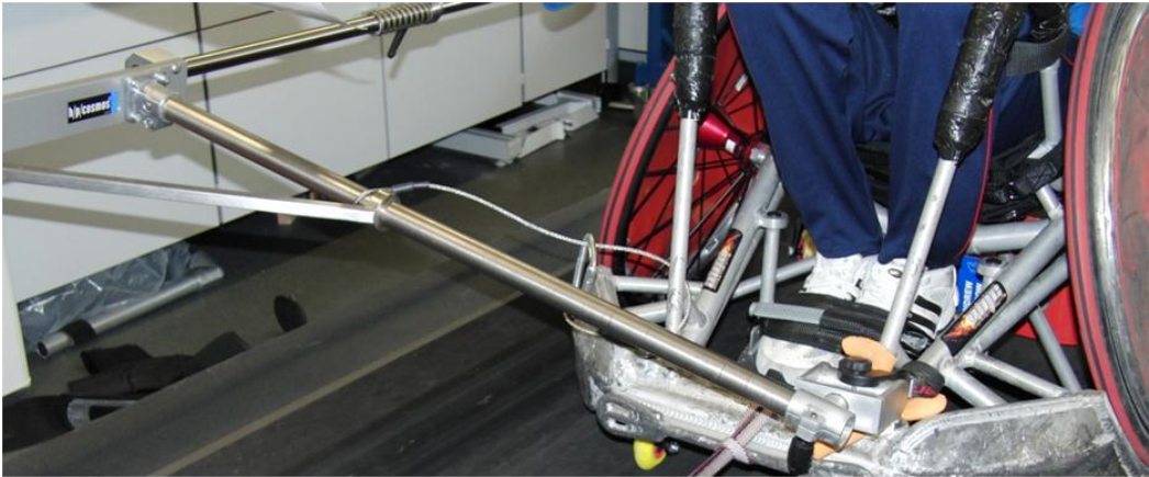
Fig 3-13 Method of securing the wheelchair to the treadmill.
