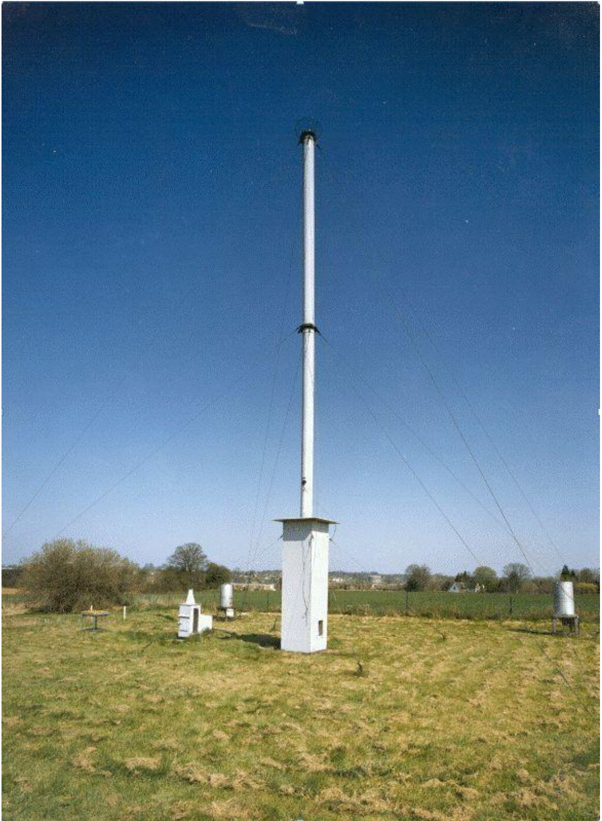
Figure 2.2. An aphid suction trap. (Photograph provided to AWS by Dr R. Harrington).
