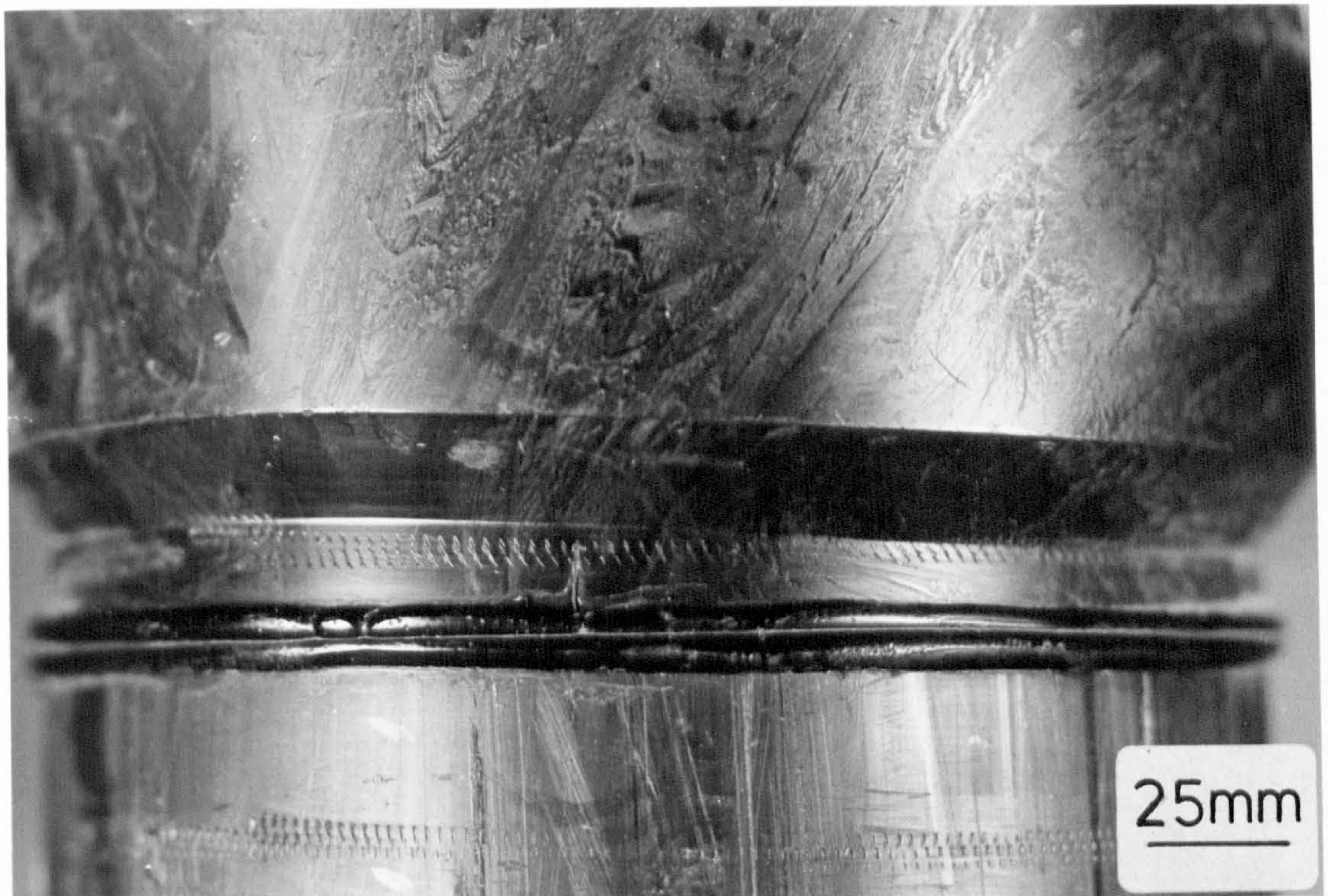
FIGURE 6.3b Example of the external appearance of a brittle fracture at a butt-weld between an injection moulded tee and extruded pipe (T2 type 1).
