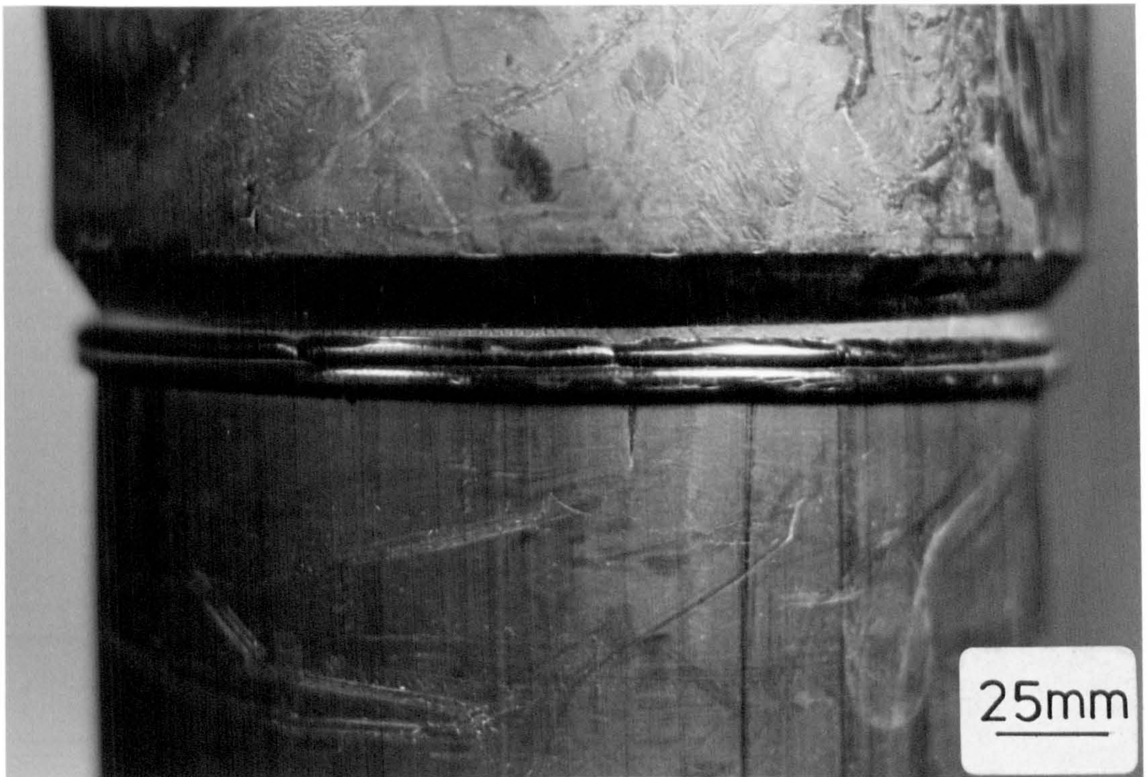
FIGURE 6.3a Example of the external appearance of a brittle fracture at a butt-weld between an injection moulded tee and extruded pipe (T2 type 1).
