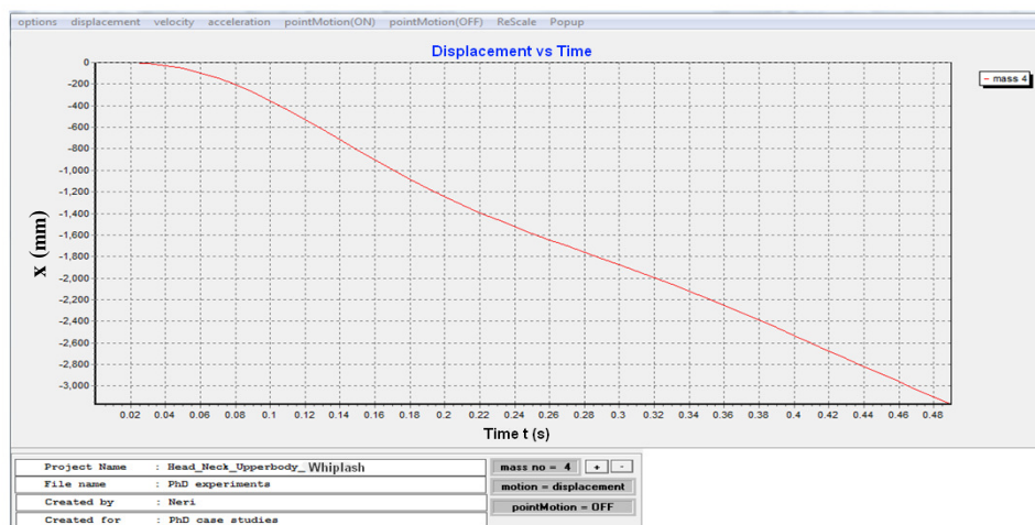
Figure 5.8 (a) Half Sine acceleration constraint shock acting on T1, the graph shows mass no 4, head movement
