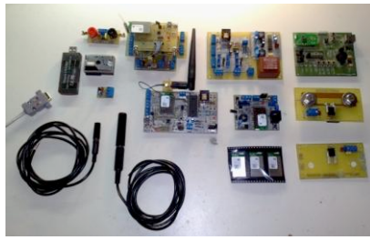
Figure 2: Monitoring system hardware.
