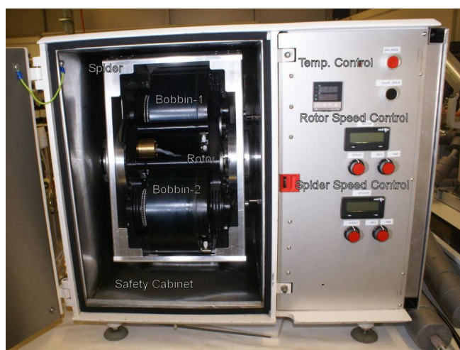
Figure 7.3.1: A photo of the interior of the non synchronous CCC machine. Typically the rotor speed would be kept constant at 800rpm. The spider speed control is changed to attain the appropriate Pr ratio for the run.
