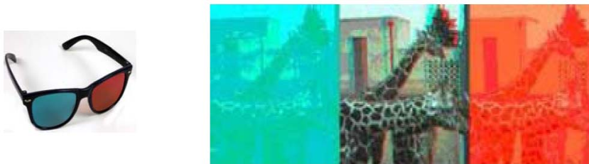
Figure 3-9: Anaglyph glasses and anaglyph image [27].
