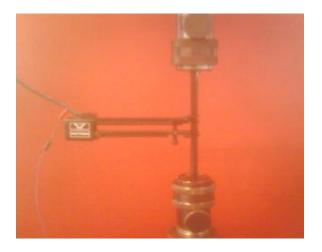
Fig: 4.10. The extensioneter-device that acquires the elastic modulus can be seen strapped to the test sample. See also the bolt head and the slip ring.
