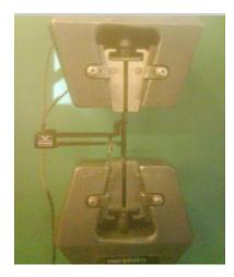
Fig: 4.23. The V grips- the fixture that secured the tubular test sample in place. The inner sections have V grooves that ensure better gripping of the sample. See attached also the extensioneter.
