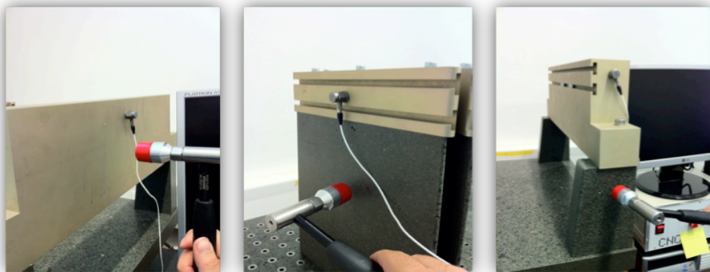
Figure 6.4: Positions of accelerometers and excitation points.
