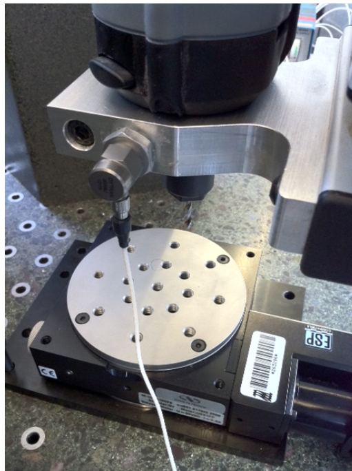
Figure 6.12: Rotary stages configuration with a spindle attached.
