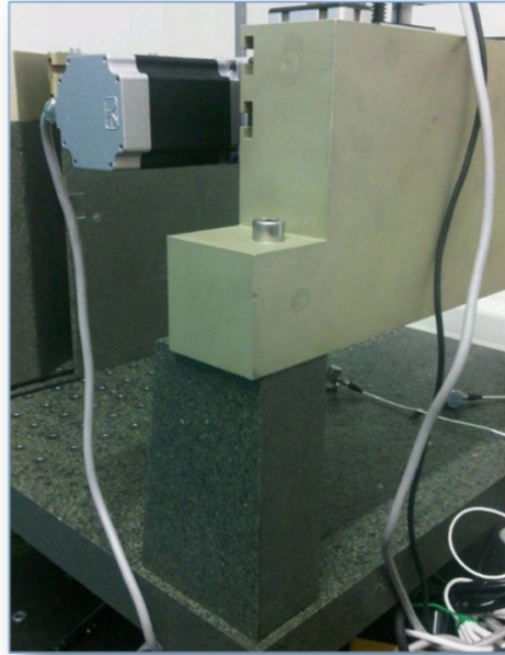
Figure 5.11: Assembled gantry structure.
