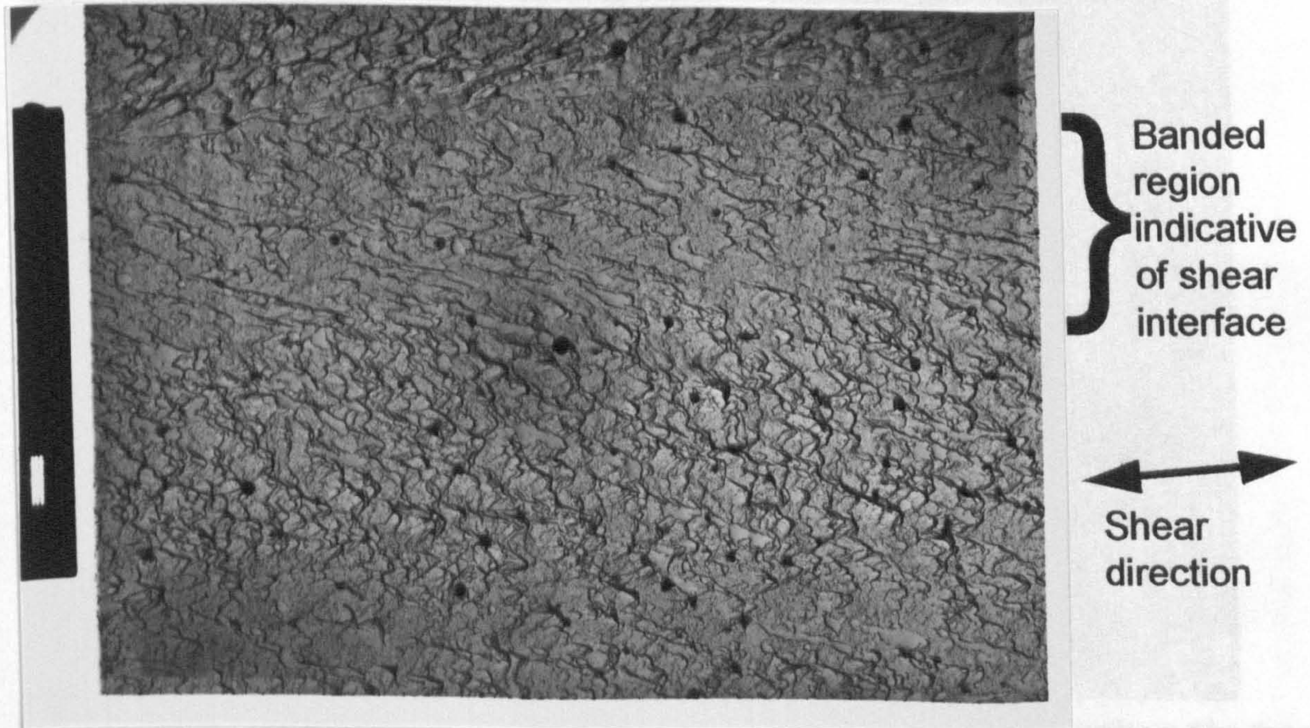
Figure 4.8 TEM micrograph viewed perpendicular to flow of the shear region of an iPP SCORIM moulding. The moulding was produced using 5 shears with no delay inbetween them. The directional change of the flow has been encapsulated within this microstructure as banded regions. Scale bar 2 \mu m.
