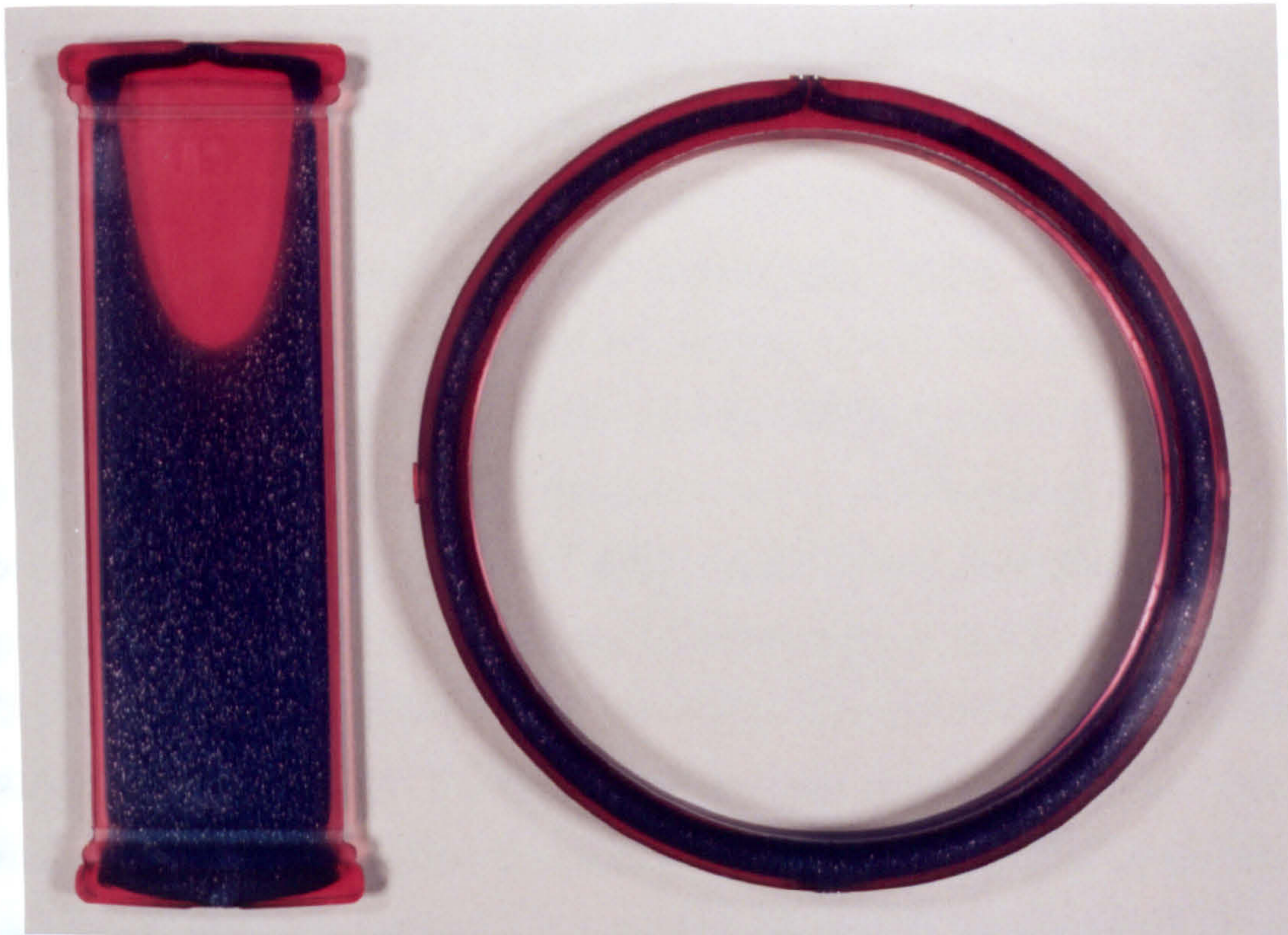
Figure 3.32 Two two-colour mouldings which demonstrate the potential application for SCORIM to be used for the insertion of recyclate (e.g. the blue material) into a virgin skin (e.g. the red material) after initially filling the mould cavity with the skin material.
