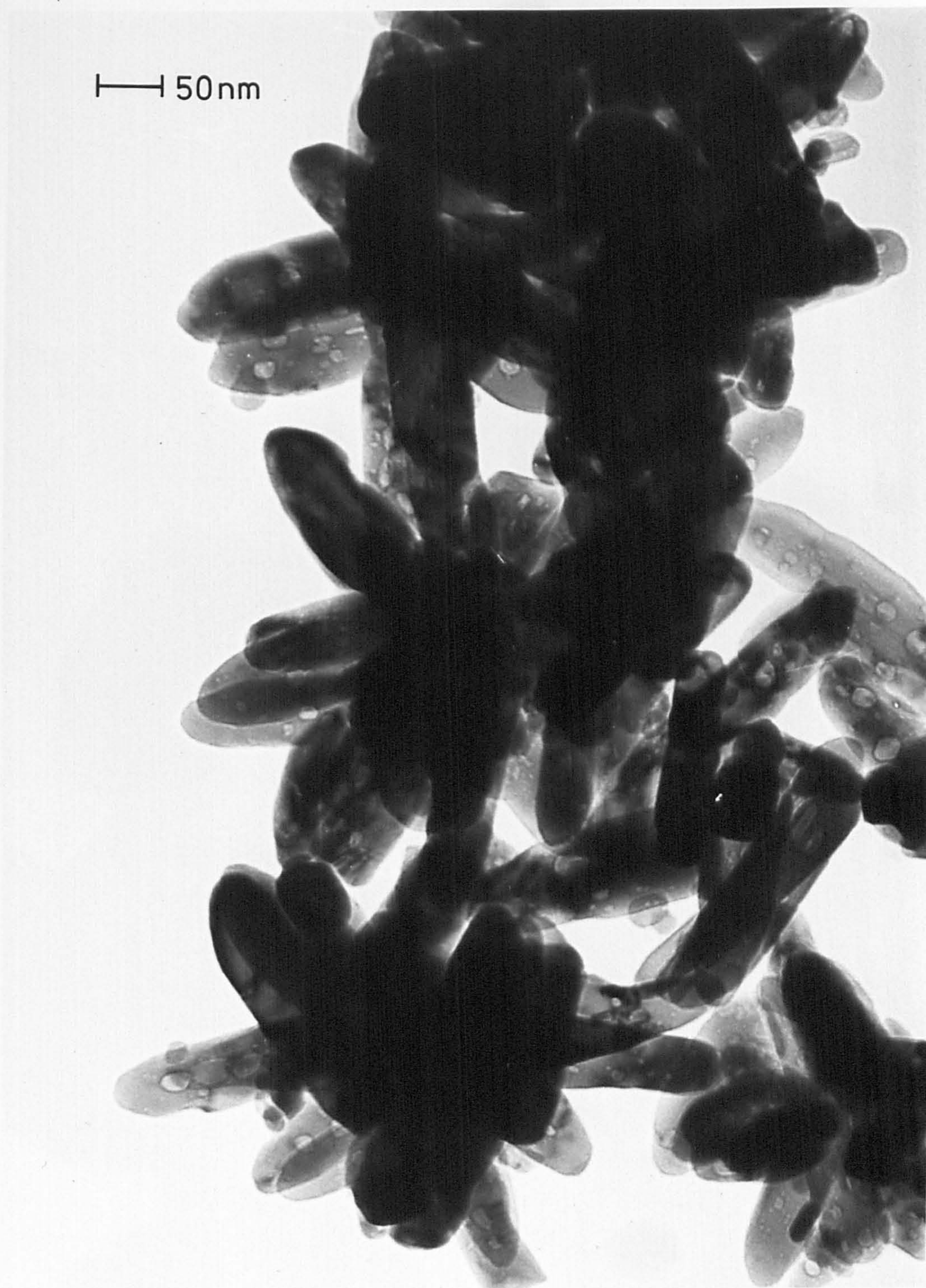
FIGURE 3-1 Transmission Electron Micrograph (magnification 200,000) BASE RUTILE [CL/D702]
