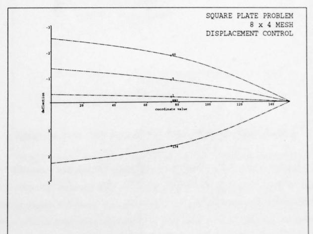
Figure 7.8. Mode shapes along the transverse axis of the perfect plate using the  $8 \times 4$  mesh.
