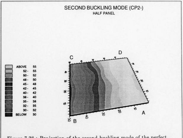
Figure 7.38: Projection of the second buckling mode of the perfect shell at CP2- for the  $8\times 8$  mesh (deformations magnified by factor 5).
