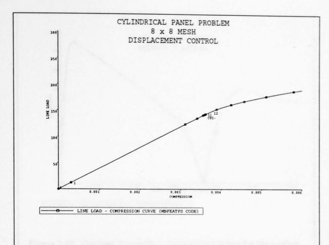
Figure 7.24. Line load - compression curve for the perfect shell using the  $8 \times 8$  mesh.
