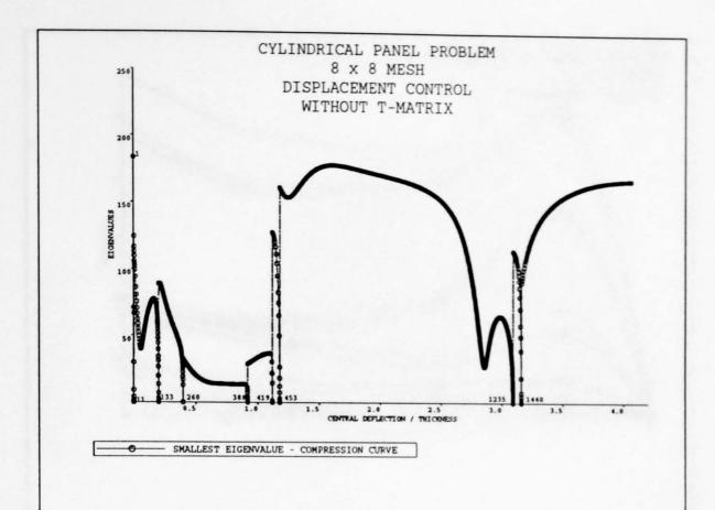
Figure 7.32. Smallest eigenvalue - compression curve for the perfect shell using the  $8 \times 8$  mesh (without T-matrix, *i.e.* eigenvalues  $\theta^{(r)}$  calculated from  $\mathbf{K_T}\boldsymbol{\xi}^{(r)} = \theta^{(r)}\boldsymbol{\xi}^{(r)}$  (no sum on r))
