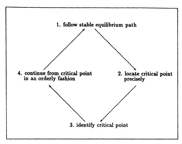
The emphasis in the present work is given to the continuation from bifurcation points since no generally valid method has been developed for this. Limit points can be handled without difficulty by employing the arc length technique as mentioned earlier.
