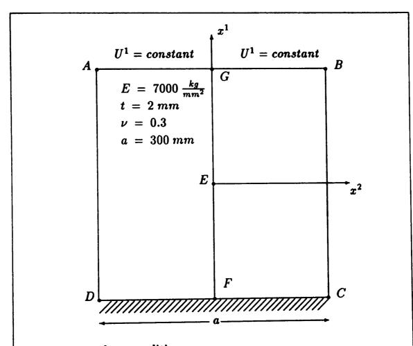
Boundary conditions:  $AB : U^{1} = constant, U^{2} = U^{3} = \frac{\partial U^{3}}{\partial n} = 0$   $DC : U^{1} = U^{2} = U^{3} = \frac{\partial U^{3}}{\partial n} = 0$   $BC, AD : U^{3} = \frac{\partial U^{3}}{\partial n} = 0$
