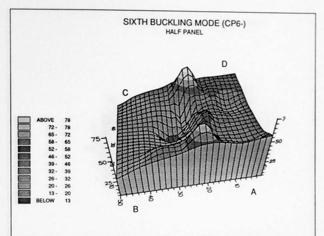
Figure 7.45: Asymmetric sixth buckling mode of the perfect shell at CP6- for the  $8\times 8$  mesh (deformations magnified by factor 5).
