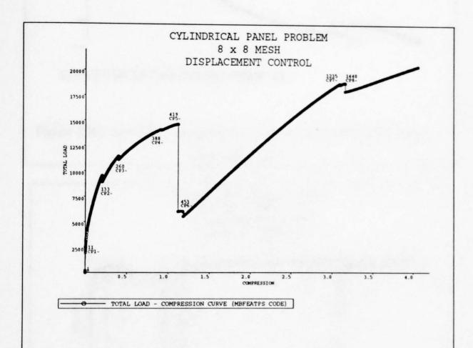
Figure 7.29. Total load - compression curve for the perfect shell using the  $8\times 8$  mesh.
