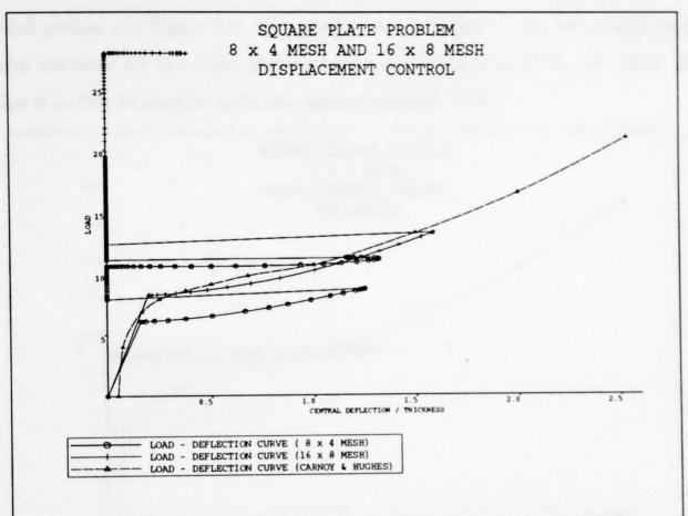
Figure 7.14. Mesh comparison of load - deflection curves for the perfect plate using the  $8 \times 4$  and the  $16 \times 8$  mesh.
