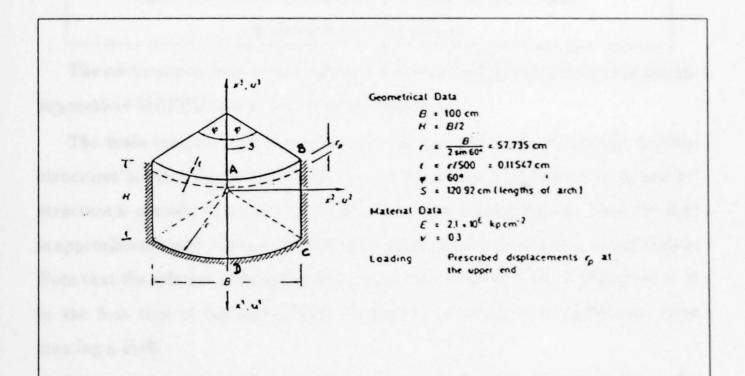
Figure 7.21: Cylindrical panel: material and geometrical data and boundary conditions.
