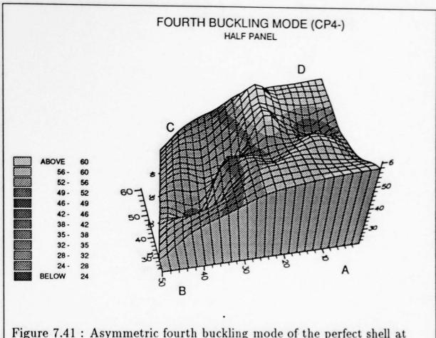
Figure 7.41: Asymmetric fourth buckling mode of the perfect shell at CP4- for the  $8\times 8$  mesh (deformations magnified by factor 5).
