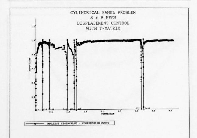
Figure 7.31. Smallest eigenvalue - compression curve for the perfect shell using the  $8 \times 8$  mesh (with T-matrix, *i.e.* eigenvalues  $\theta^{(r)}$  calculated from  $\mathbf{K_T}\boldsymbol{\xi}^{(r)} = \theta^{(r)}\mathbf{T}\boldsymbol{\xi}^{(r)}$  (no sum on r))
