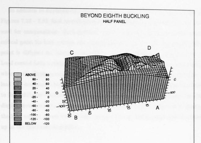
Figure 7.51: Asymmetric mode shape at a point beyond the eighth buckling mode of the perfect shell for the  $8 \times 8$  mesh (deformations magnified by factor 5).
