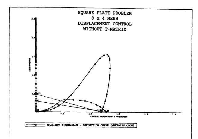
Figure 7.5. Smallest eigenvalue - deflection curve for the perfect plate using the  $8 \times 4$  mesh (without T-matrix, *i.e.* eigenvalues  $\theta^{(r)}$  calculated from  $\mathbf{K_T} \boldsymbol{\xi^{(r)}} = \theta^{(r)} \boldsymbol{\xi^{(r)}}$  (no sum on r)).
