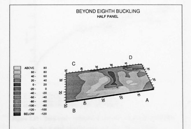
Figure 7.52: Projection of the mode shape at a point beyond the eighth buckling mode of the perfect shell for the  $8 \times 8$  mesh (deformations magnified by factor 5).
