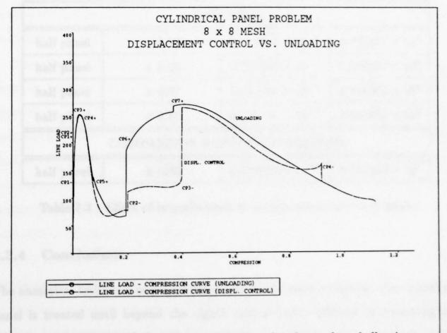
Figure 7.56: Line load - compression curve for the perfect shell using the  $8 \times 8$  mesh (displacement control vs. unloading).
