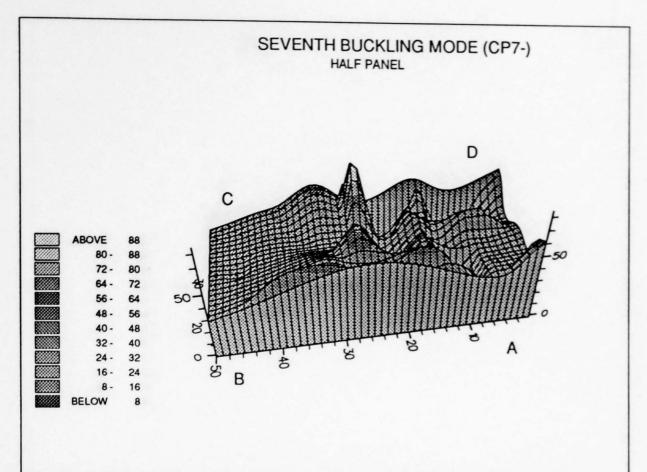
Figure 7.47: Asymmetric seventh buckling mode of the perfect shell at CP7- for the  $8\times 8$  mesh (deformations magnified by factor 5).
