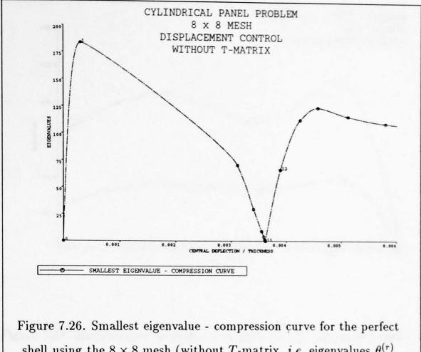
Figure 7.26. Smallest eigenvalue - compression curve for the perfect shell using the  $8 \times 8$  mesh (without T-matrix, *i.e.* eigenvalues  $\theta^{(r)}$  calculated from  $\mathbf{K_T}\boldsymbol{\xi}^{(r)} = \theta^{(r)}\boldsymbol{\xi}^{(r)}$  (no sum on r))
