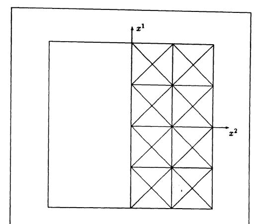
Figure 7.2. Half a plate modelled using the  $8 \times 4$  mesh.
