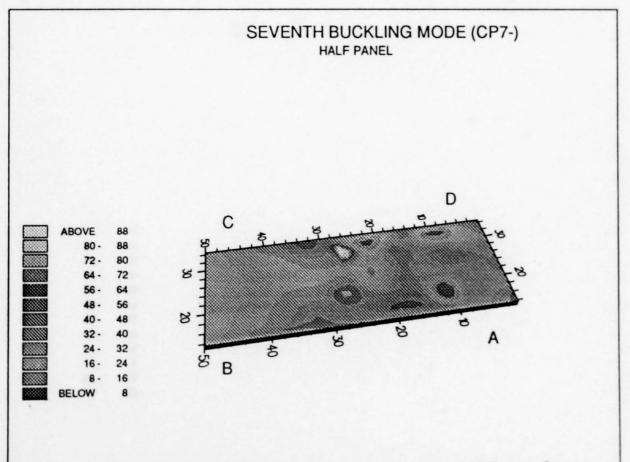
Figure 7.48: Projection of the seventh buckling mode of the perfect shell at CP7- for the  $8\times 8$  mesh (deformations magnified by factor 5).
