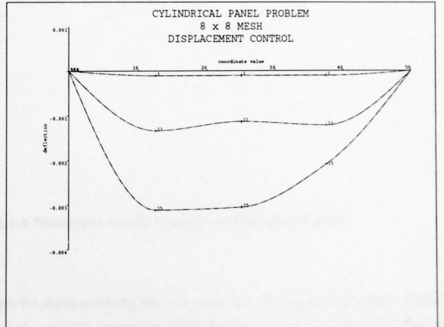
Figure 7.27. Mode shapes along the longitudinal axis for the perfect shell using the  $8 \times 8$  mesh.
