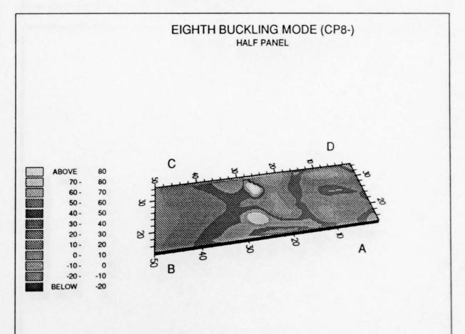
Figure 7.50: Projection of the eighth buckling mode of the perfect shell at CP8- for the  $8\times 8$  mesh (deformations magnified by factor 5).
