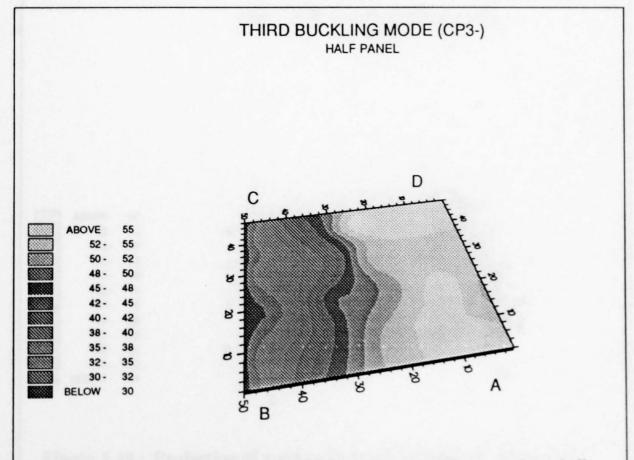
Figure 7.40: Projection of the third buckling mode of the perfect shell at CP3- for the  $8\times 8$  mesh (deformations magnified by factor 5).
