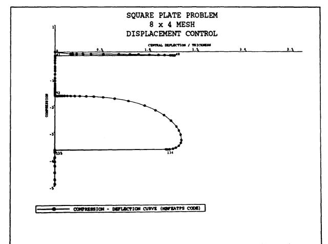
Figure 7.6. Compression - deflection curve for the perfect plate using the  $8 \times 4$  mesh.
