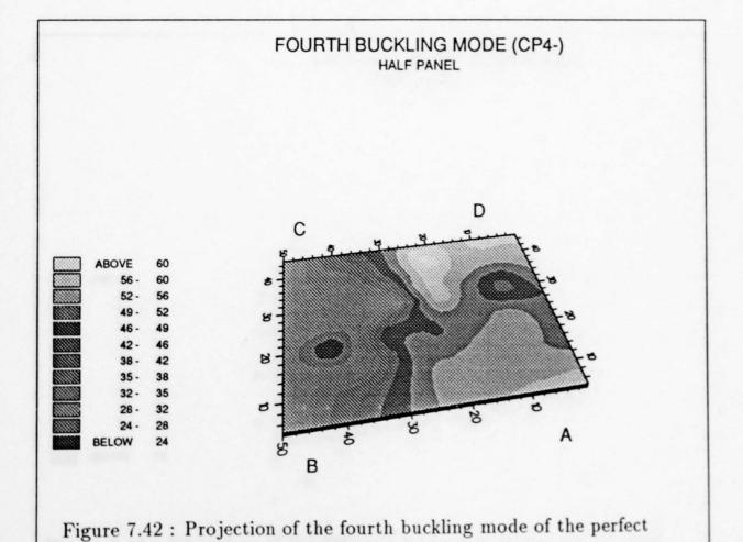
shell at CP4- for the  $8\times 8$  mesh (deformations magnified by factor 5).
