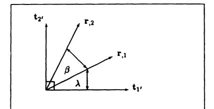
Figure 2.1. Base and unit orthogonal tangent vectors at a point of the surface.
