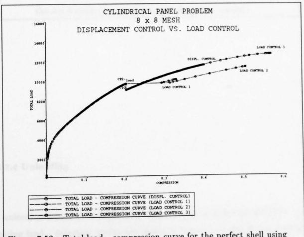
Figure 7.53: Total load - compression curve for the perfect shell using the 8 × 8 mesh (displacement control vs. load control).
