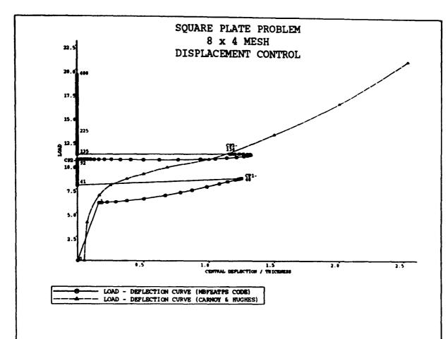
Figure 7.3. Load - deflection curve for the perfect plate using the  $8 \times 4$  mesh.
