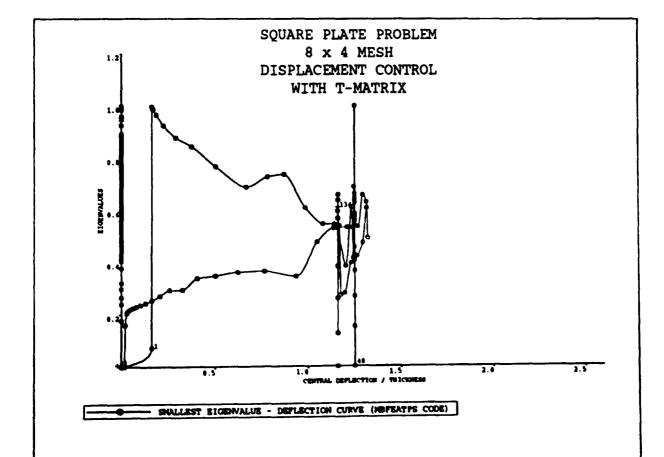
Figure 7.4. Smallest eigenvalue - deflection curve for the perfect plate using the  $8 \times 4$  mesh (with T-matrix, i.e. eigenvalues  $\theta^{(r)}$  calculated from  $\mathbf{K_T} \boldsymbol{\xi^{(r)}} = \theta^{(r)} \mathbf{T} \boldsymbol{\xi^{(r)}}$  (no sum on r)).
