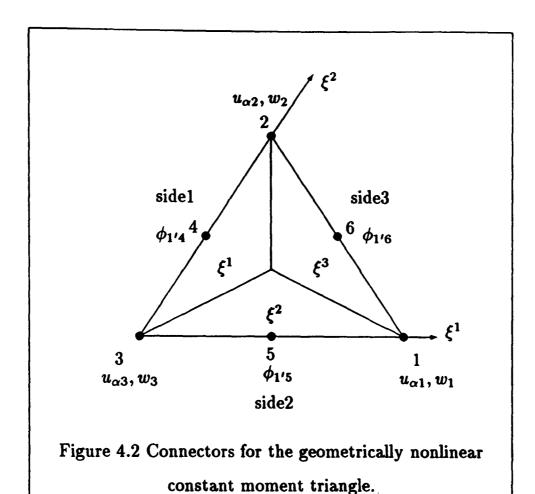
It is readily observed that for passing the patch test the  $u_{\alpha}$  and w must be cubic and quadratic polynomials, respectively. On the interelement boundaries, the in-plane displacements  $\tilde{u}_{\alpha}$  and the deflection  $\tilde{w}$  vary linearly whereas the normal rotation  $\tilde{\phi}_{1'}$  is assumed to be constant along each side. The modified generalized Hu-Washizu variational principle with the constant strain tensor  $\tilde{\gamma}_{\alpha\beta}$  is defined by
