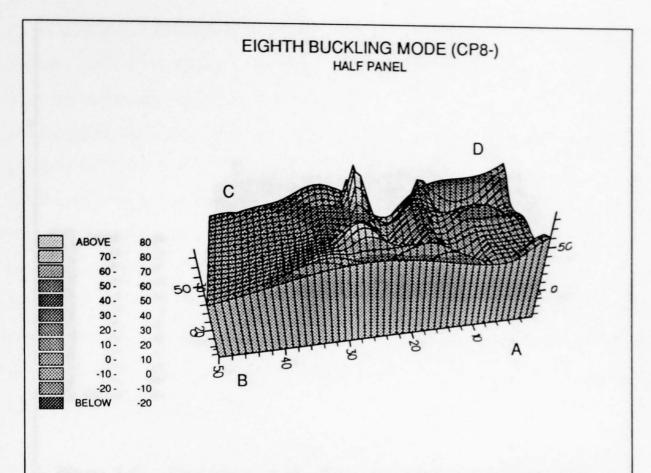
Figure 7.49: Asymmetric eighth buckling mode of the perfect shell at CP8- for the  $8\times 8$  mesh (deformations magnified by factor 5).
