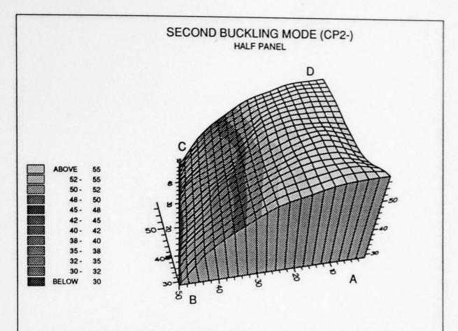
Figure 7.37: Asymmetric second buckling mode of the perfect shell at CP2- for the  $8\times 8$  mesh (deformations magnified by factor 5).
