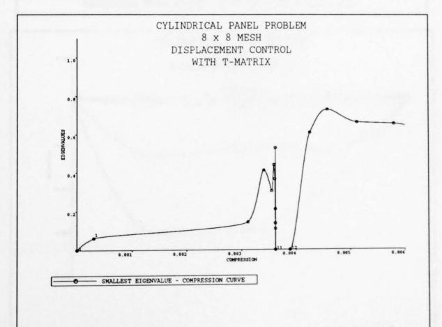
Figure 7.25. Smallest eigenvalue - compression curve for the perfect shell using the  $8 \times 8$  mesh (with T-matrix, *i.e.* eigenvalues  $\theta^{(r)}$  calculated from  $\mathbf{K_T}\boldsymbol{\xi}^{(r)} = \theta^{(r)}\mathbf{T}\boldsymbol{\xi}^{(r)}$  (no sum on r))
