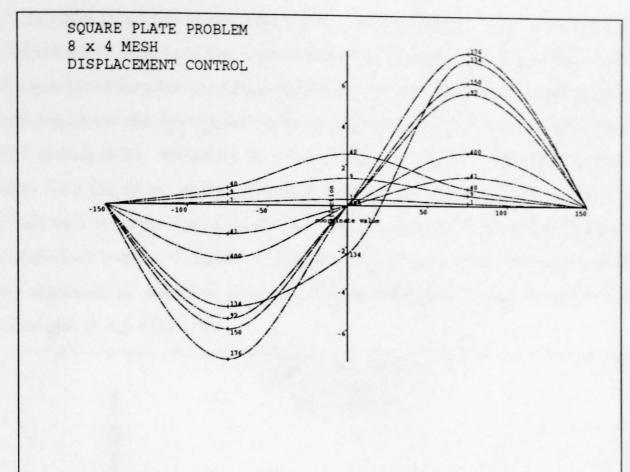
Figure 7.7. Mode shapes along the longitudinal axis of the perfect plate using the  $8\times 4$  mesh.
