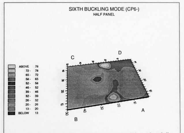
Figure 7.46: Projection of the sixth buckling mode of the perfect shell at CP6- for the  $8\times 8$  mesh (deformations magnified by factor 5).
