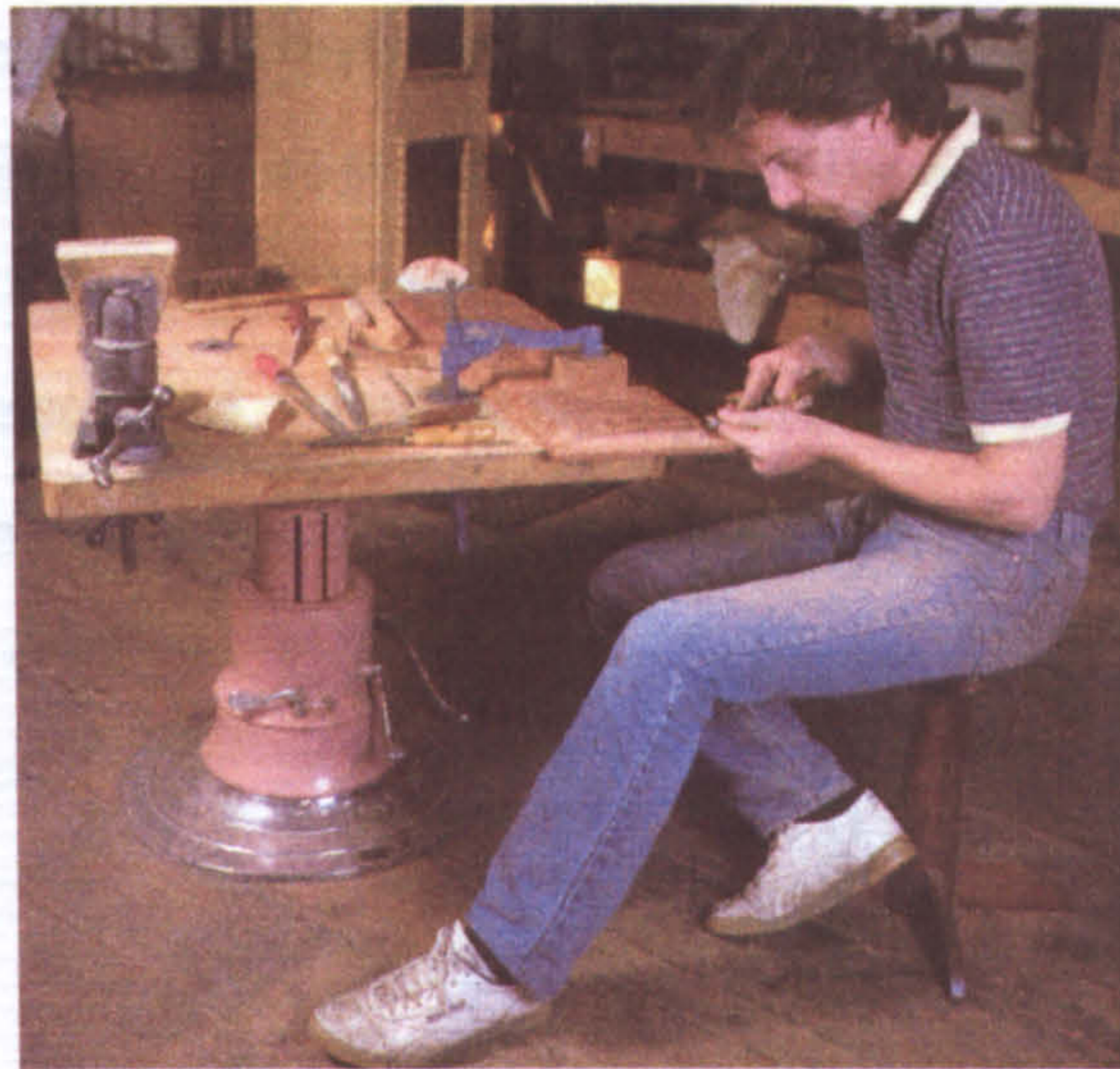
Figure 2-8 A purpose made adjustable bench. (Landis 1998)
