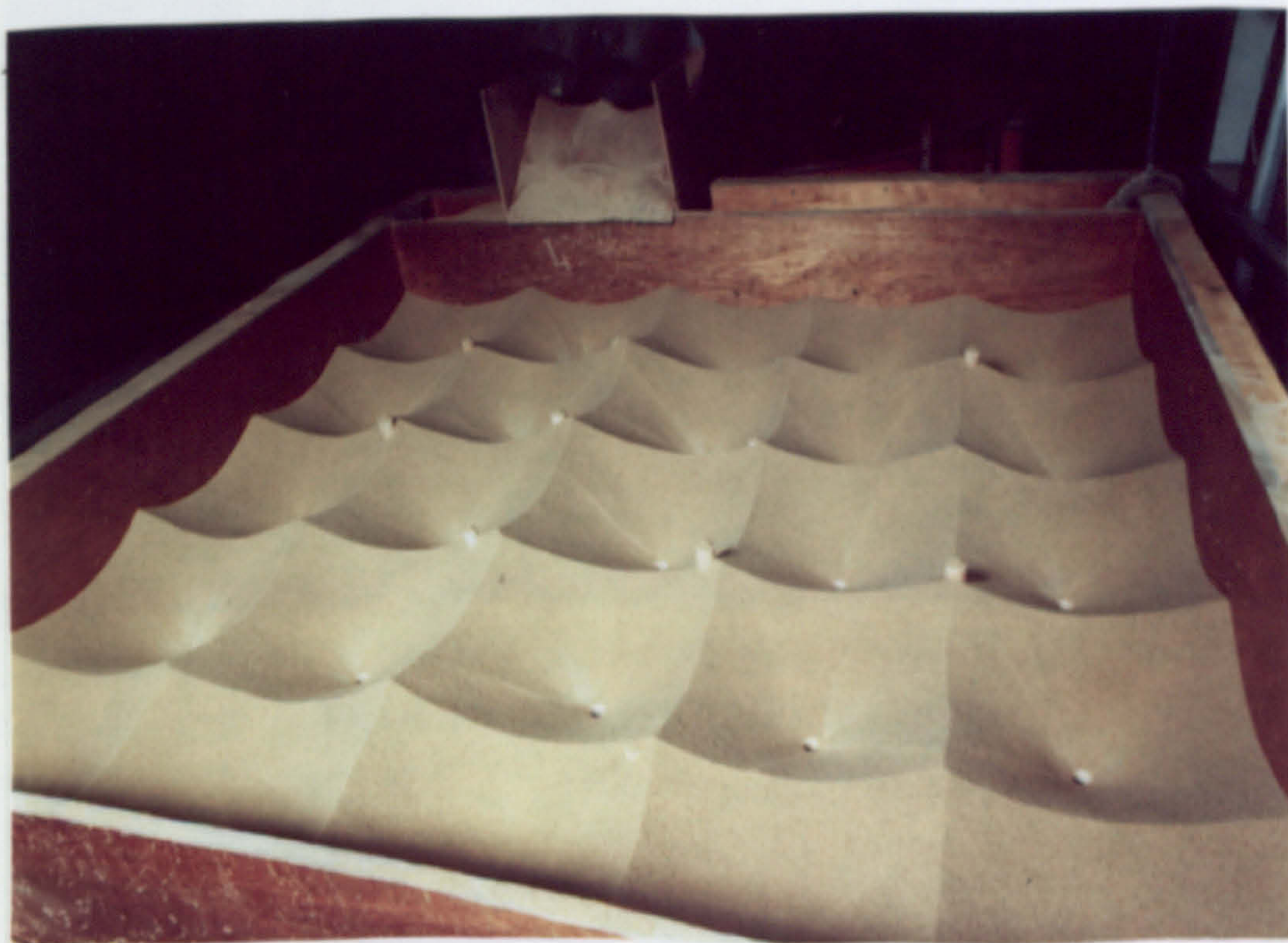
Figure 4.4(b) FILLER BOX AFTER DISCHARGE
