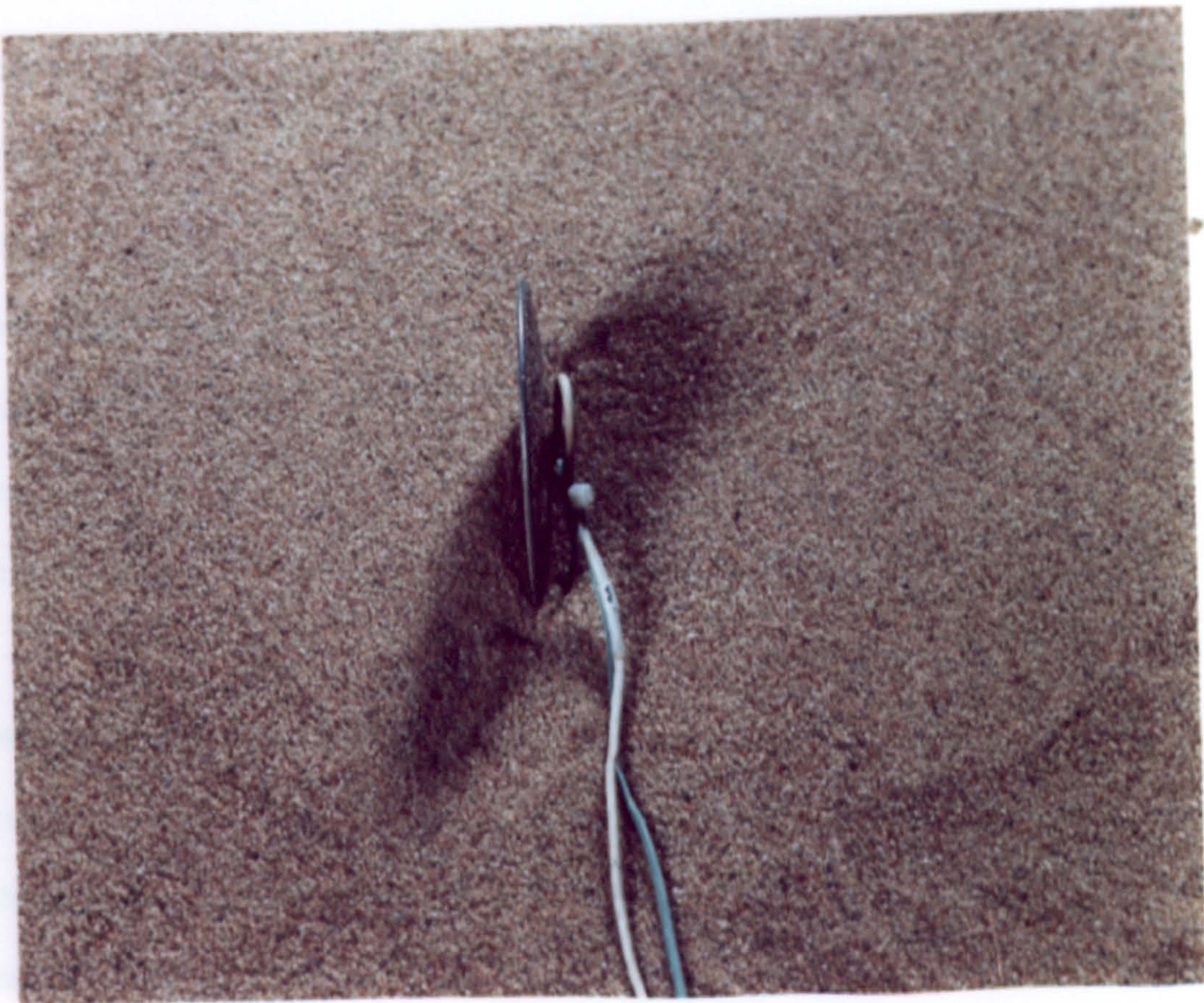
Figure 5.4(b) EMBEDDED CELL PLACED TO MEASURE HORIZONTAL PRESSURE
