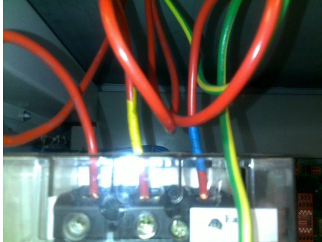
Fig. 3.3 Three phase power supply of the Bridgeport CNC milling machine
