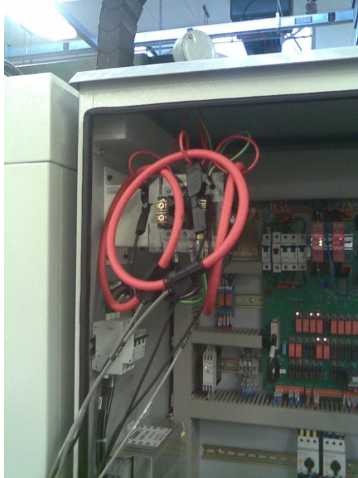
Fig. 6.1 The connection of the measurement device with the CNC machine
