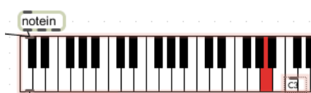
Fig. 1.8 The notein and kslider objects to enable the use of a MIDI controller keyboard
