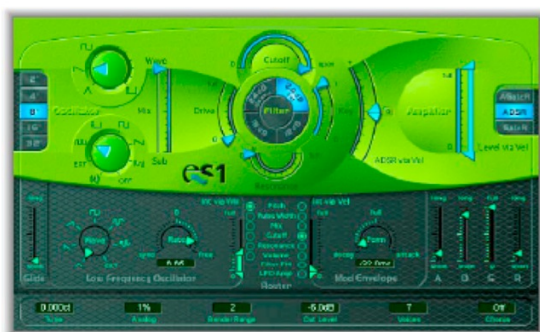
Fig 4.1 Logics ES1 synthesiser. Notice the ADSR envelope on the right hand side (see Tutorial 3)
