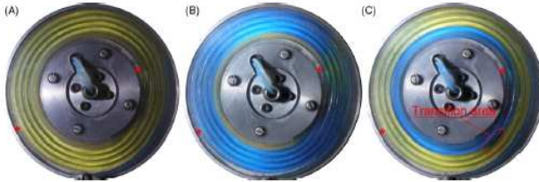
Fig. 4. Picture of the coil spinning at 1000 rpm with 4B phase system and the phases at equilibrium at: (A) 50 ml/min for both the upper phase and the lower phase; (B) 150 ml/min for the upper phase and 50 ml/min lower phase flow rates; and (C) 85 ml/min for the upper phase flow rate and 10 ml/min for the lower phase flow rate. The asterisks mark the location of the coil terminals.
