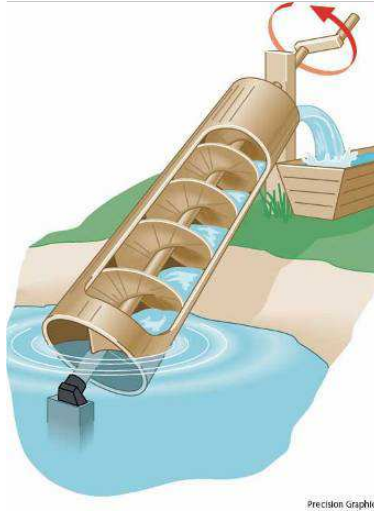
Figure 1-7: Archimedean screw used to pump up water 1 .
