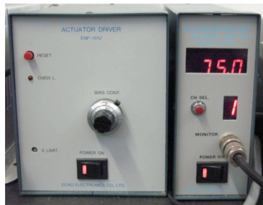
Figure 5.6 - Actuator driver ENP-1-1U (Echo Electronics) and actuator monitor unit ENP-50U (Echo Electronics).
