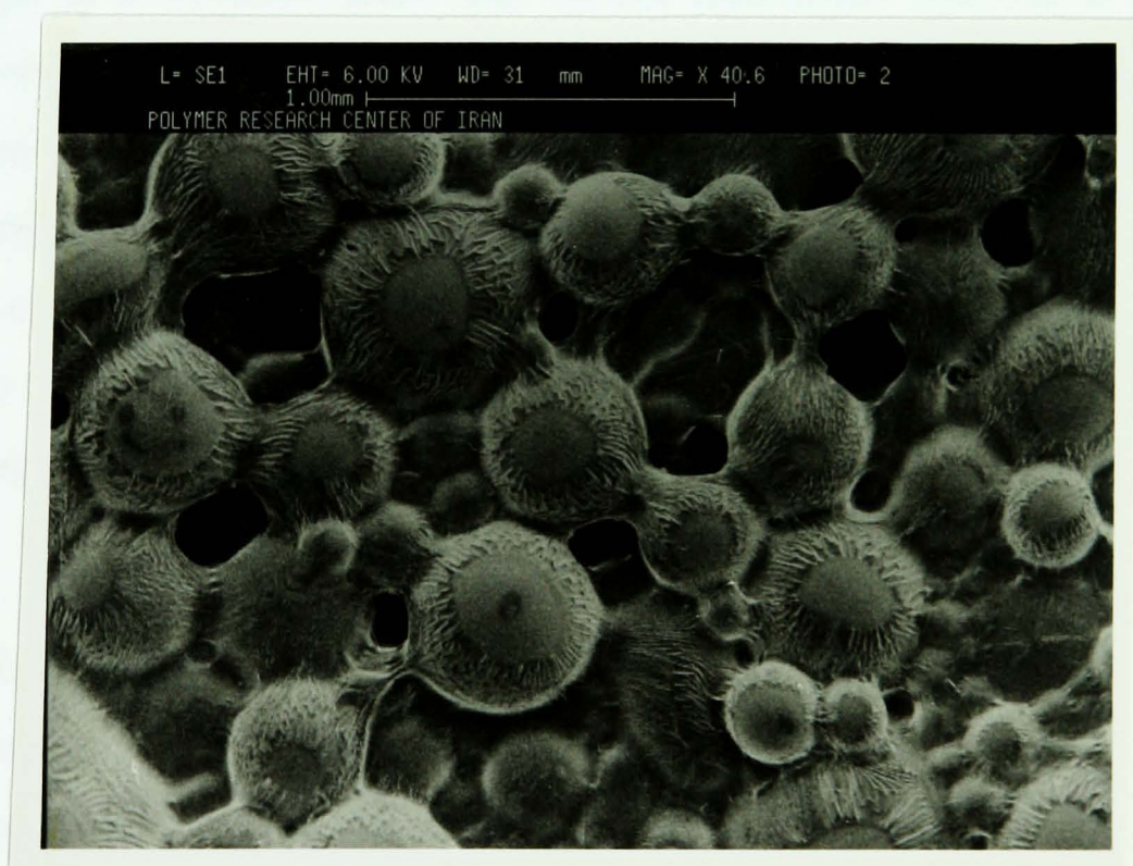
Figure 3.6 SEM micrograph of a sample obtained in Expt. 15, clearly shows the presence of ethyl cellulose over the polymer surface.
