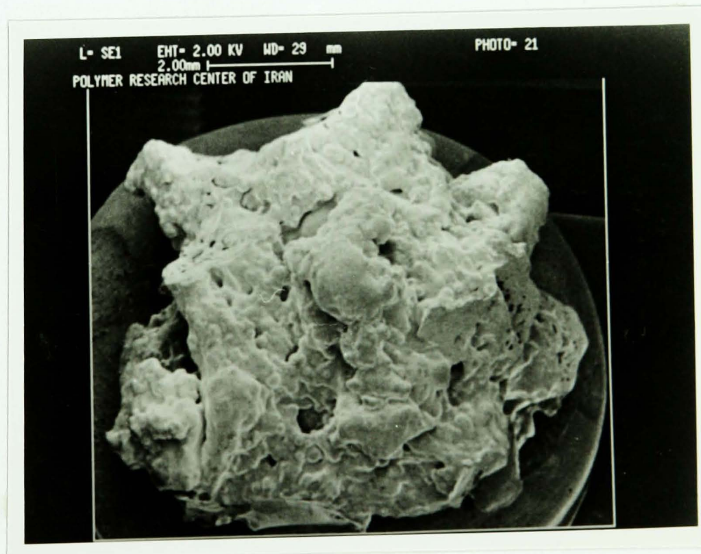
Figure 3.2 SEM micrograph of an isolated star-shaped granule obtained from the Expt. 7.
