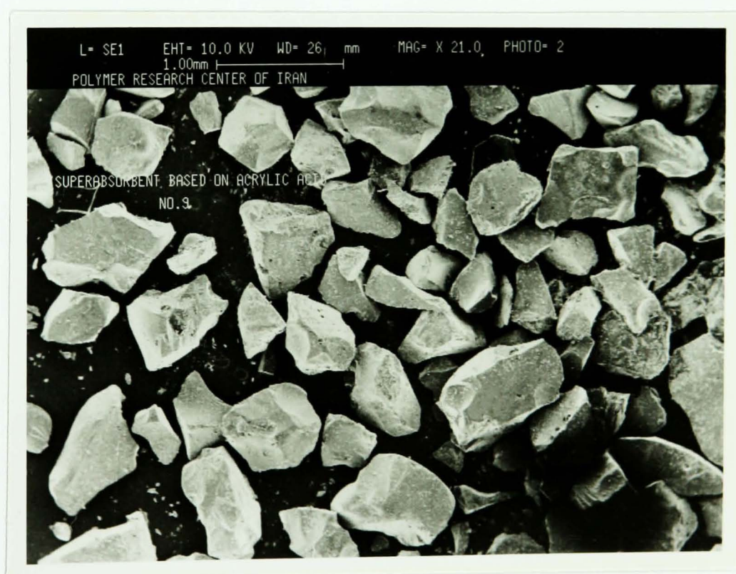
Figure 3.4 SEM micrograph of ground-up absorbent obtained from the Expt. 14.
