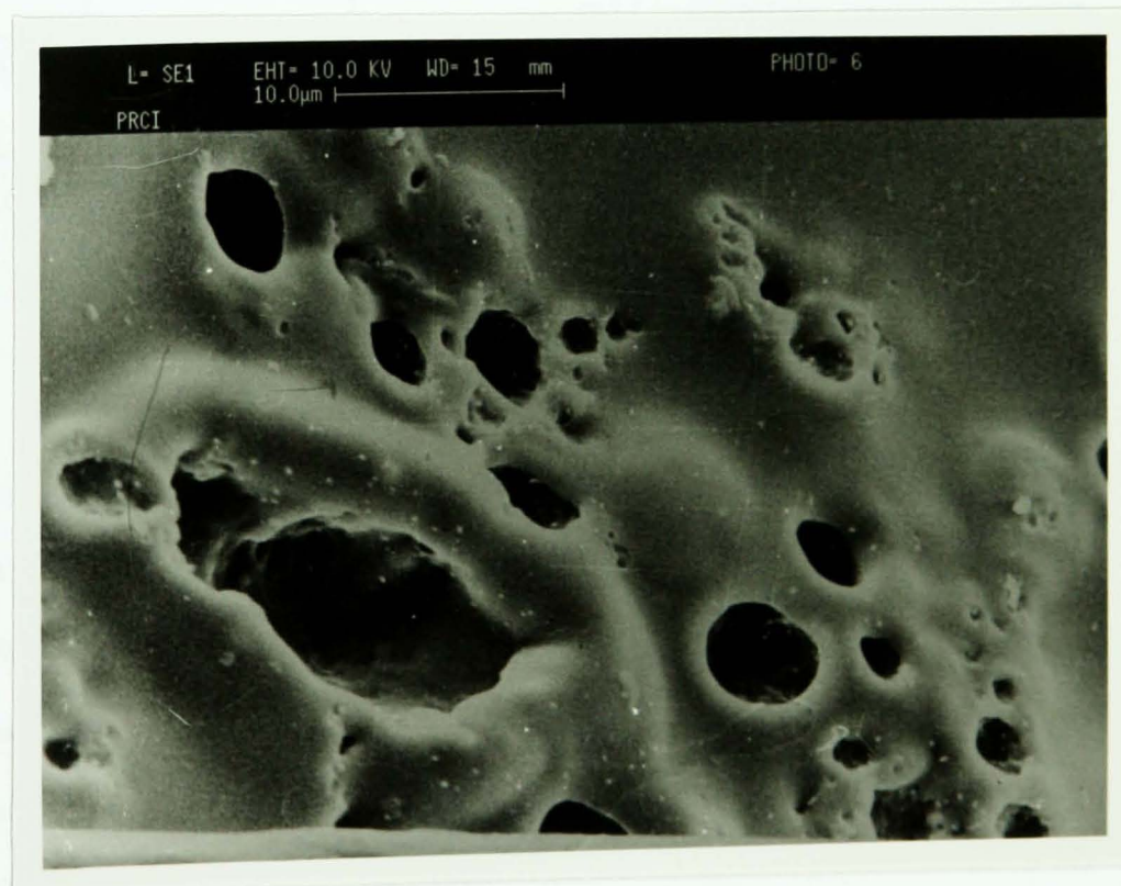
Figure 3.56: Micrograph of an PVC-contained sample which has been extracted with tetrahydrofuran.
