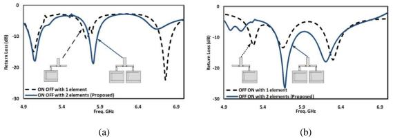
Fig.3 (a) The effect of adding an absorber between the patches (b) The effect of the combined impedance on the wideband performance Case 1 is 500hm Case 2 is 680hm and Case 3 is 86 0hm
