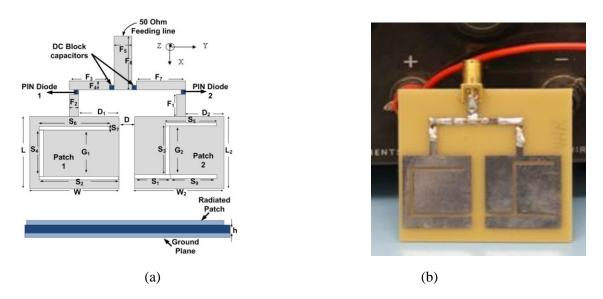
Fig. 1 (a) Configuration of the proposed microstrip antenna (b) Fabricated prototype
