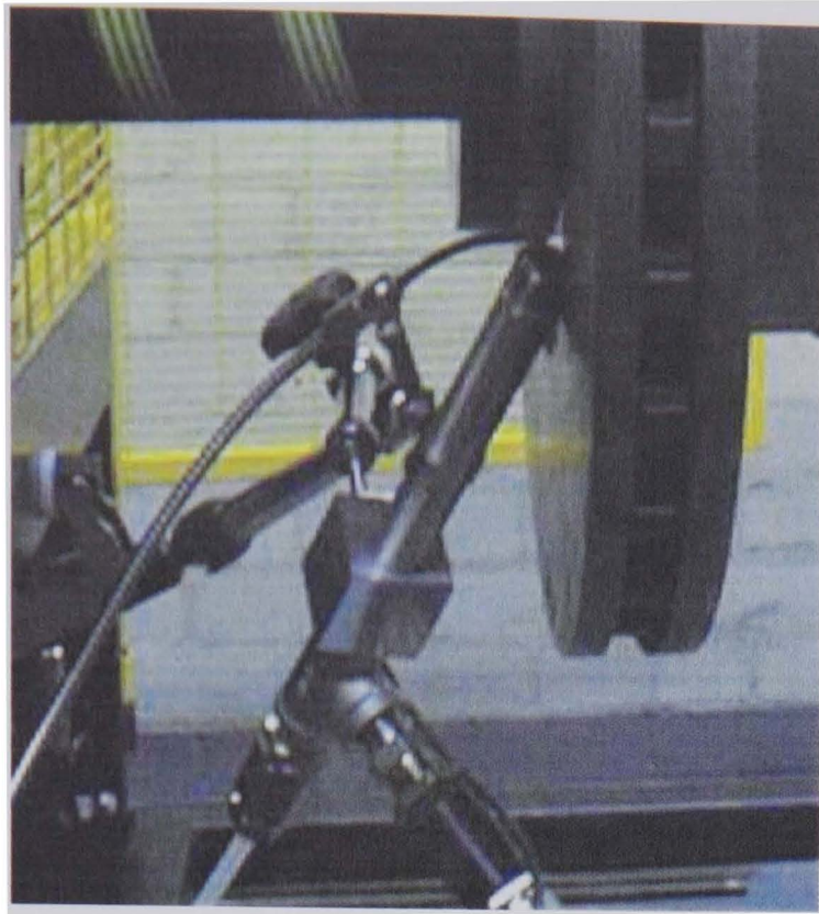
Figure D14 Heating of ventilated CV disc with air heater
