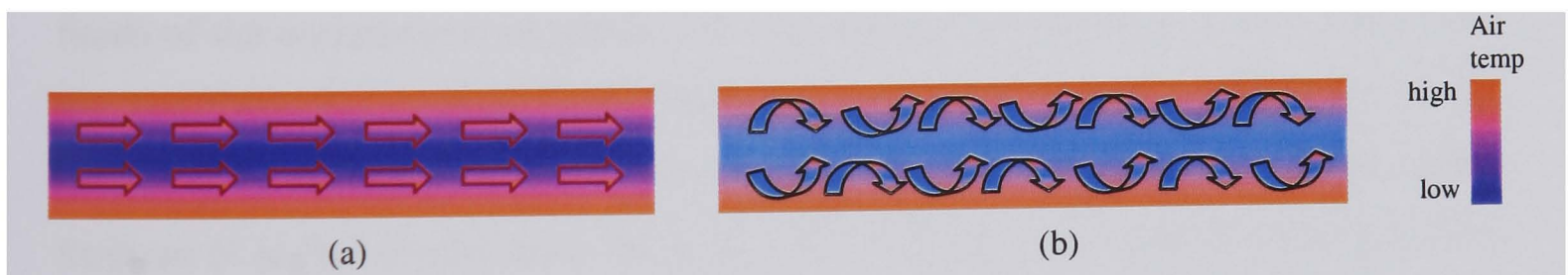
Figure 9.1 (a) Laminar and (b) turbulent airflow heat dissipation of the ventilation channel
