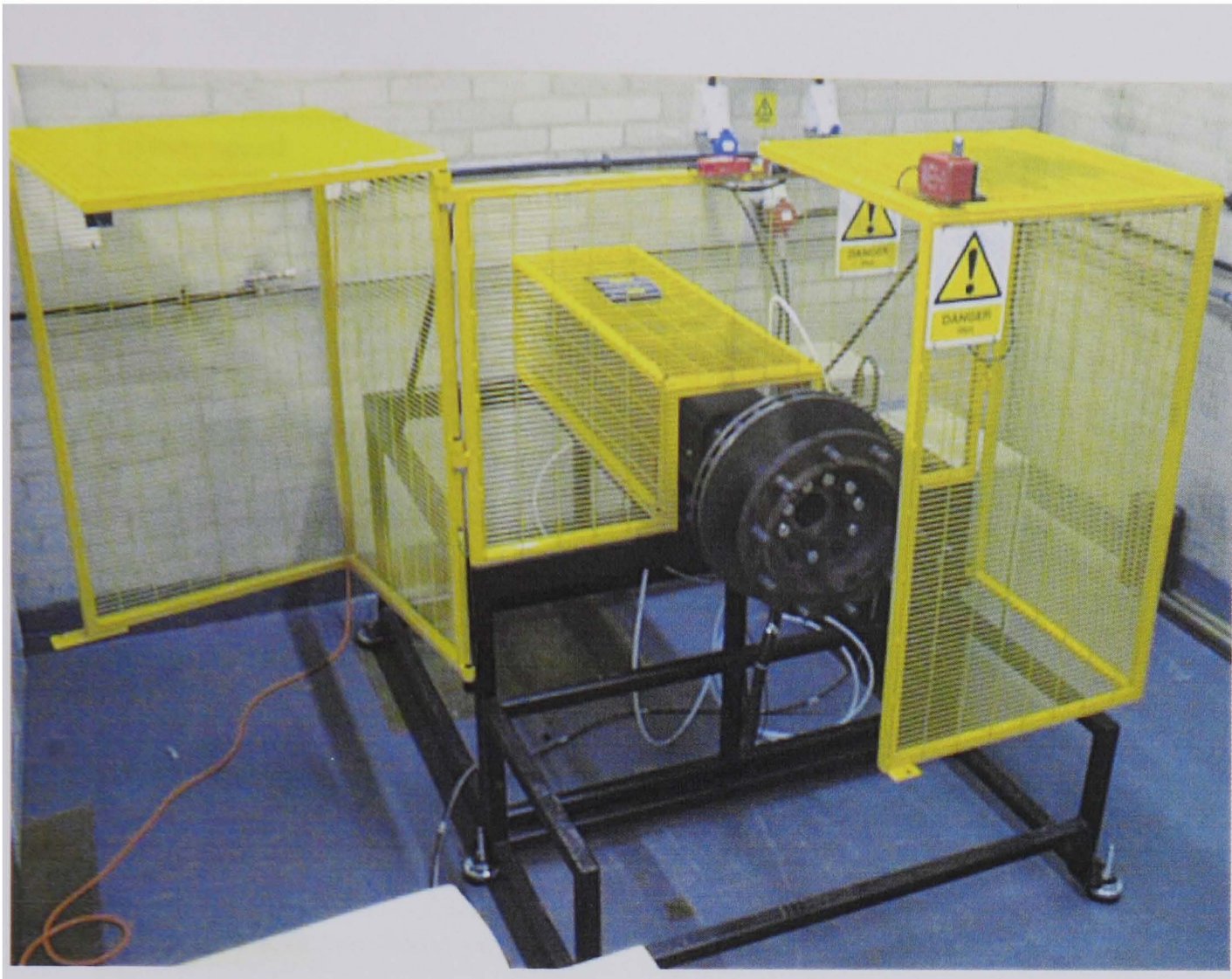
Figure 3.5 Spin Rig for studying airflow and heat dissipation from brakes
