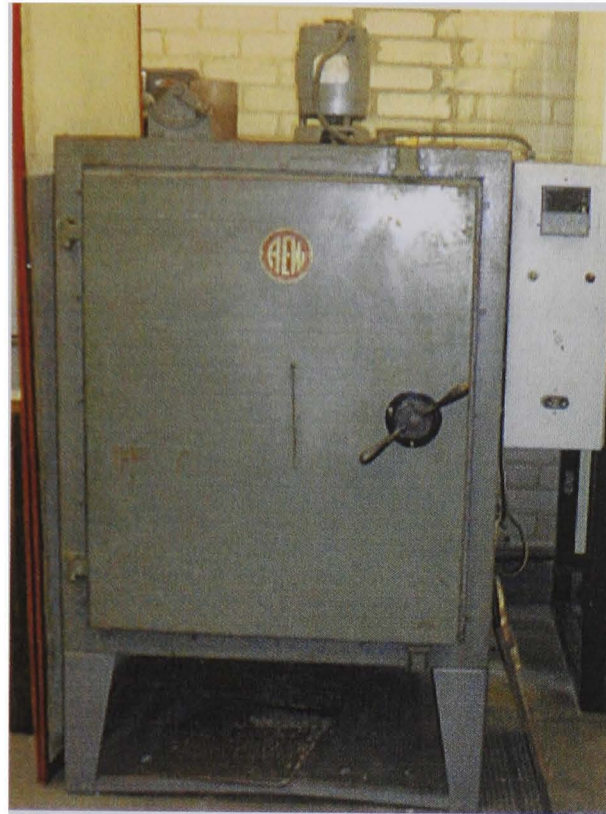
Figure 3.11 Industrial oven used to heat TGV railway disc
