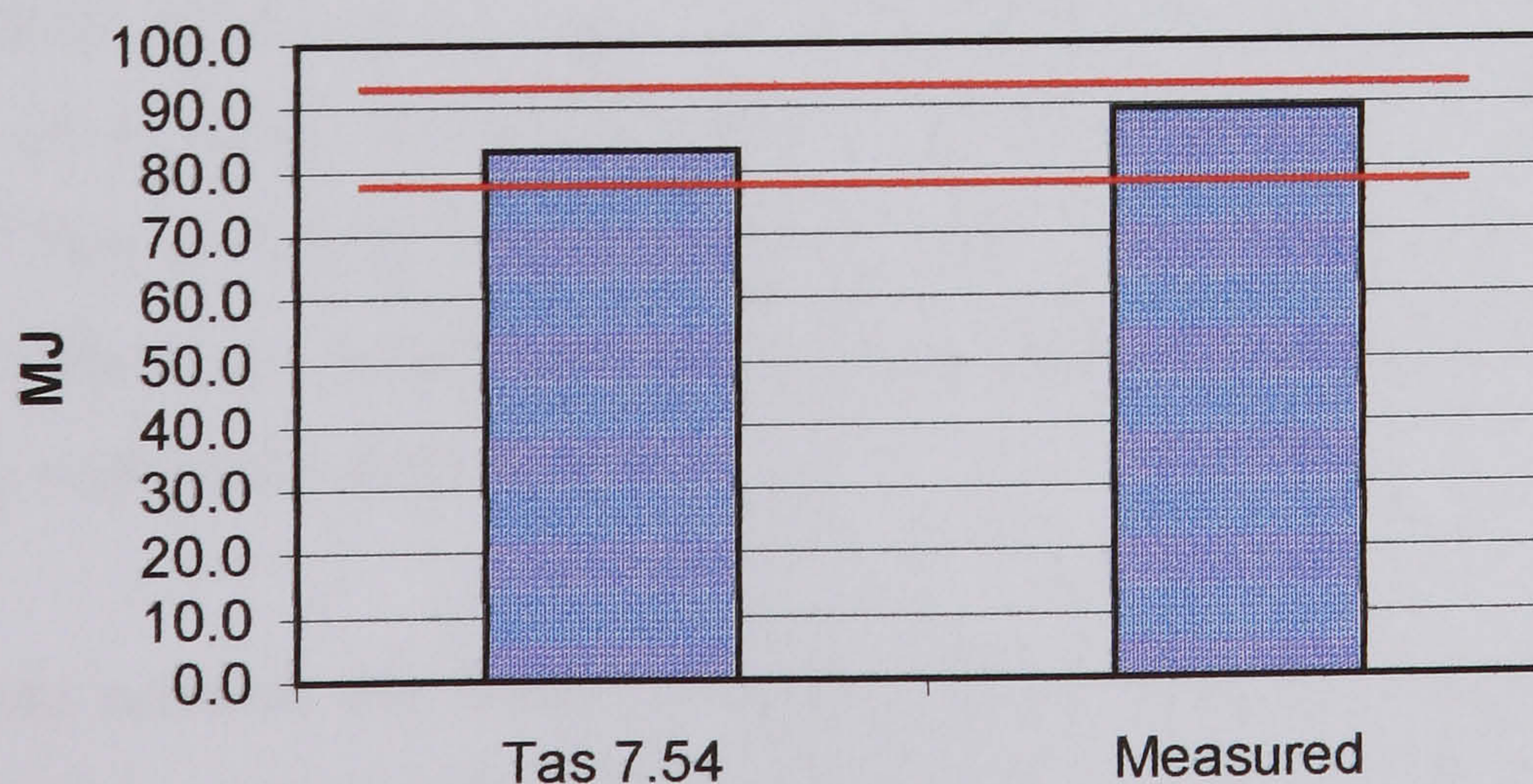
Figure 7.4: Predicted heating energy used in the double-glazed test room compared to the measured value, for Tas 7.54 (Lomas, Eppel et al. 1994)
