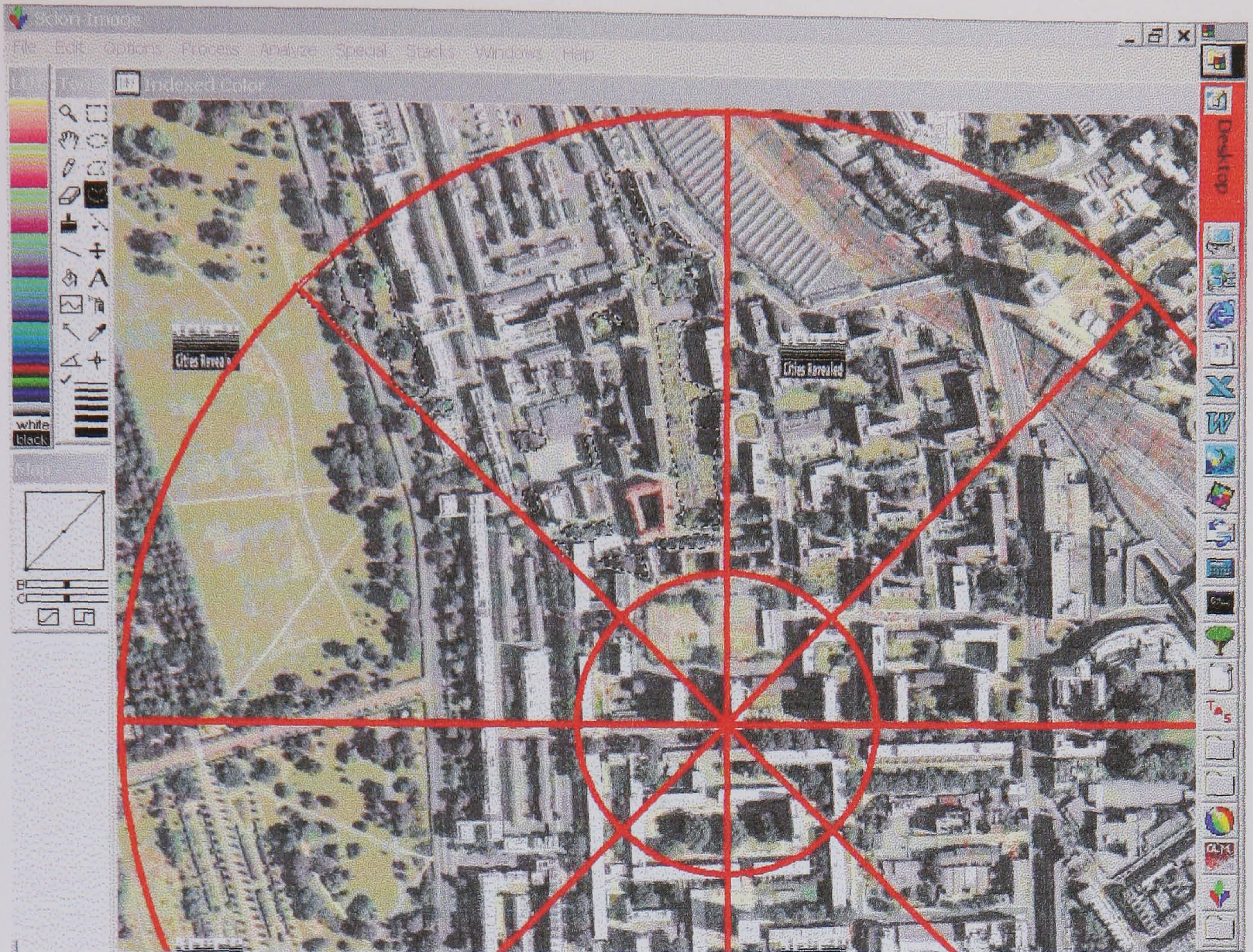
Measurement of green areas: example for the NW01 site (NW to N sector annulus)
