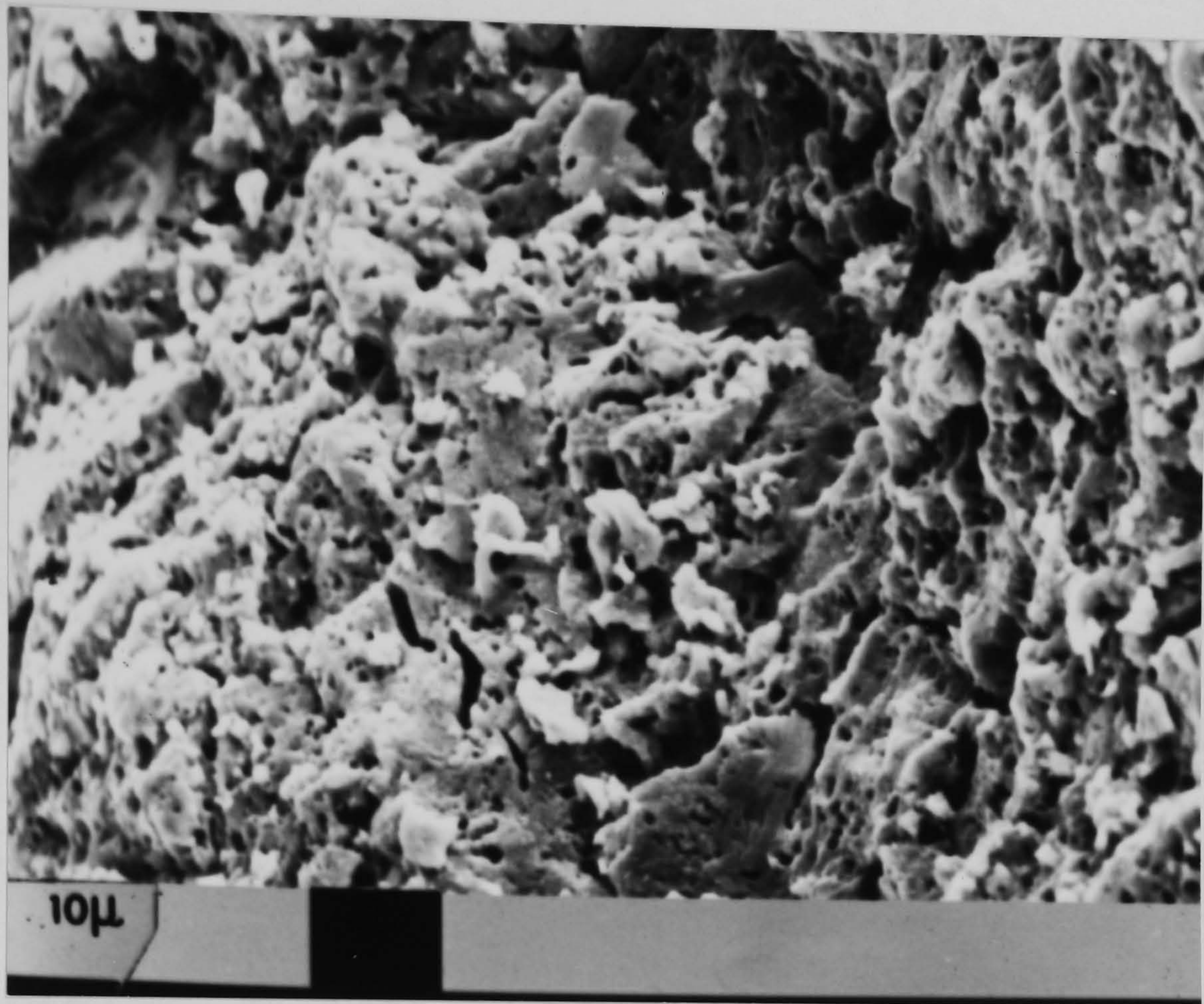
Scanning Electron Micrograph M: Sponge produced at 819^{\circ}\text{C} , Run No. 40. x 2000
