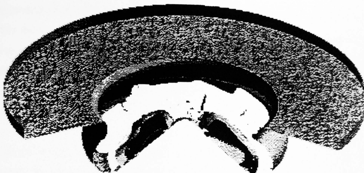
Figure 6.20 Three dimensional perspective view of a section of two-thirds of piston bowl shape TWO, illustrating iso-concentration surfaces of soot, formed at 15 degrees after TDC, of the best injector configuration case (150 degree cone angle, 5.5mm washer thickness). Engine speed 1500 rpm, full-load (see table 5.2).
