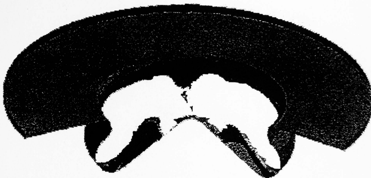
Figure 6.19 Three dimensional perspective view of a section of two-thirds of piston bowl shape TWO, illustrating iso-concentration surfaces of soot, formed at 10 degrees after TDC, of the worst injector configuration case (140 degree cone angle, 2.5mm washer thickness). Engine speed 1500 rpm, full-load (see table 5.2).
