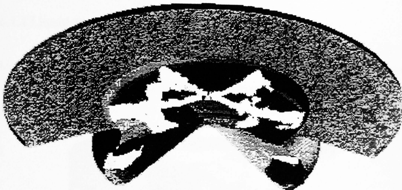
Figure 6.15 Three dimensional perspective view of a section of two-thirds of piston bowl shape TWO, showing the liquid fuel envelope and the initial sites of ignition, as dark regions of the fuel spray. Start of combustion occurred at 6 degrees after TDC, for the best injector configuration case (140 degree cone angle, 2.5mm washer thickness). Engine speed 1500 rpm, full-load (see table 5.2).
