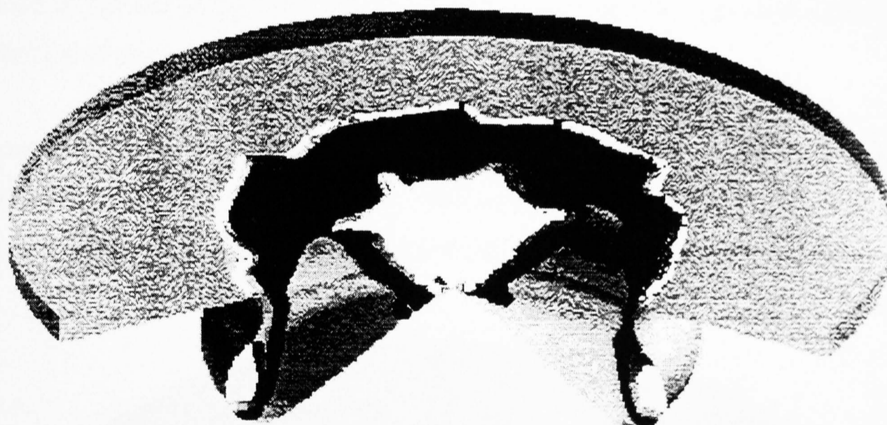
Figure 6.21 Three dimensional perspective view of a section of two-thirds of piston bowl shape TWO, illustrating iso-concentration surfaces of soot, formed at 15 degrees after TDC, of the worst injector configuration case (140 degree cone angle, 2.5mm washer thickness). Engine speed 1500 rpm, full-load (see table 5.2).
