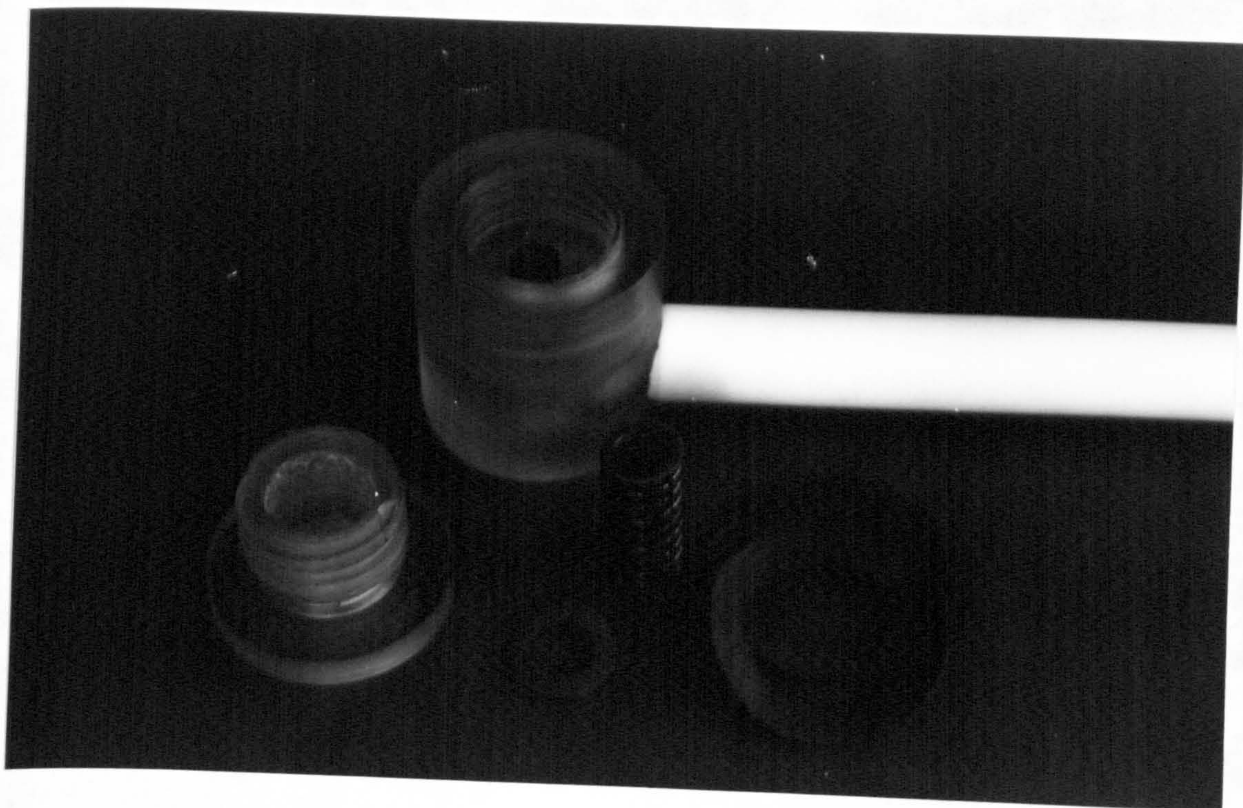
Fig. 14. Dismantled Disc Electrode Holder Showing Component Parts.
