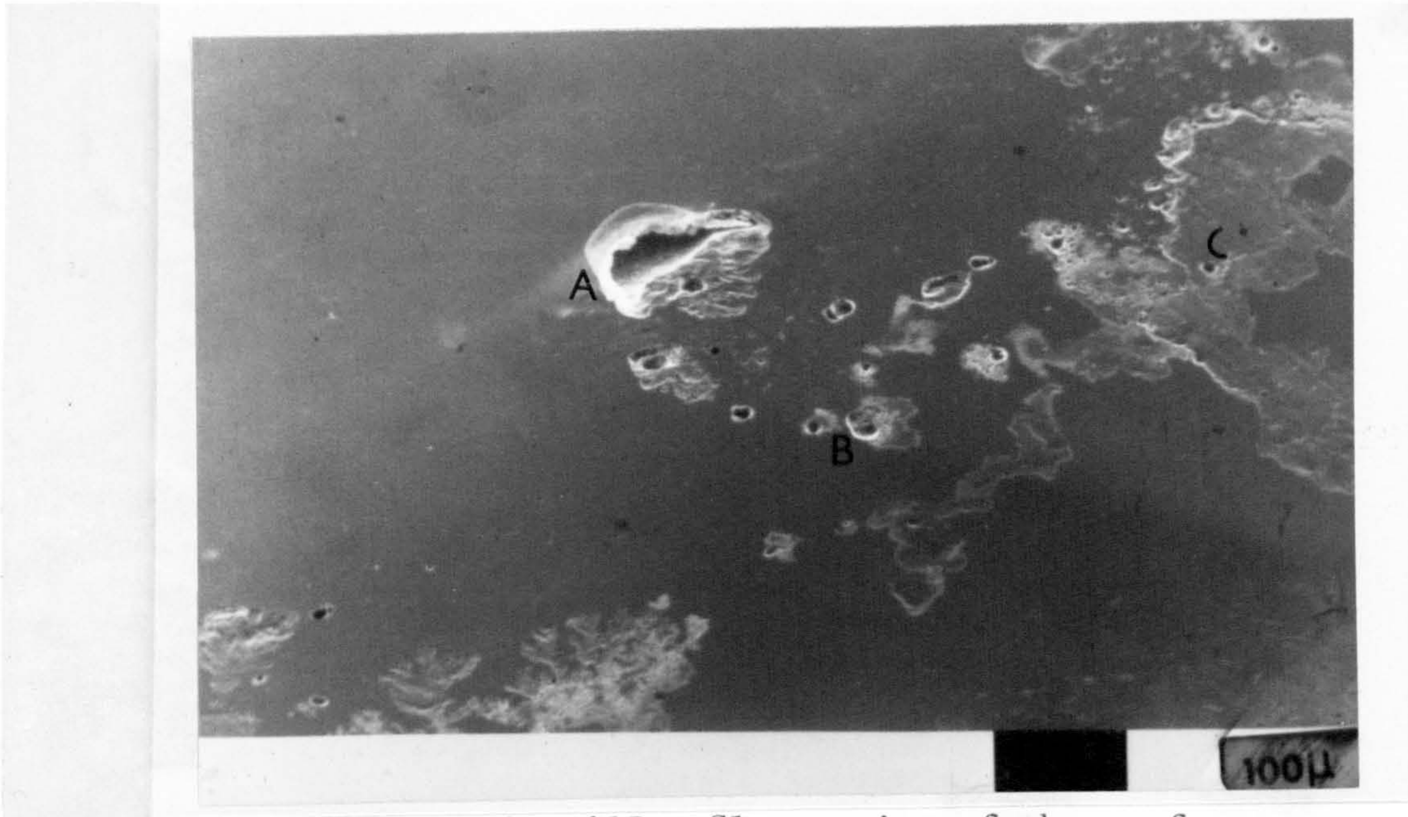
Fig. 106. As Fig. 105. Closer view of the surface area covered by the gasket. Feature A typical cervix morphology. Feature B, pits well developed. Feature C, general dissolution areas. x200.
