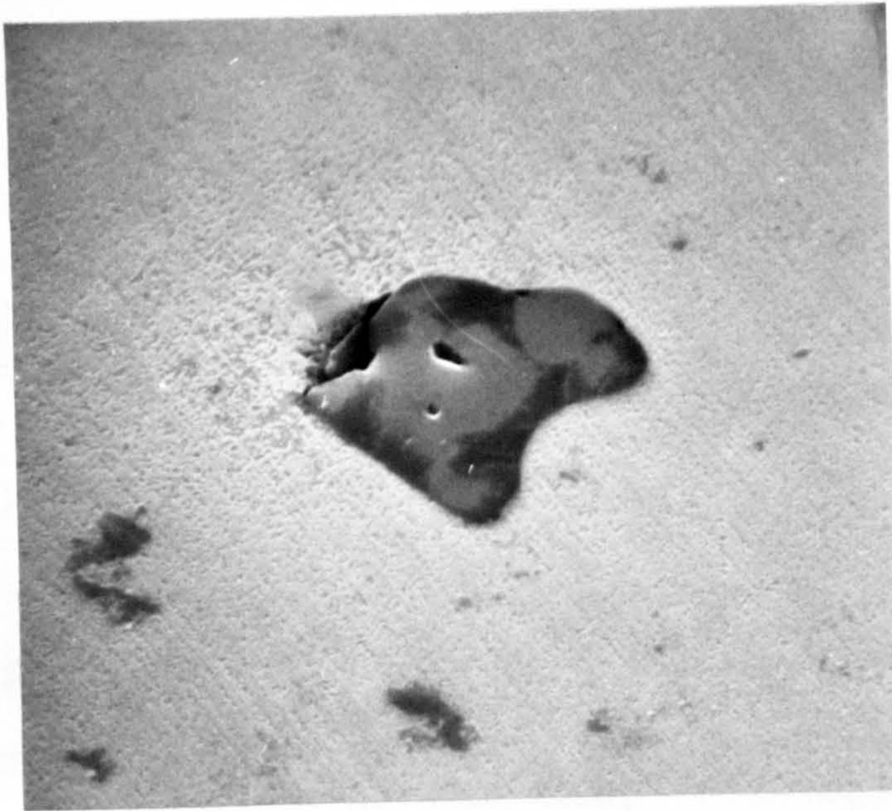
Fig. 92. As Fig. 91 showing a inclusion. 5K undergoing dissolution.
