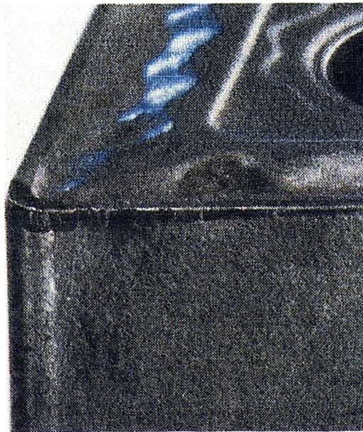
Figure 2.1. Flank wear of carbide tool [(Model Metal Cutting - A Practical Handbook, (1994)].
