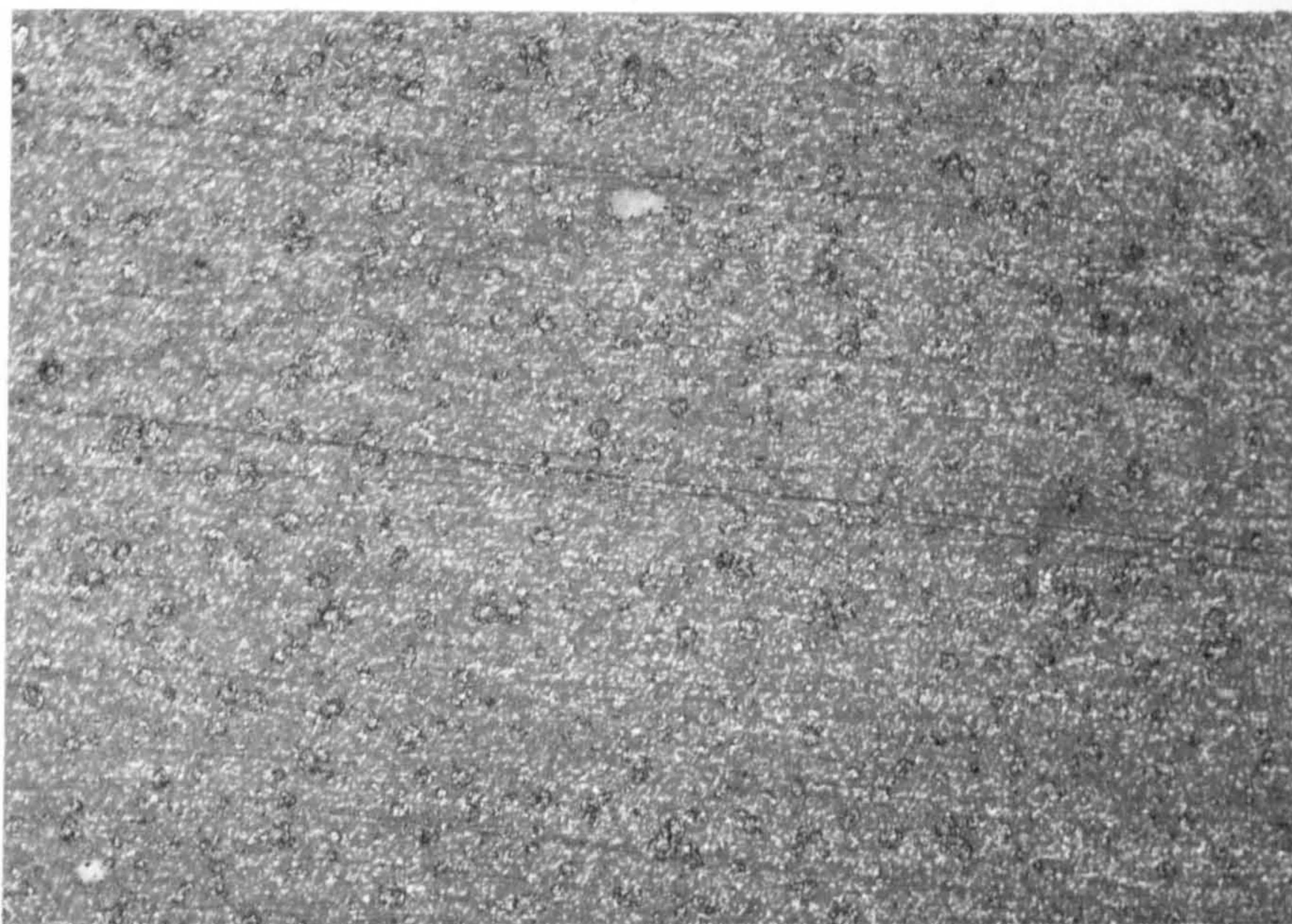
Fig.3.2.18 Optical microscopic photograph of Mo-black dip coating of Fig.3.2.14 in dry condition. No crack in the surface. Magnification: 100X.
