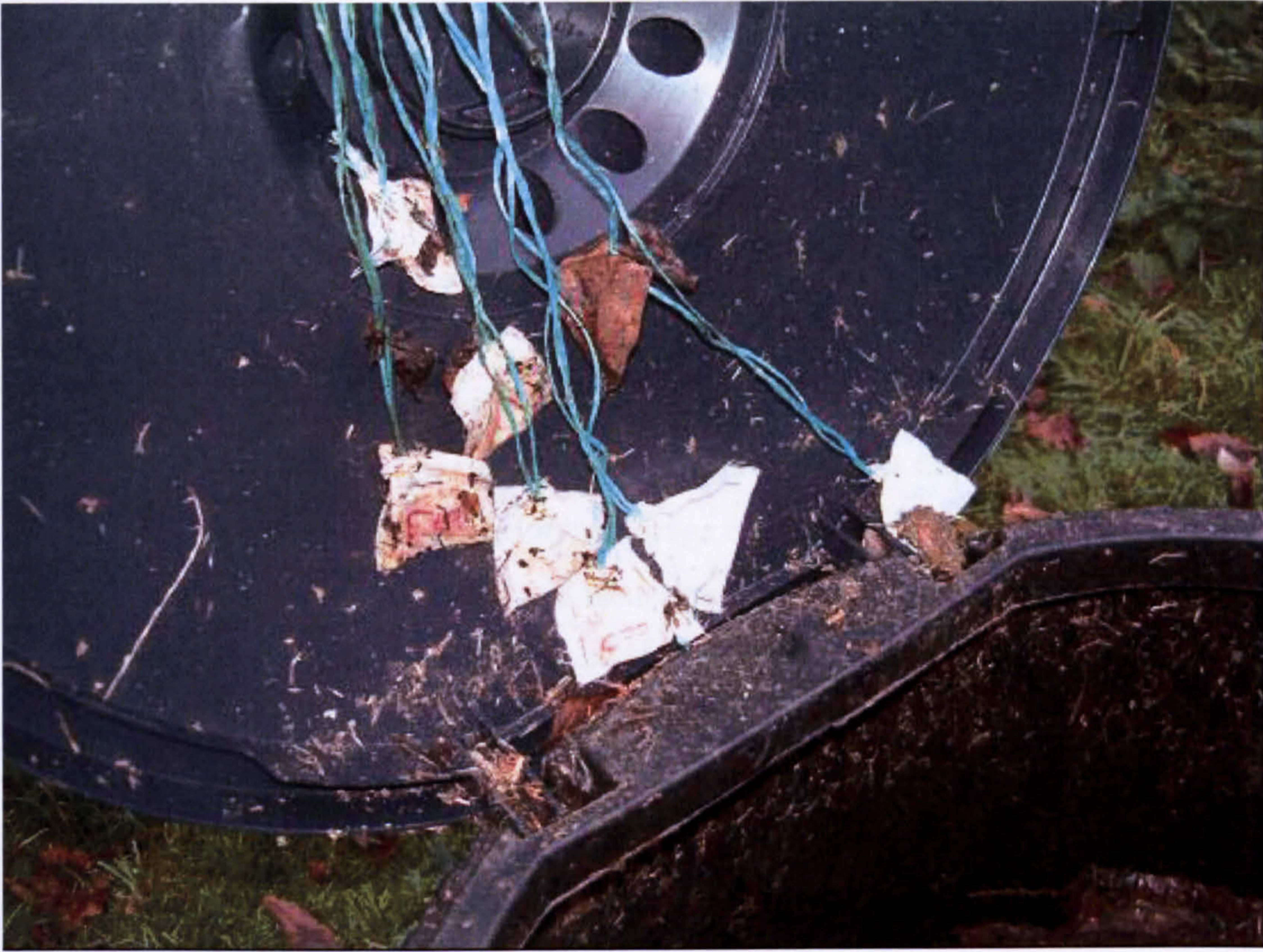
Figure 8.8: 'Take out' specimens added to the composting bins containing the stainless steel racks.
