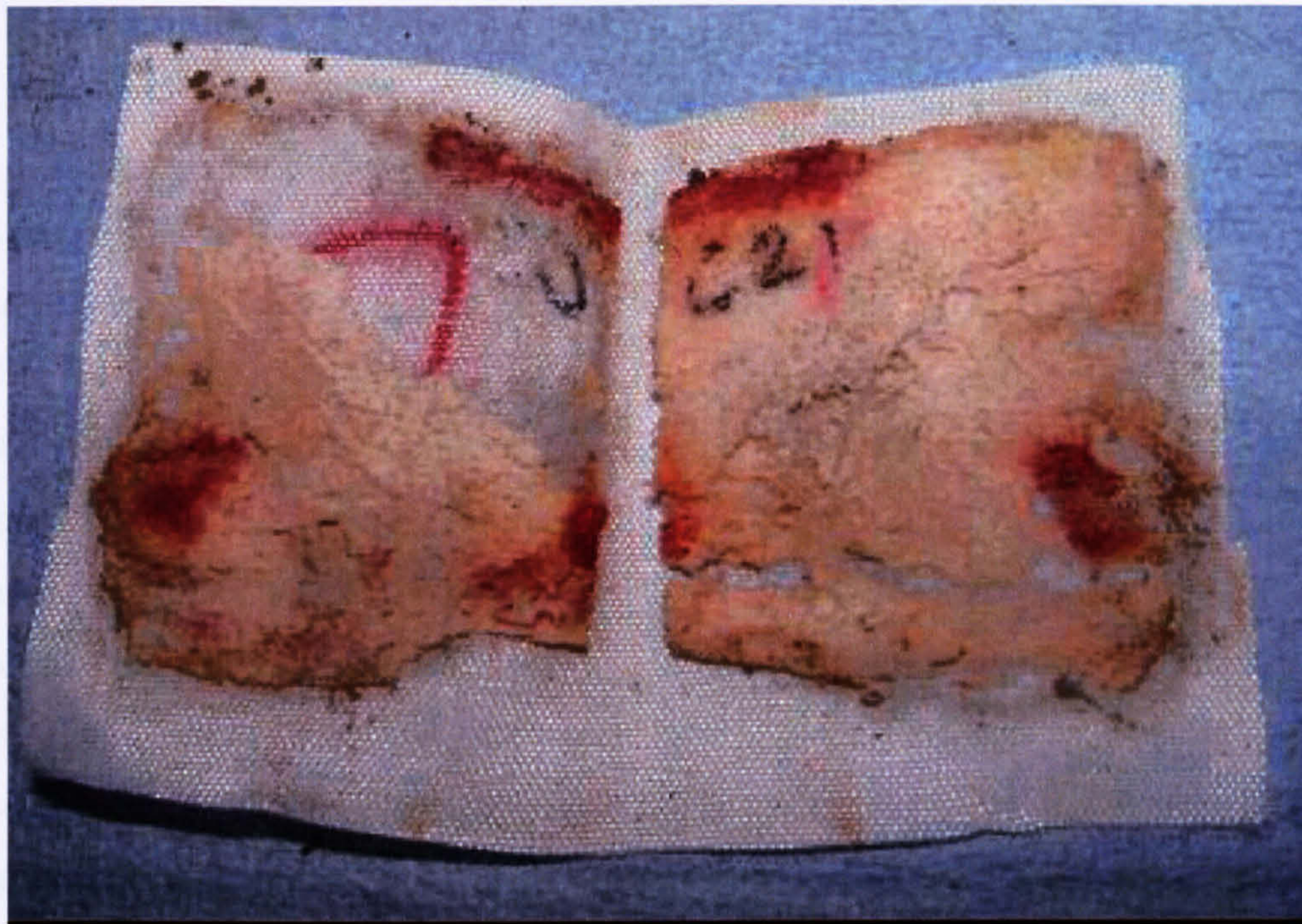
Figure 8.9: showing a detailed close up of a degraded potato starch sample
