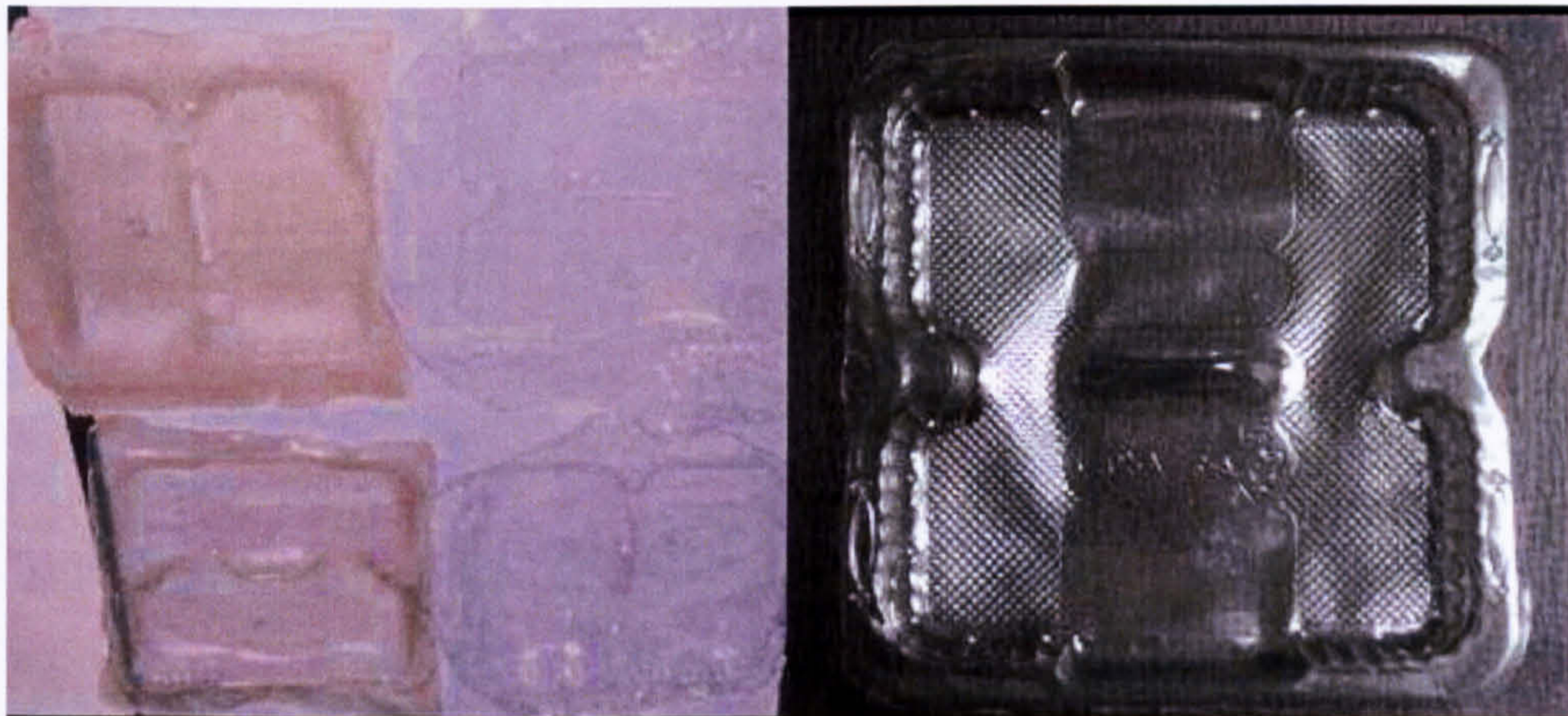
Figure 6.16: “A” and “B” samples successfully vacuum formed, with a close up of sample “A” material.
