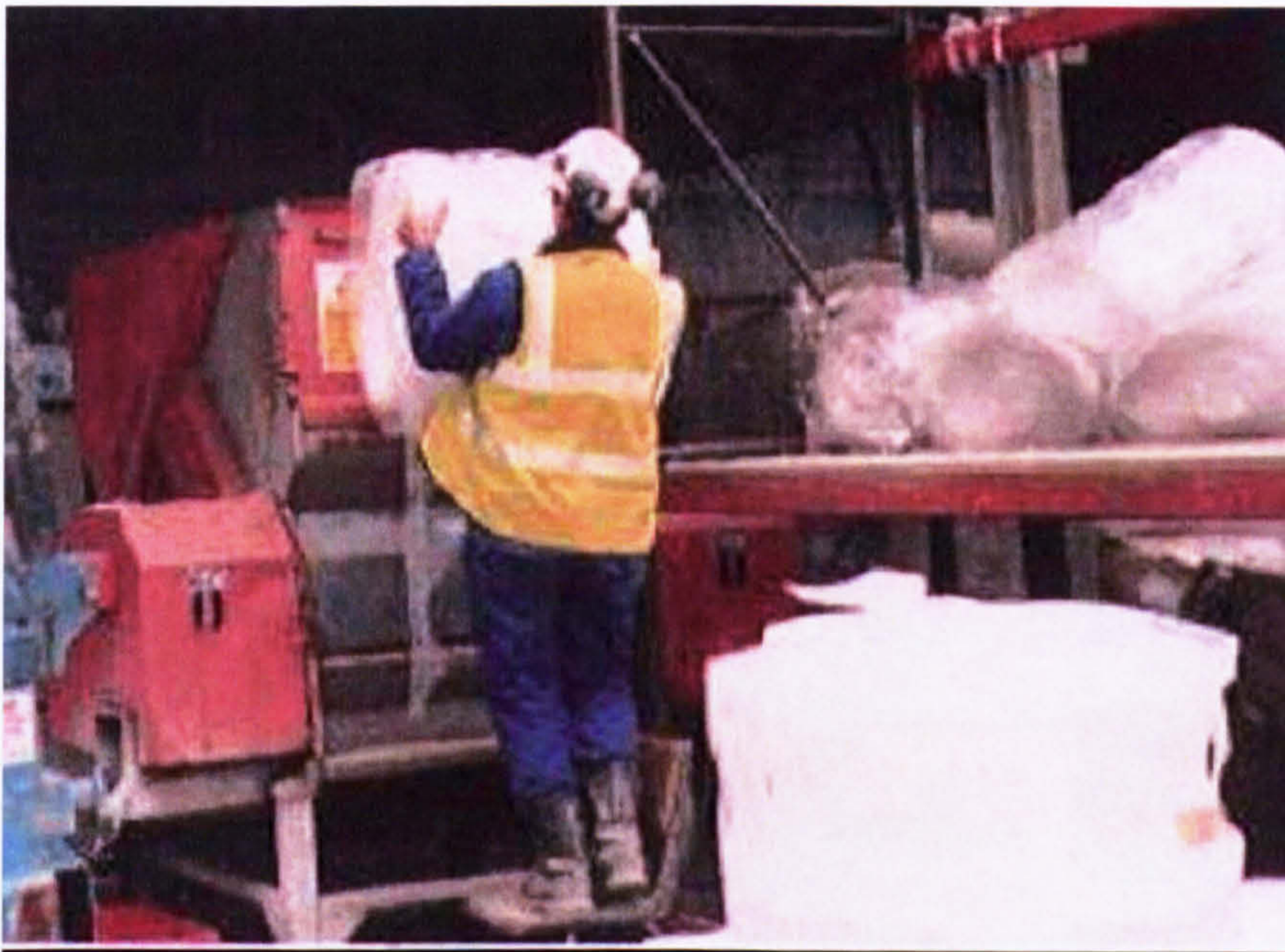
Figure 4.29: Skeletal waste plastic material being manually placed into the hopper
