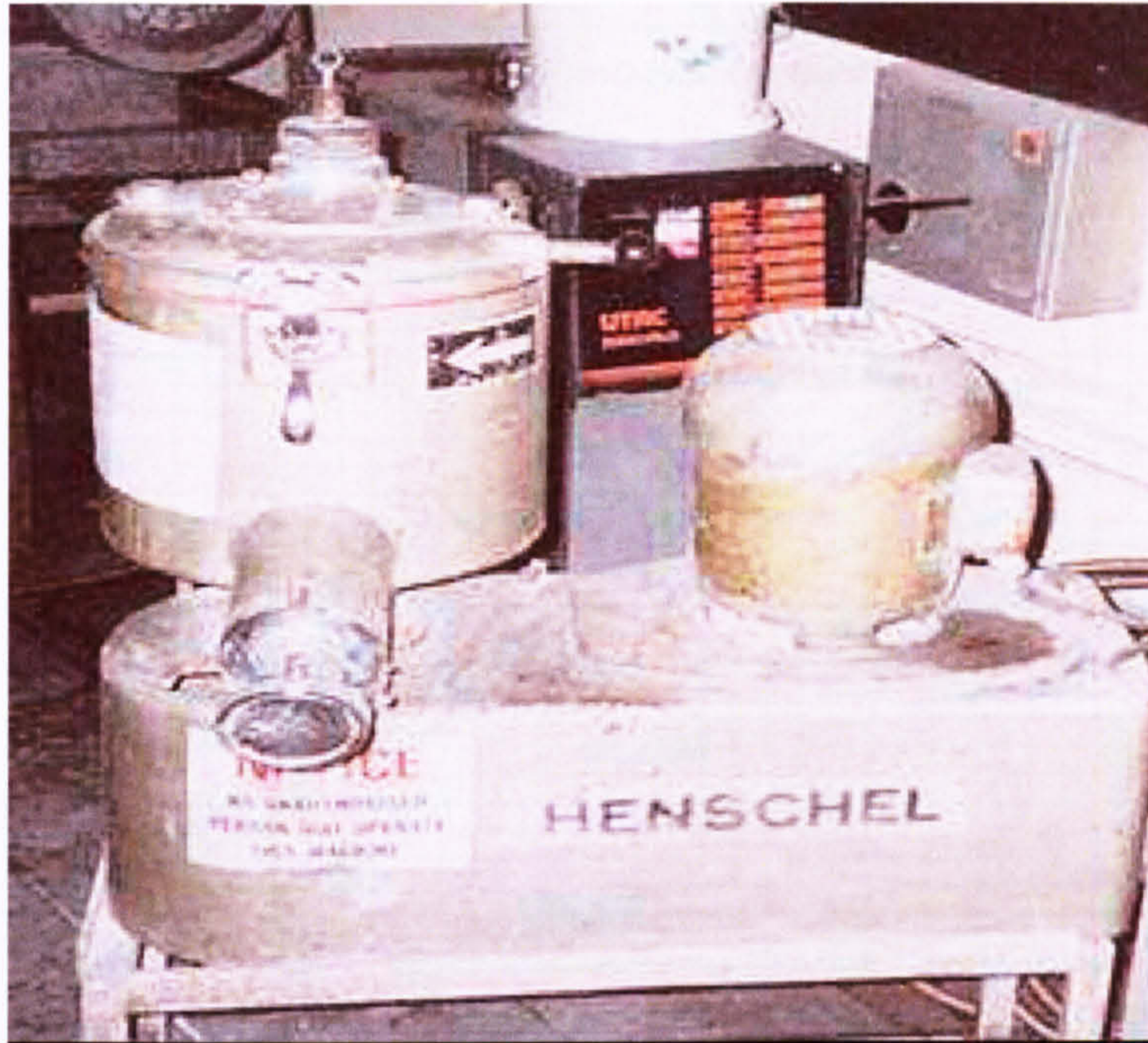
Figure 6.1: Henschel high-speed mixer used to blend purified wheat starch, wheat flour, glycerol and PVA combinations
