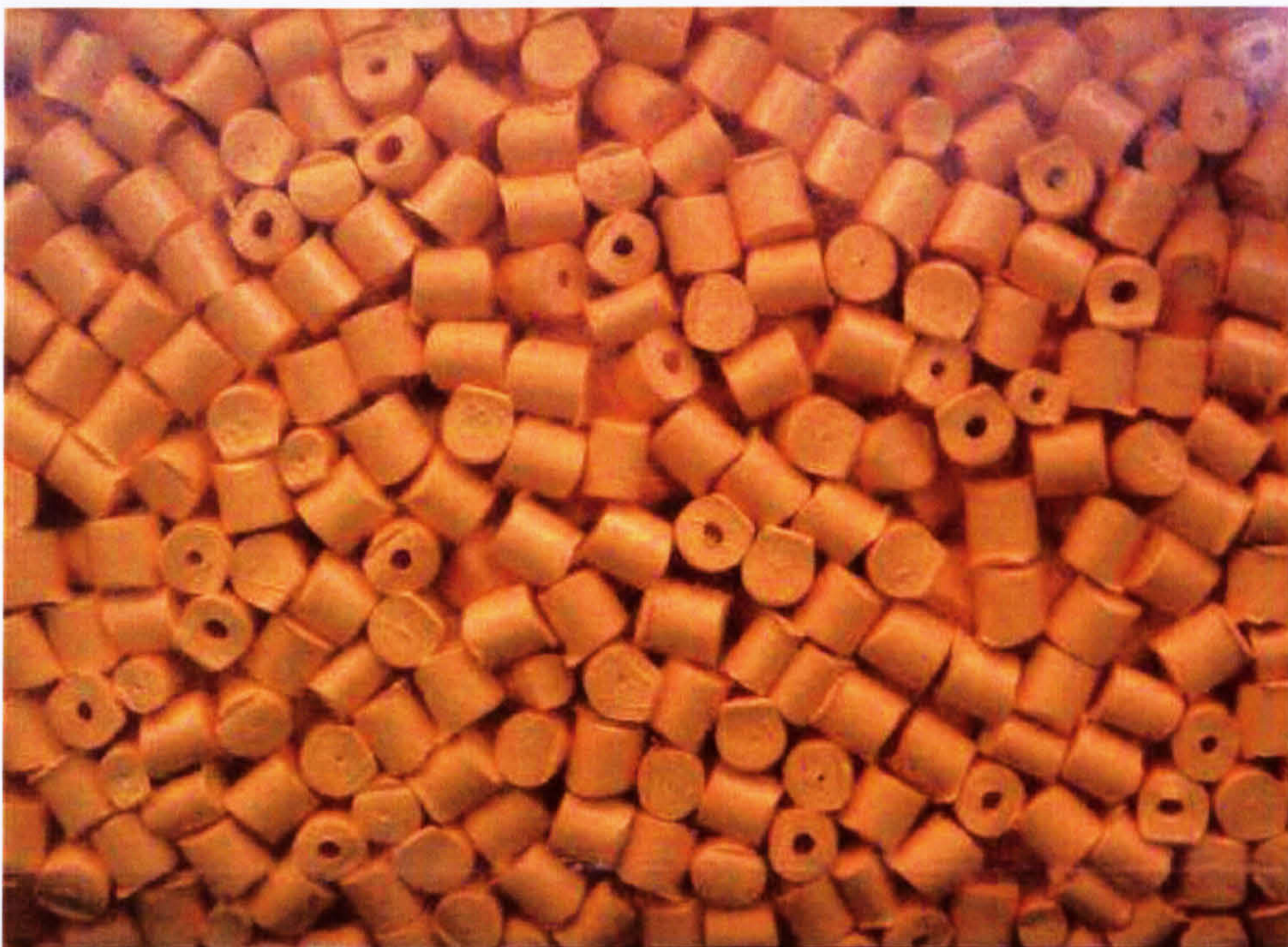
Figure 4.12: Thermoplastic in a pellet format
