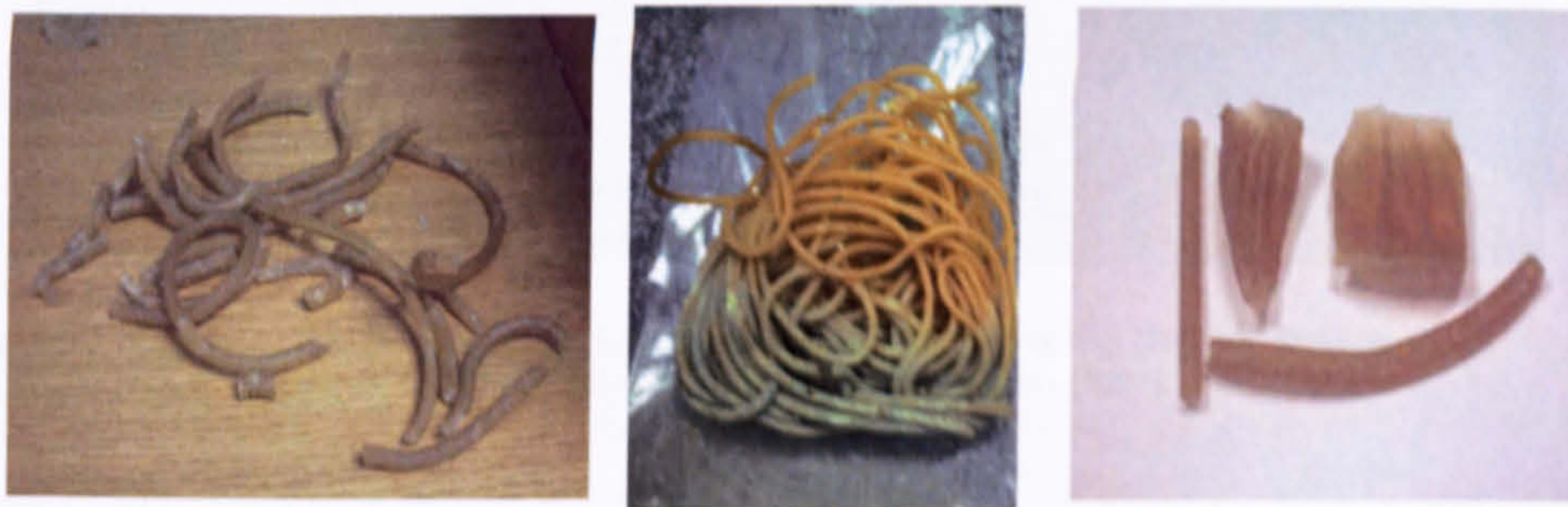
Figure 9 Initial trialing proving that 100% starch could be extruded
