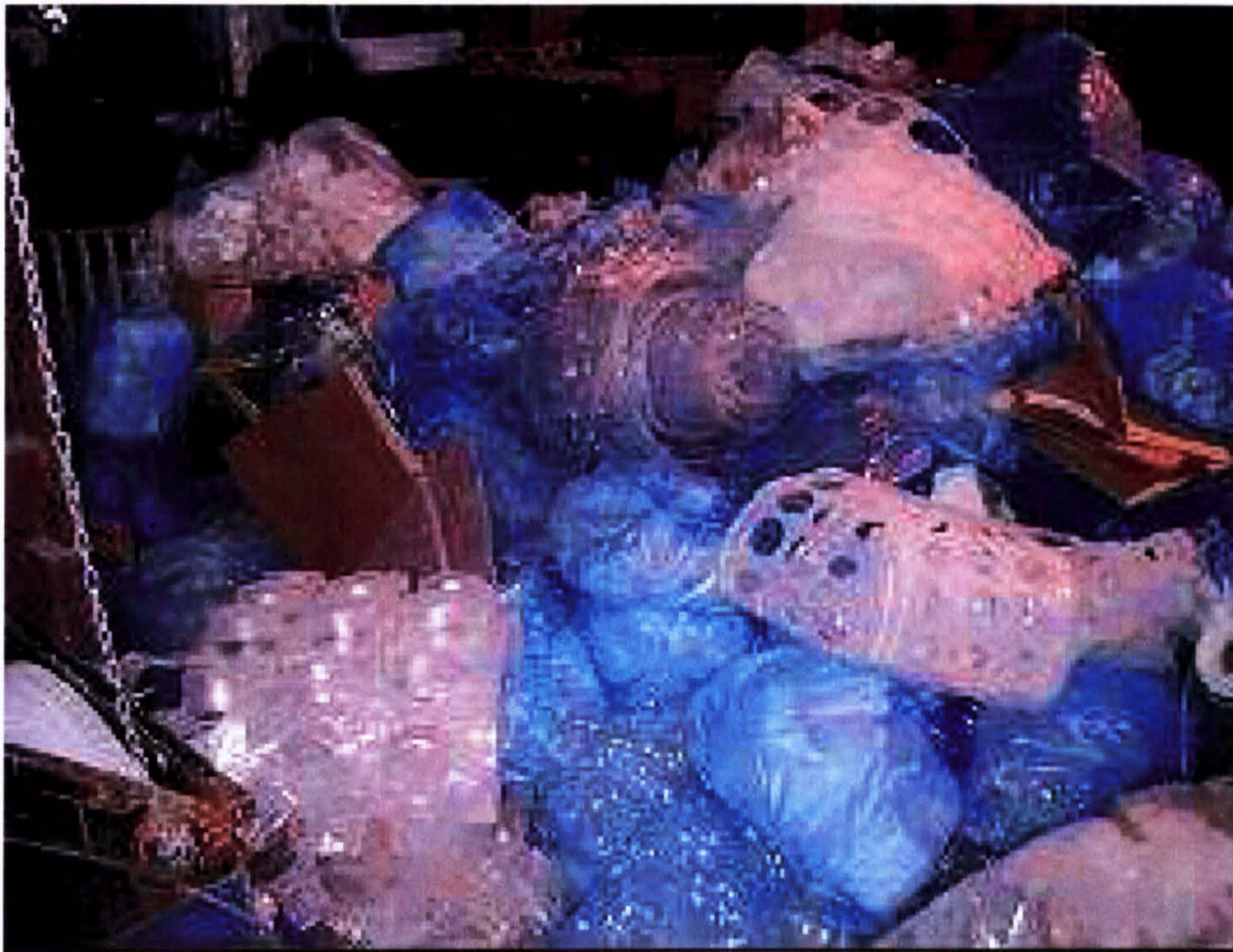
Figure 4.25: A close up of the general waste showing skeletal waste and reject forming
