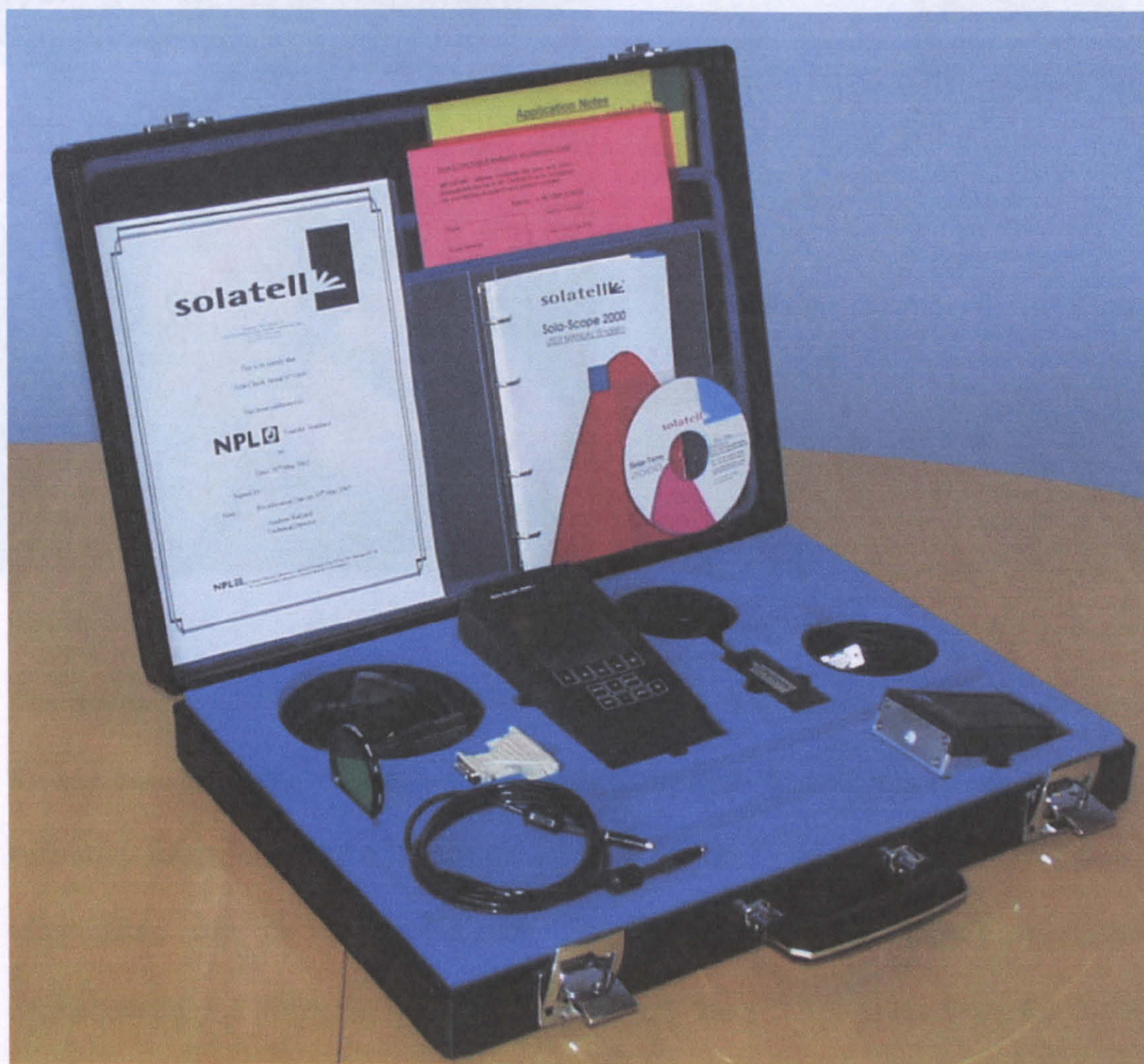
Figure 2.3: Sola Scope 2000 as supplied by 4D controls Ltd. (Picture courtesy of 4D controls).
