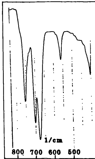
Fig 4.4.11 IR spectrum of 20% iso-propyl ZDDP in DMA
