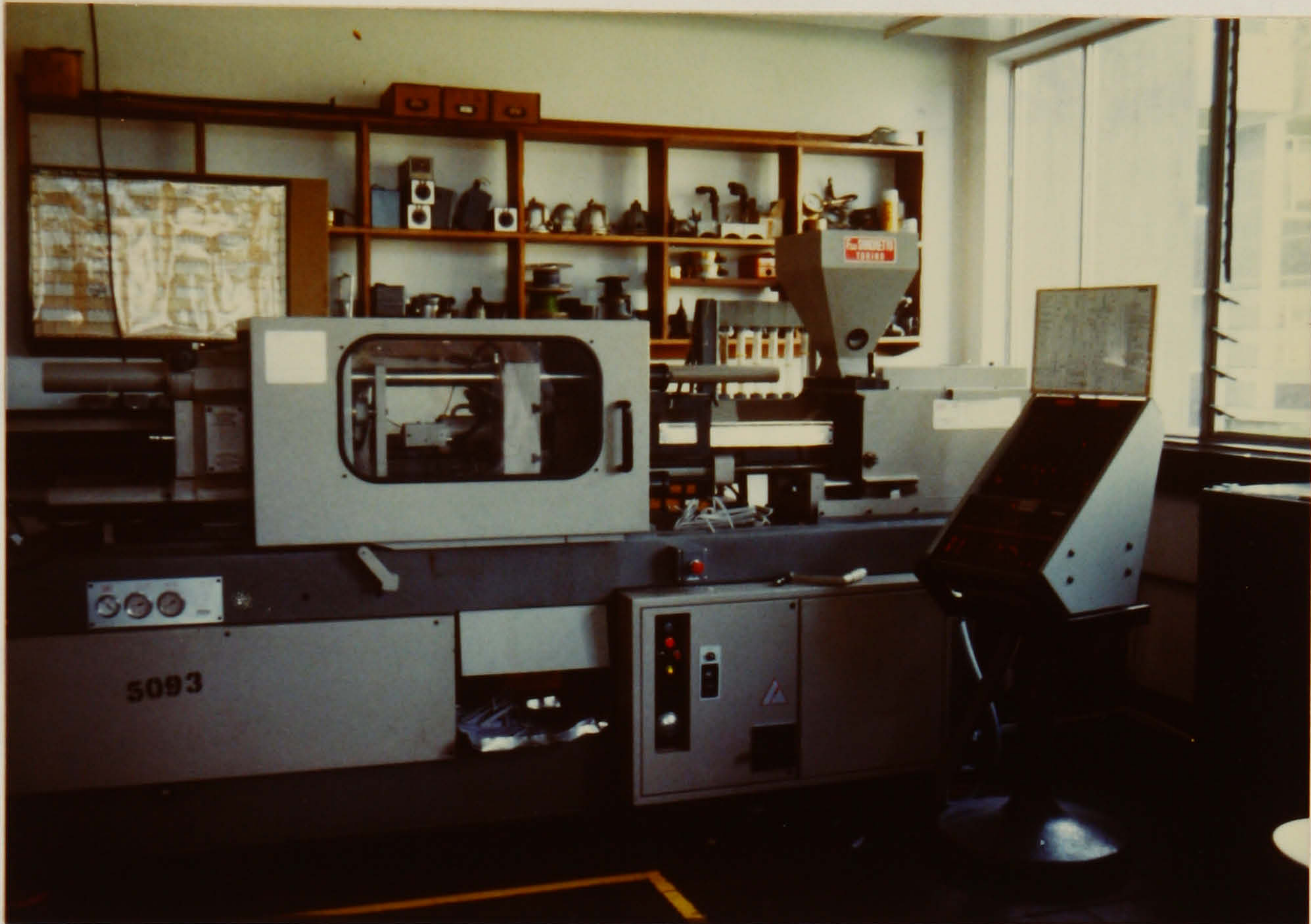
Fig (5) Injection-moulding machine used (Sandretto Co.) in preparation of tensile and flexural test specimens
