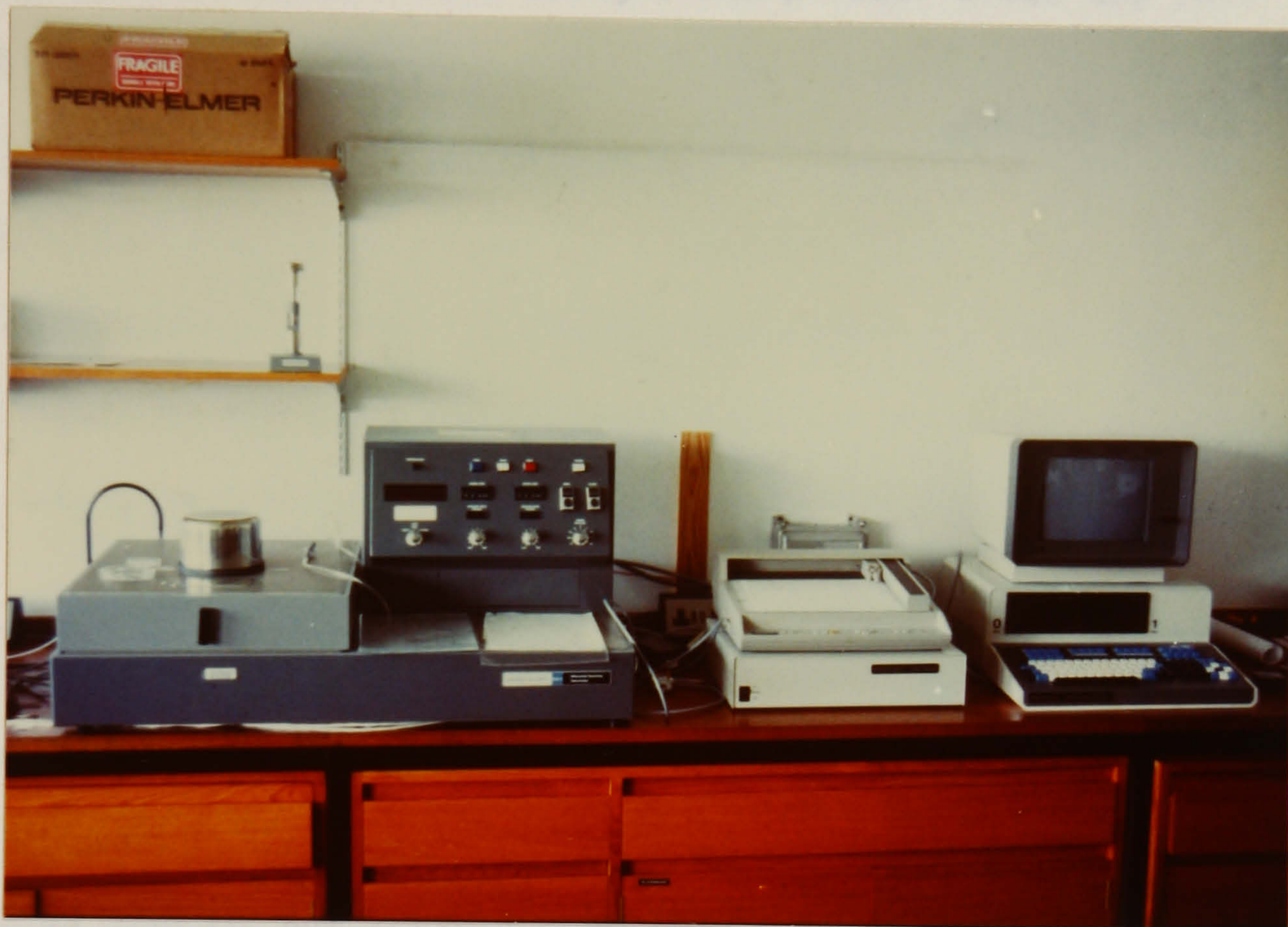
Fig (10) Differential scanning calorimeter used (Perkin-Elmer Model D.S.C.2)
