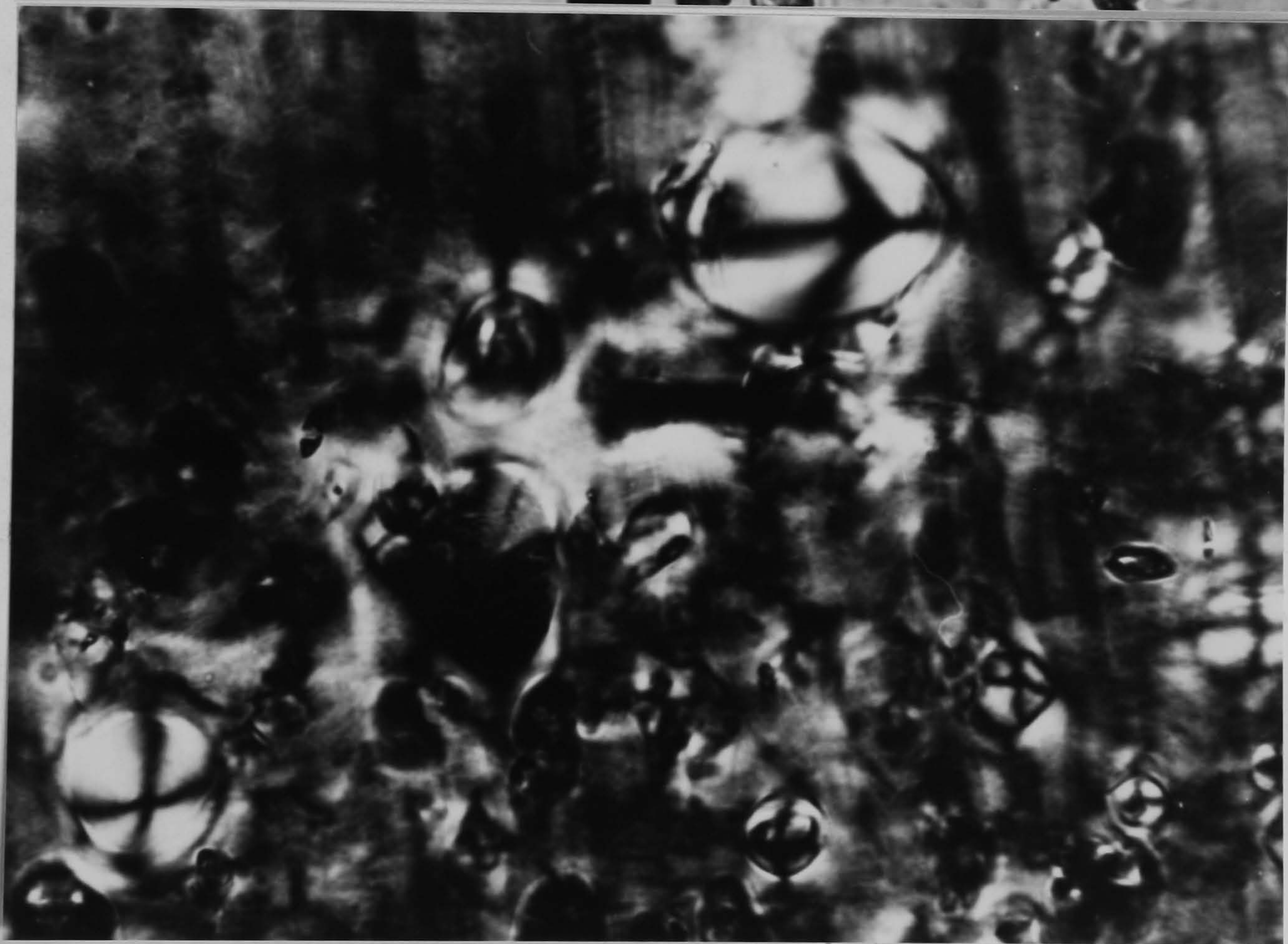
Plates (11 & 12) Optical photomicrograph of microtome cross-section of 1% potato starch filled HDPE (x 420) (Top): normal light (bottom): polarized light, mountant Canada Balsam
