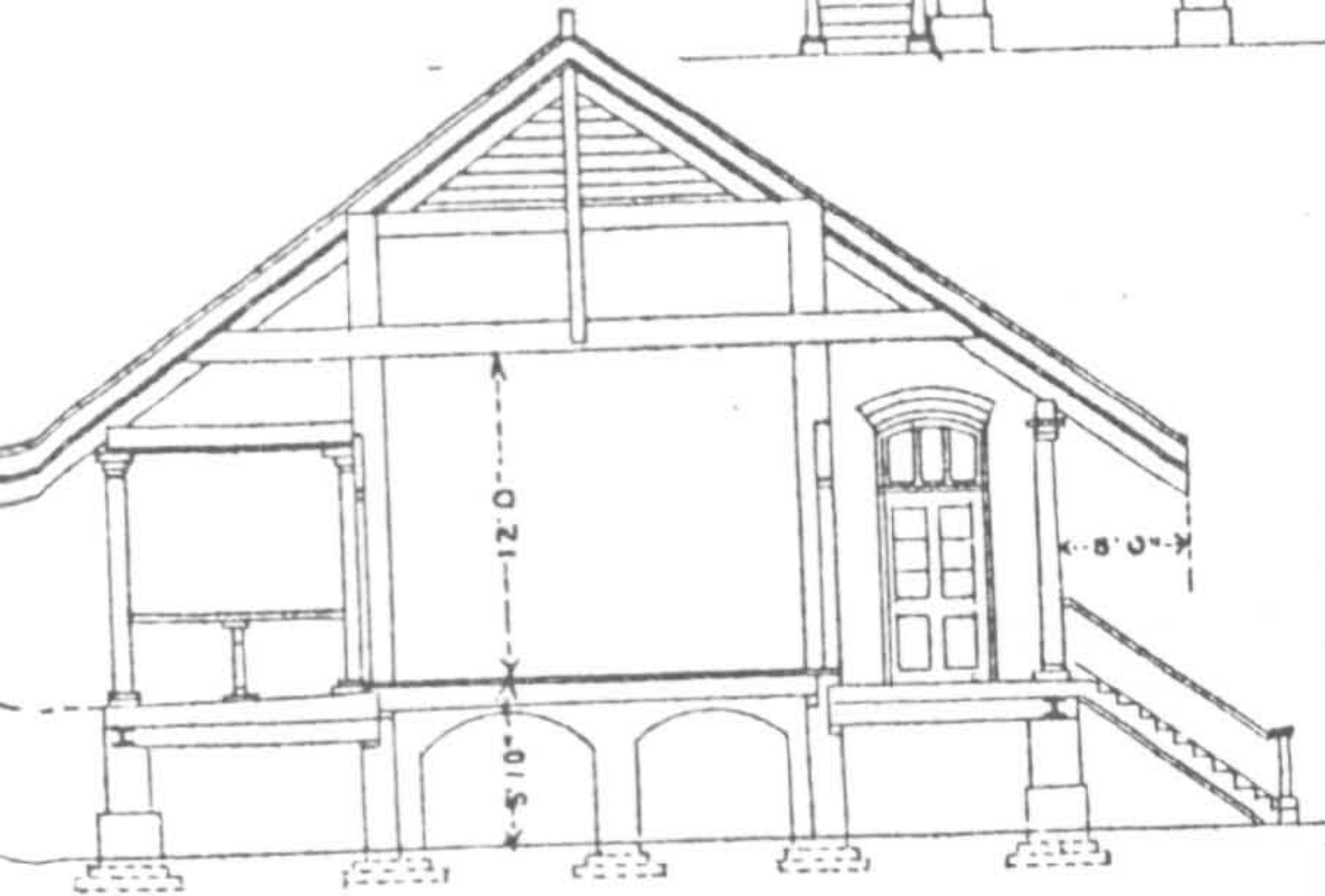
SECTION ON LINE A.B
