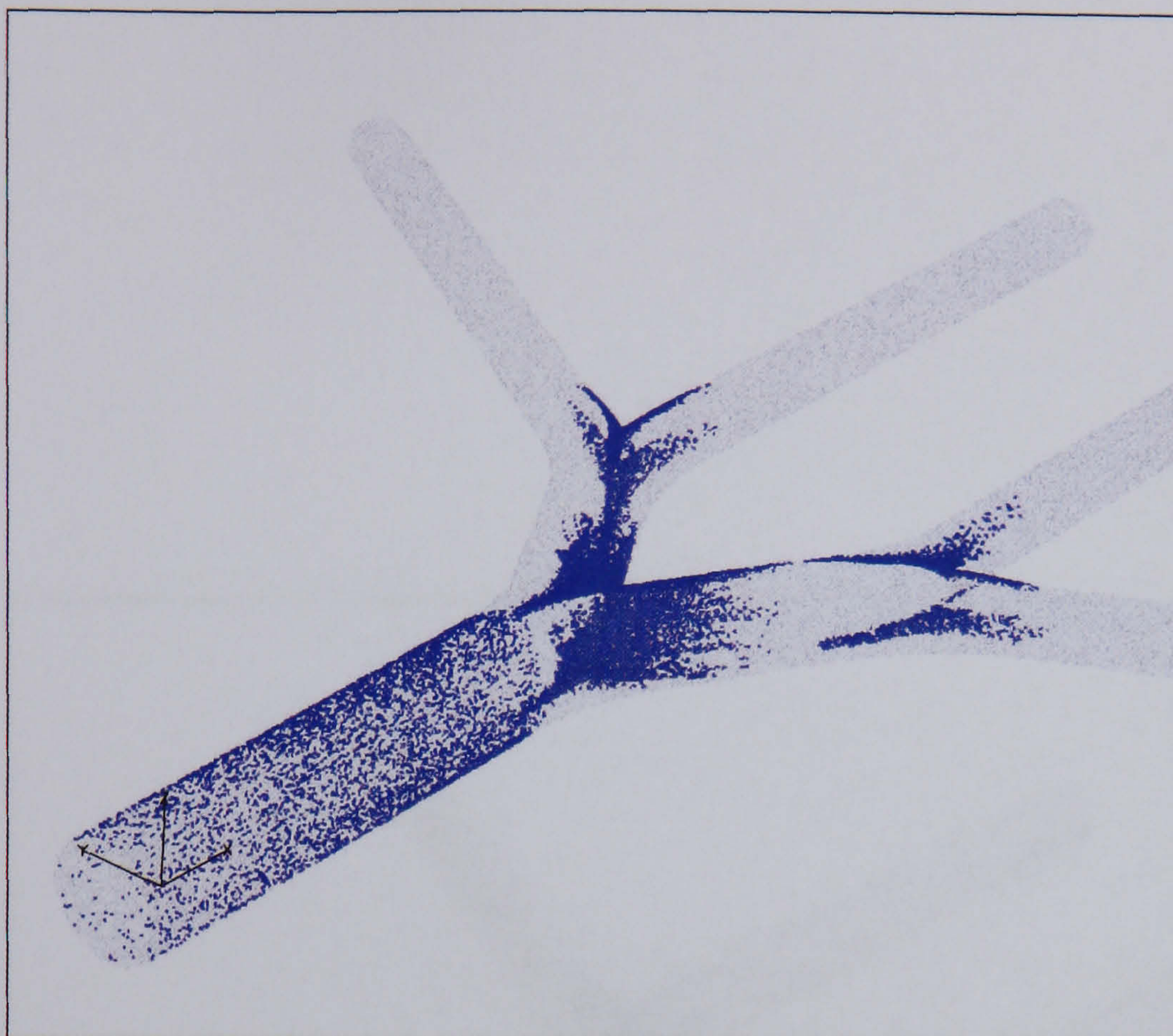
Figure 6.12: Local deposition pattern of 0.5 \mu m particles carrying q = 250e in the 3D bifurcation airway model with a uniform inlet distribution under a light activity breathing condition
