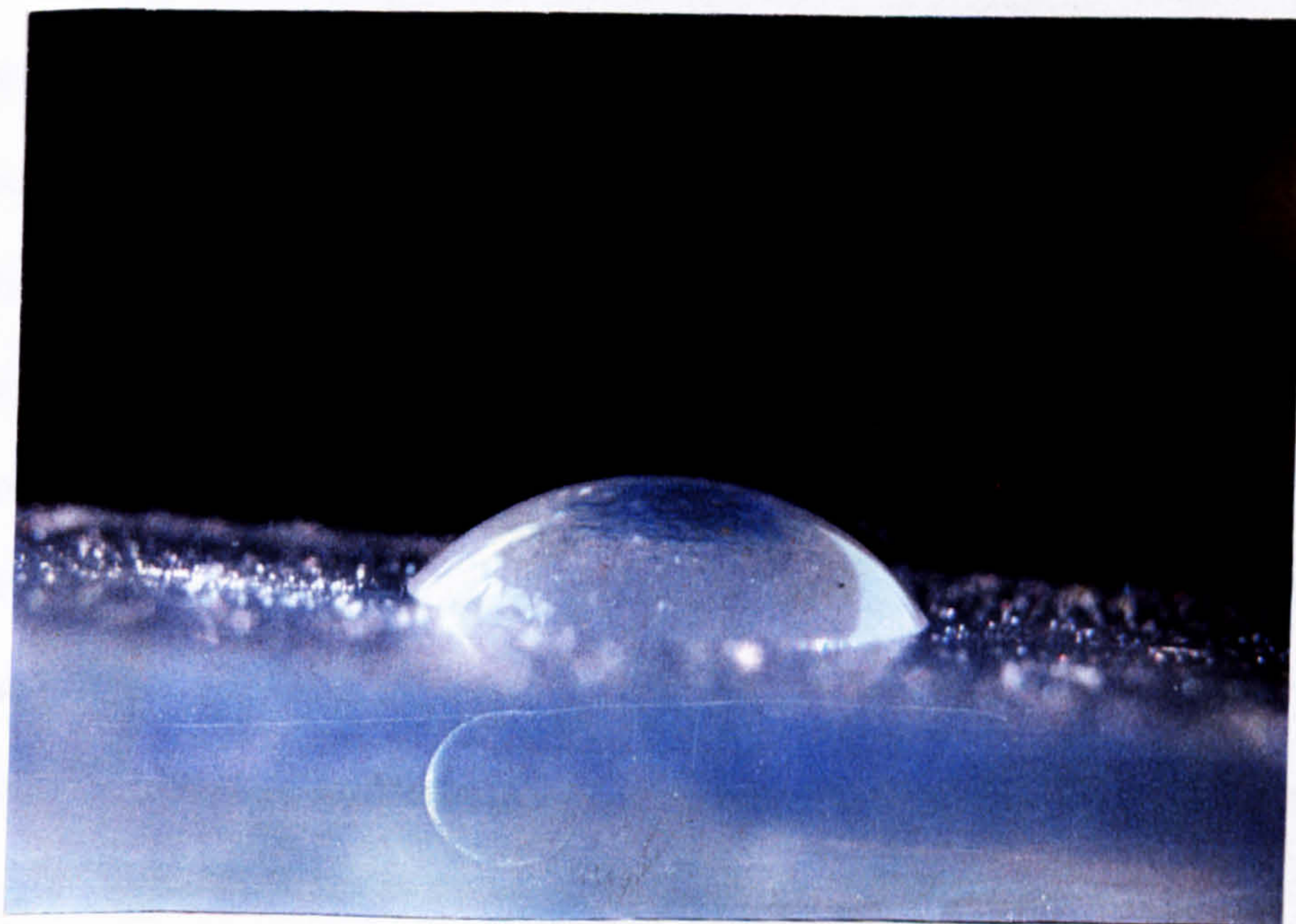
Figure 4.27 Water drop contact angle of the AAm grafted onto the PDMS surface which was pre-treated by laser beam at 9.58\ \mu\text{m} ( 1043\ \text{cm}^{-1} ) and 20 % wt concentration solution of AAm.
