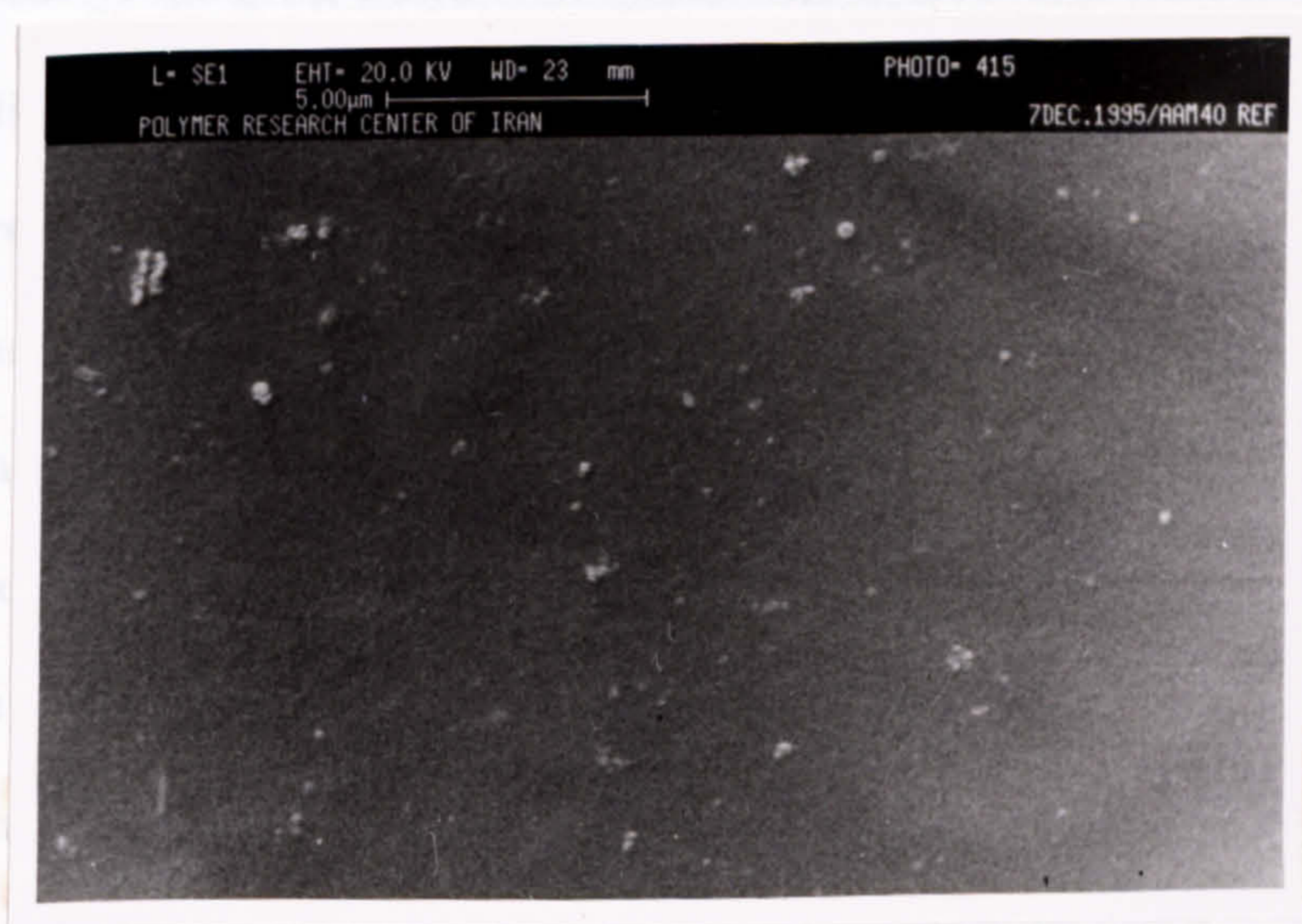
Figure 4.21 SEM micrograph (magnification is 5000 x) of untreated PDMS on which the grafting process was carried out.
