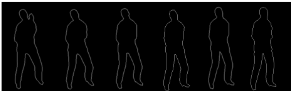
Figure 4.15. The results of the contour synthesis for human body model with clothing information. The rightmost and the leftmost images are in-out images. The others are pixel synthesis results using the proposed method.
