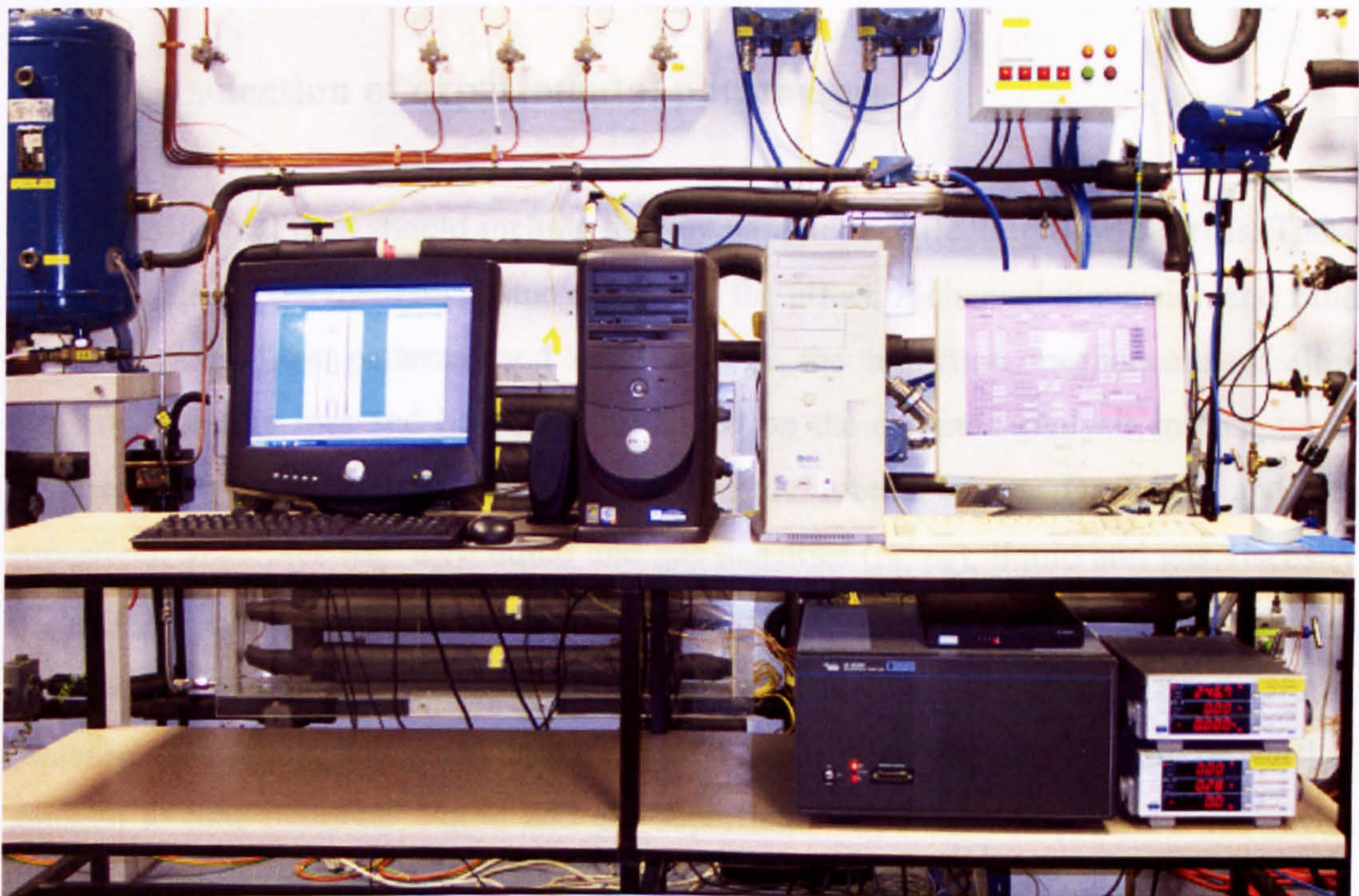
Figure 3.6 Photograph of the control and data acquisition system.
