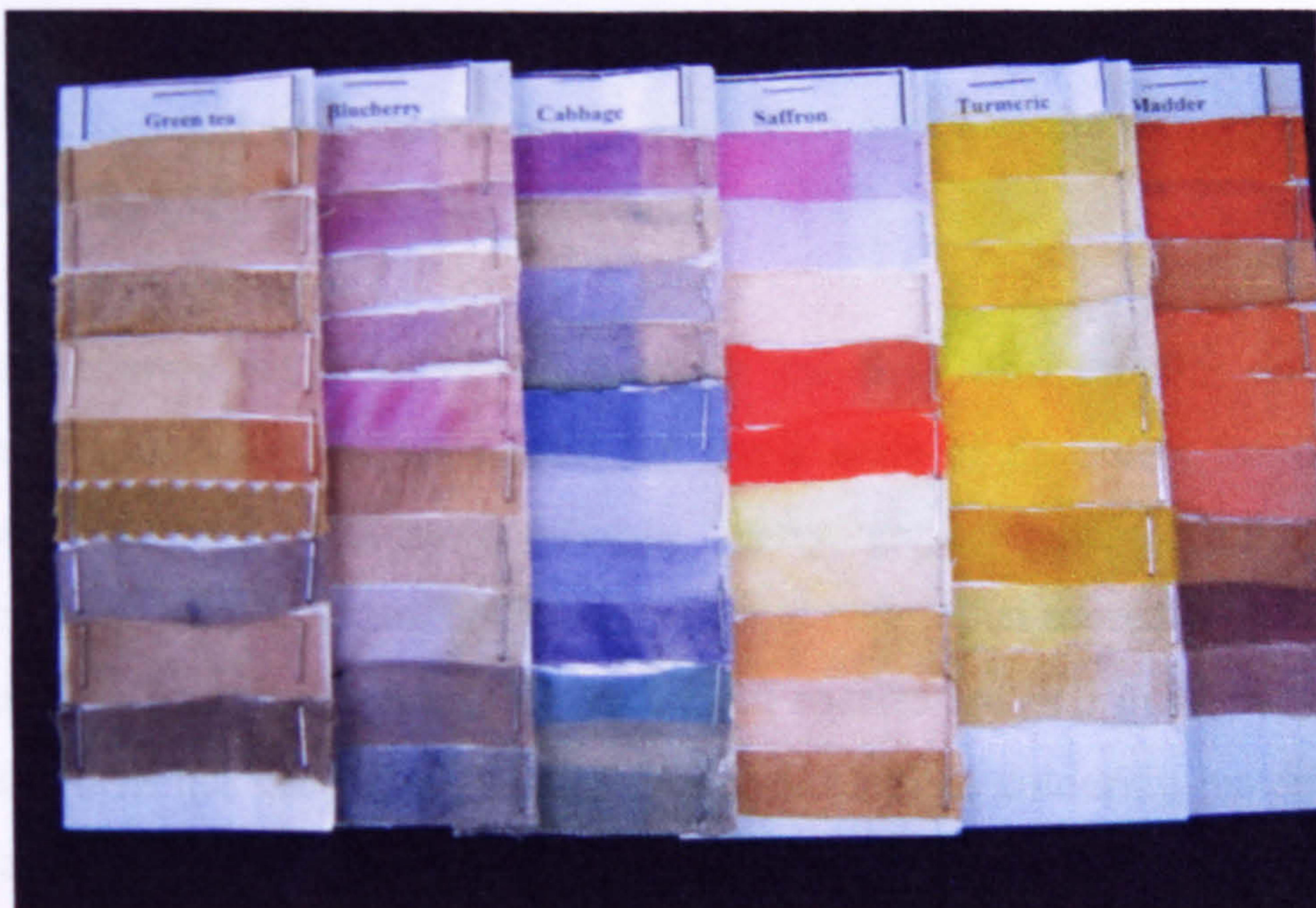
Plate 5.6: Some dyed samples against Blue Wool Standards after exposed to natural daylight
