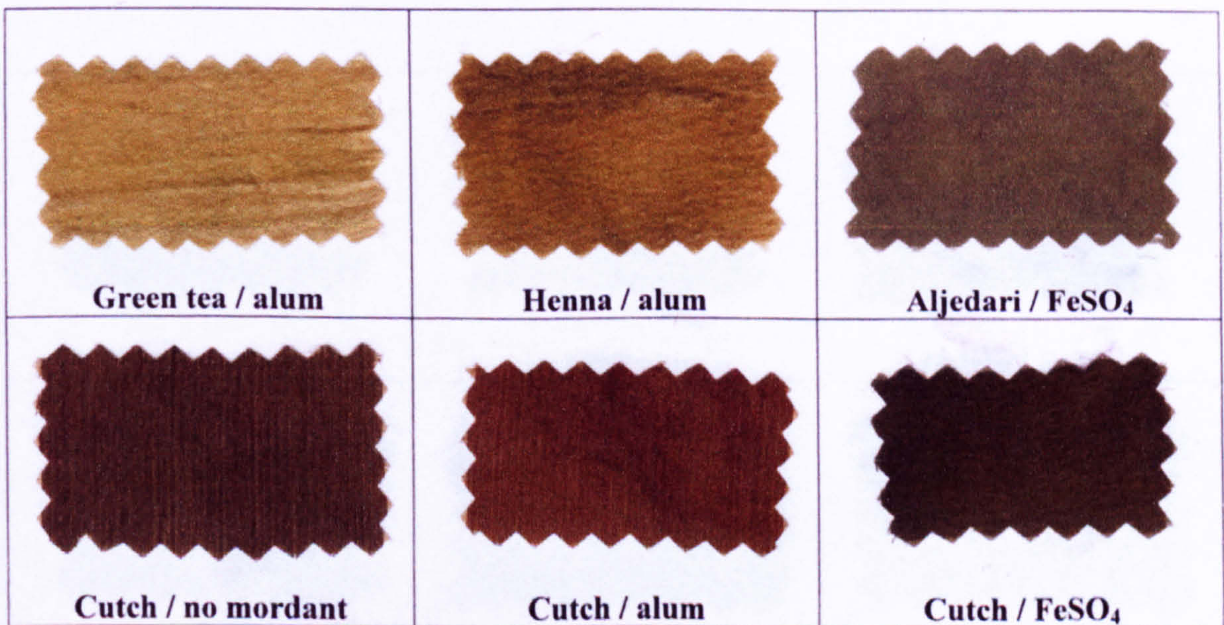
Plate 5.12: Samples of satin fabric dyed with aqueous extracts of plants yielded brown shades
