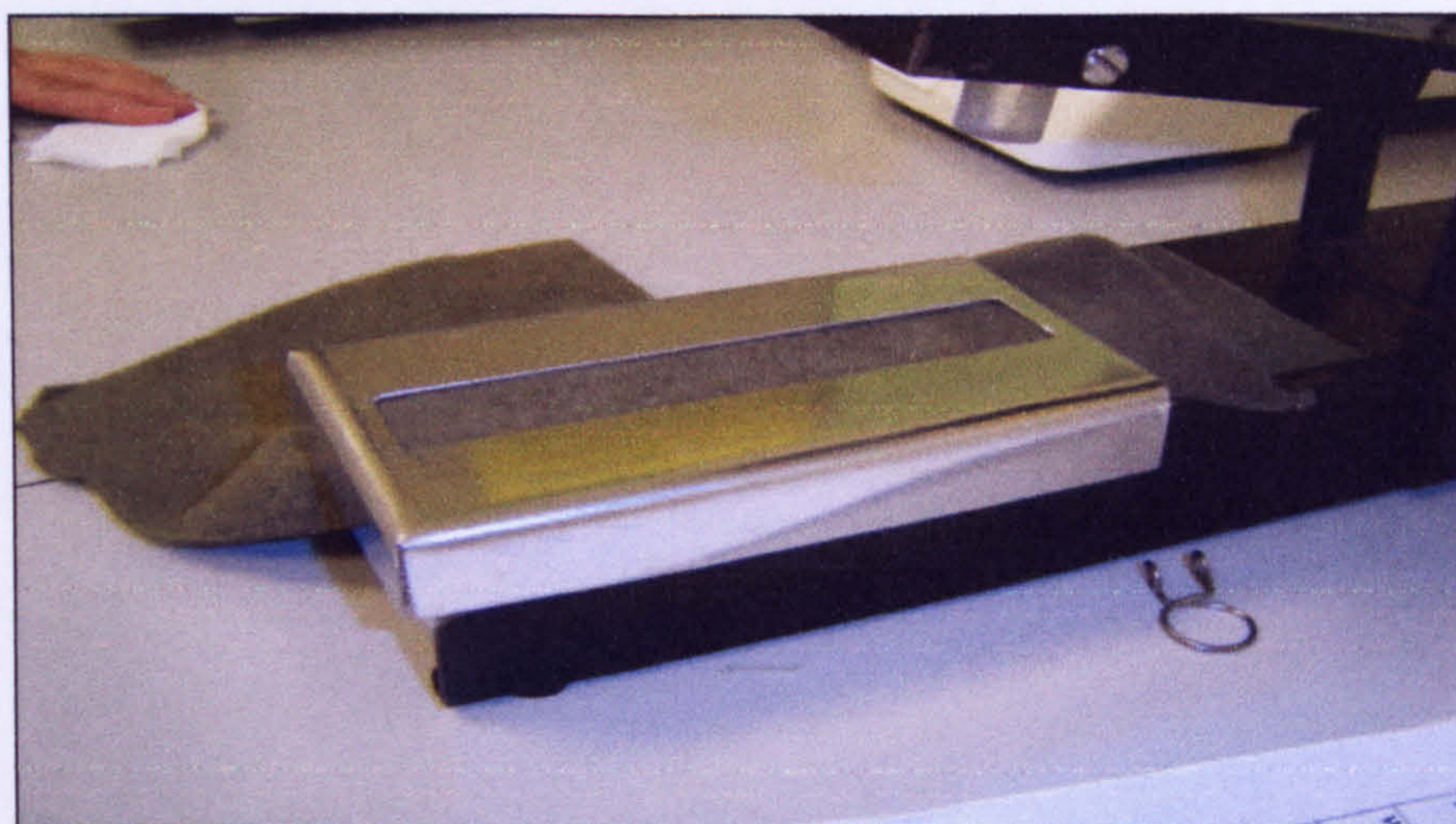
Plate 2.9: Rubbing tester against fabric for colour fastness
