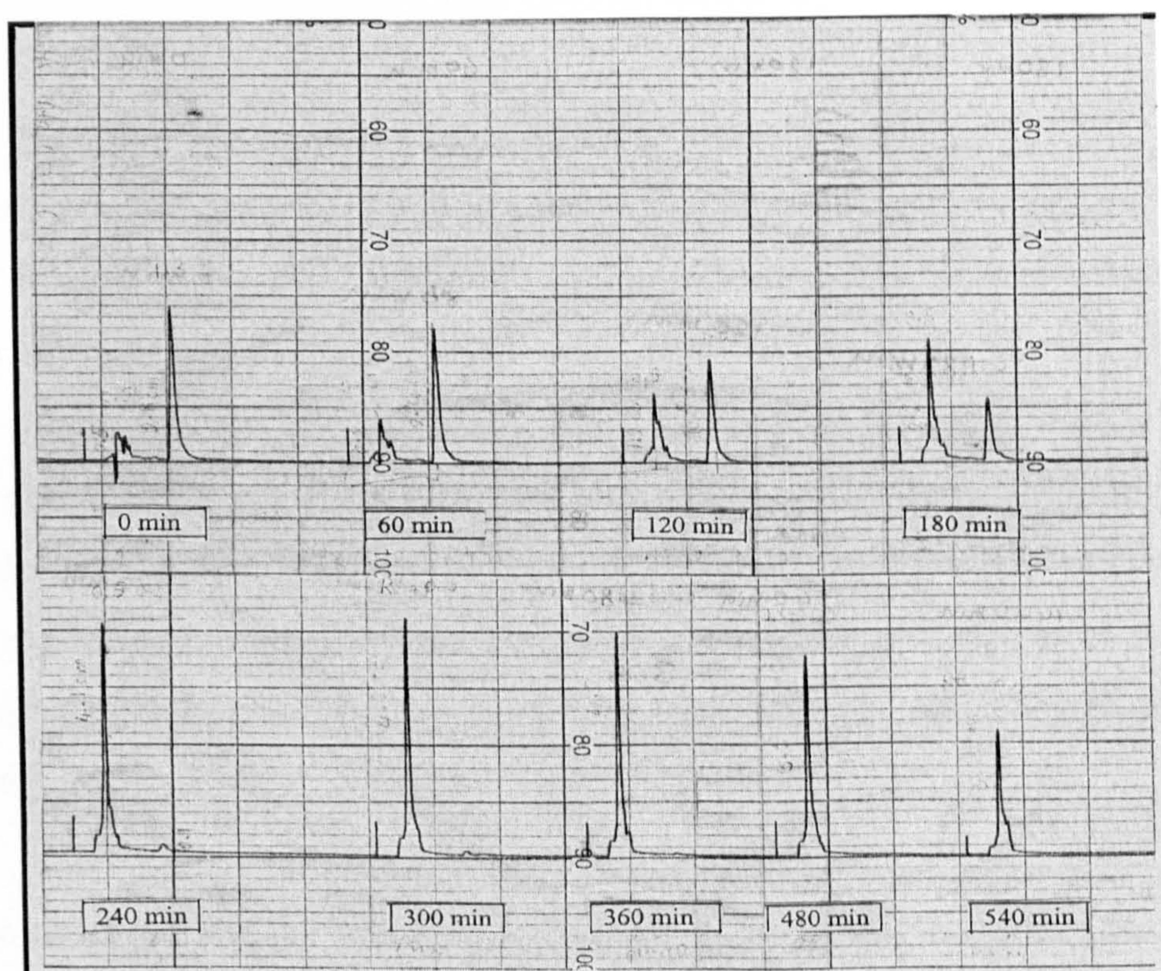
Figure 3.6: HPLC chromatogram during the electrolysis of MB in aqueous \text{Na}_2\text{CO}_3 solution at 340 nm. (Solvent; acetonitrile: \text{H}_2\text{O} (90:10), sensitivity: 0.1)
