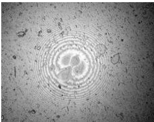
Figure 72: Di-urea grease PAO 30 Green light image taken before the tests
