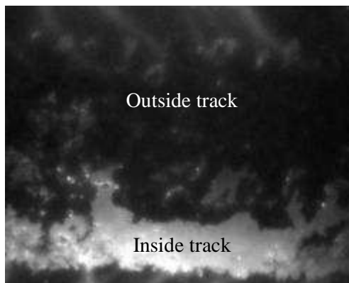
Figure 81: Di-urea grease PAO 30 Fluorescence image of the ball track after the tests were finished
