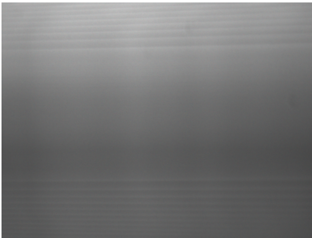
Figure 104: Interferogram for Cr only disc with a thickness of ~15nm with a 20N load
