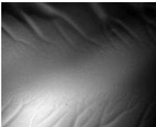
Figure 70: LiSt grease PAO 30 Fluorescence image of the disc track after the tests were finished
