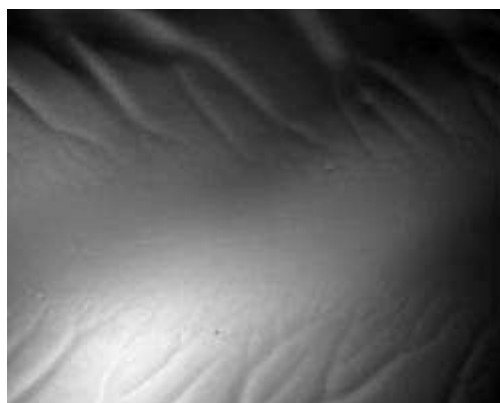
Figure 65: LiSt grease PAO 30 Fluorescence image of the disc track after the tests were finished
