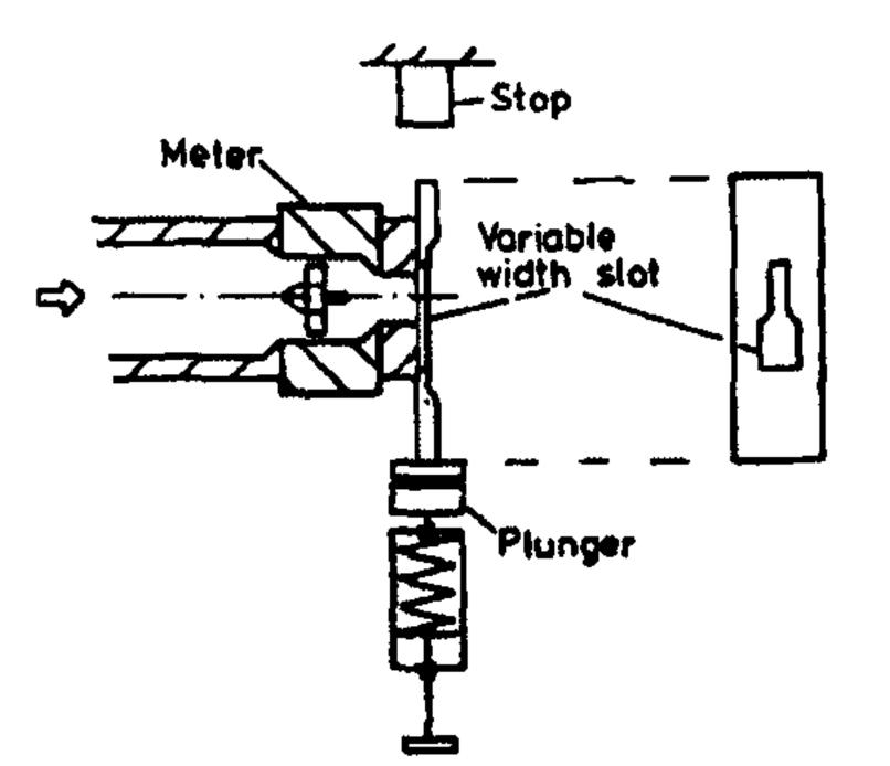
Figure B. 2 Details of the variable-area orifice used to produced changes in the flow
