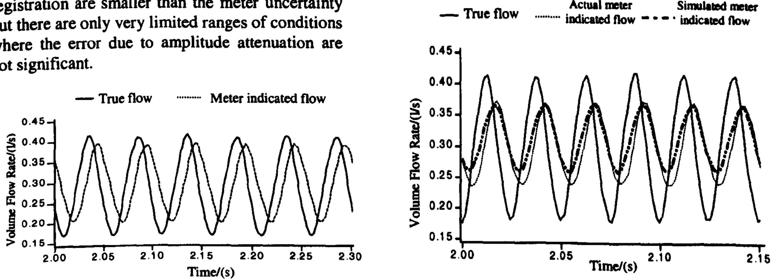
Comparison of true flow and meter indicated flow Figure 3 at 20Hz imposed pulsation with 40% relative pulsation amplitude
