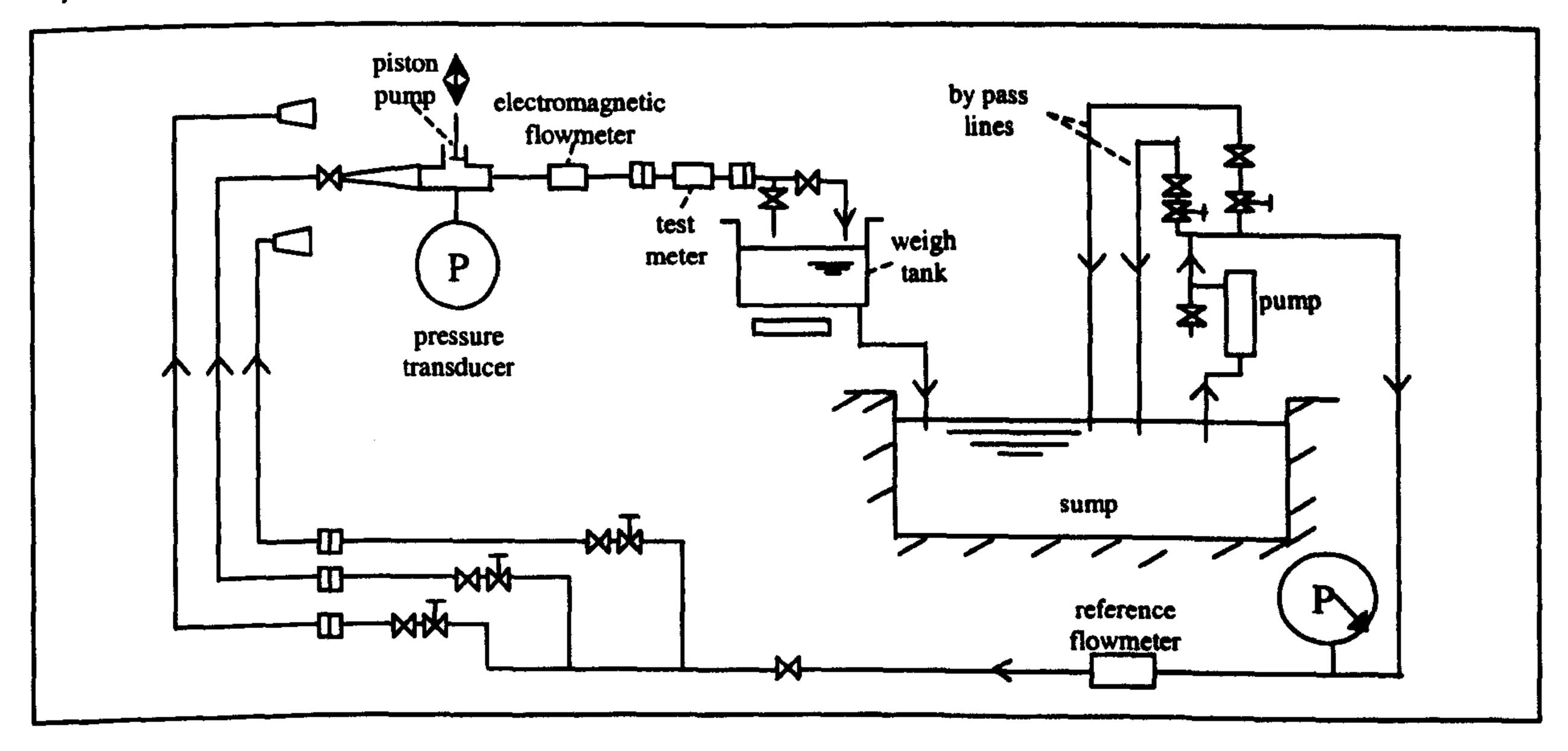
Figure 1 A schematic diagram of the test rig
