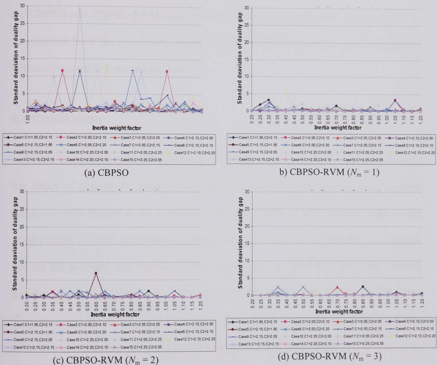
Figure 6.18 Comparison of standard deviation of duality gap between CBPSO and CBPSO-RVM for UC problem
