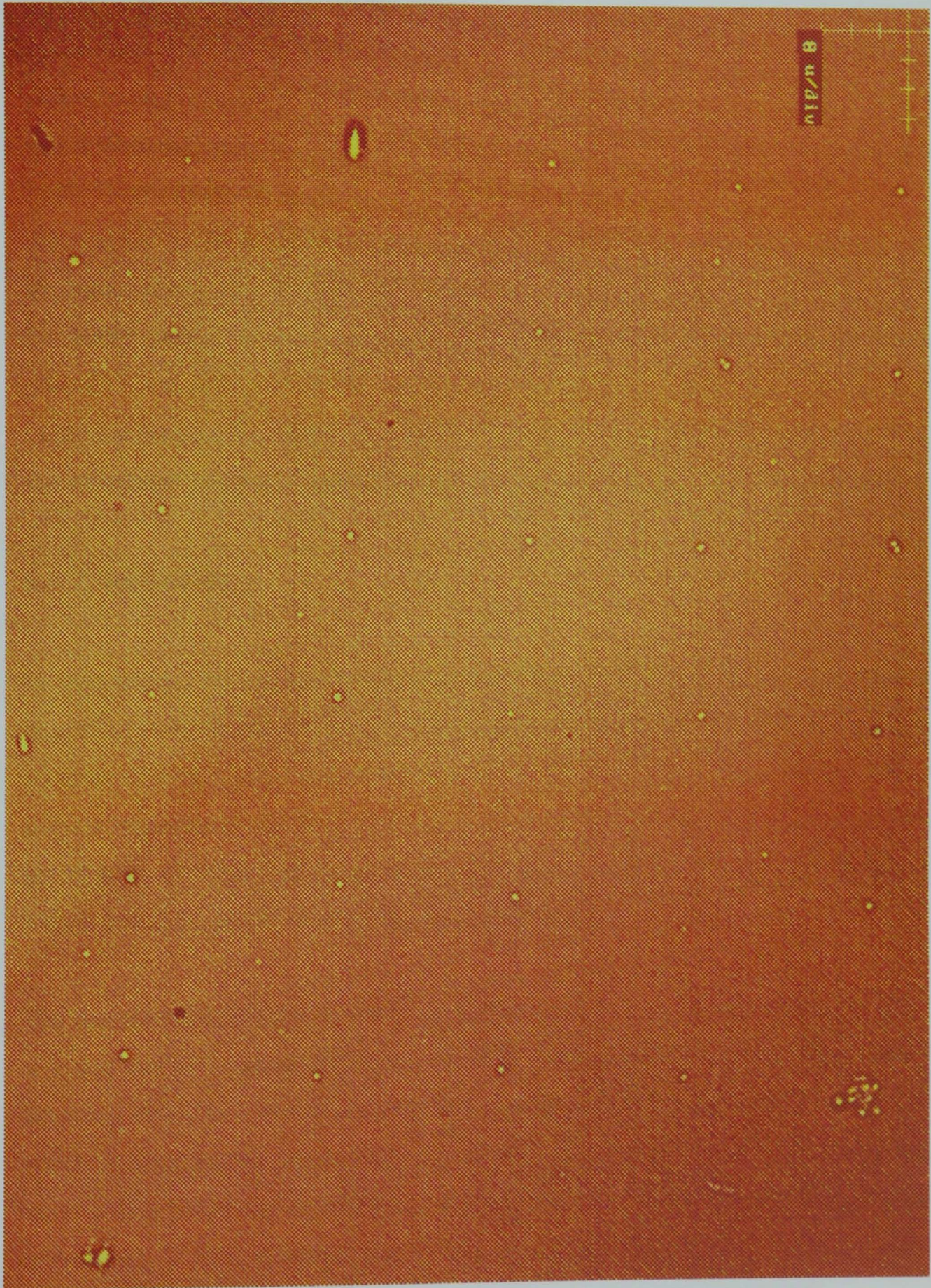
Figure 6.7 The results, in CR39 track etch plastic, of repeated single irradiations of 1 proton per point in a 50 \mu\text{m} spacing grid.
