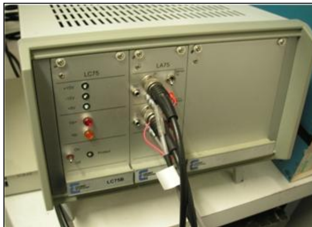
Figure 3.4: Piezo-electric power amplifier from Cedrat SA
