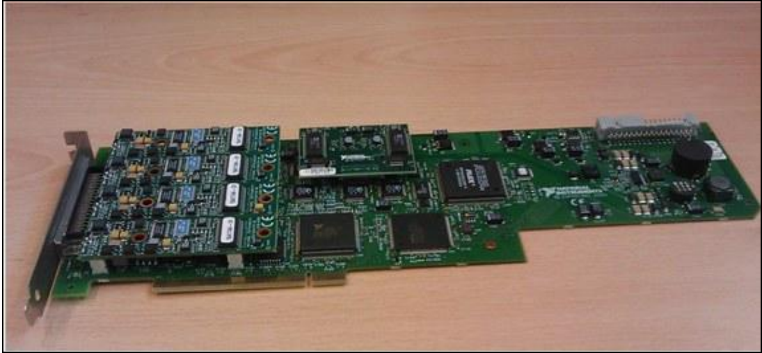
Figure 3.8: DAQ card from the National Instrument
