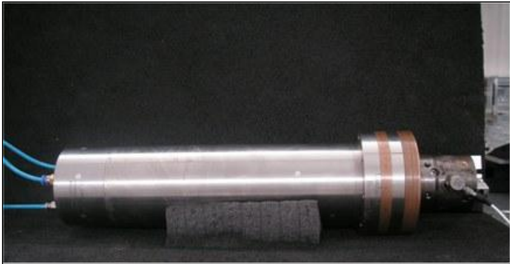
Figure 3.5: Air bearing spindle from Loadpoint LTD
