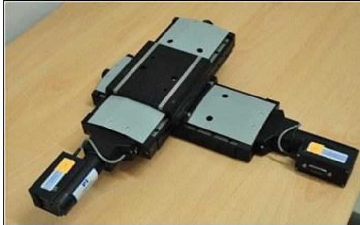
Figure 3.7: X slideway driven by leadscrew
