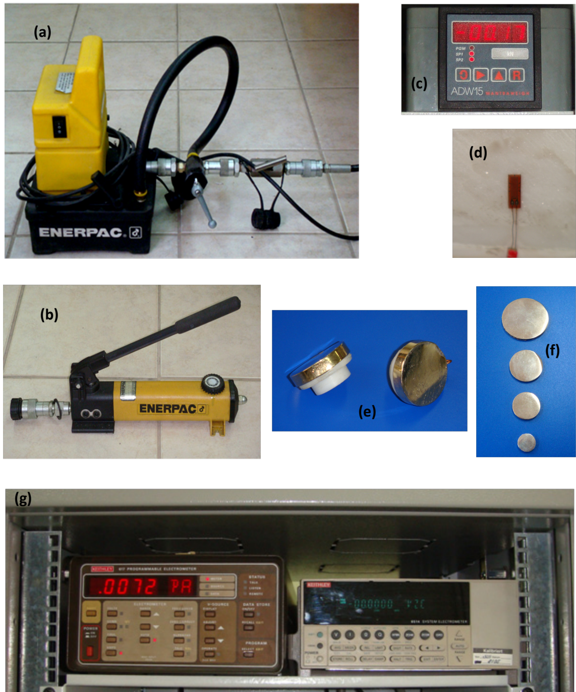
Figure B-1. (a) Electric hydraulic pump Enerpac PUJ-1200, (b) manual hydraulic pump (Enerpac P-142) (c) weighing indicator/controller ADW15 (d) strain gage sensor from Kyowa KFG series attached by adhesive on the electrode free surface of marble sample (e) golden plated electrodes with teflon interface for attachment to the samples with springs (f) mechanically stimulated electric signal sensing elements of various size - golden plated or copper made for attachment on specimens by rubber or adhesives (e) Programmable electrometers for mechanically stimulated electric signal measurements Keithley 617 and Keithley 6514
