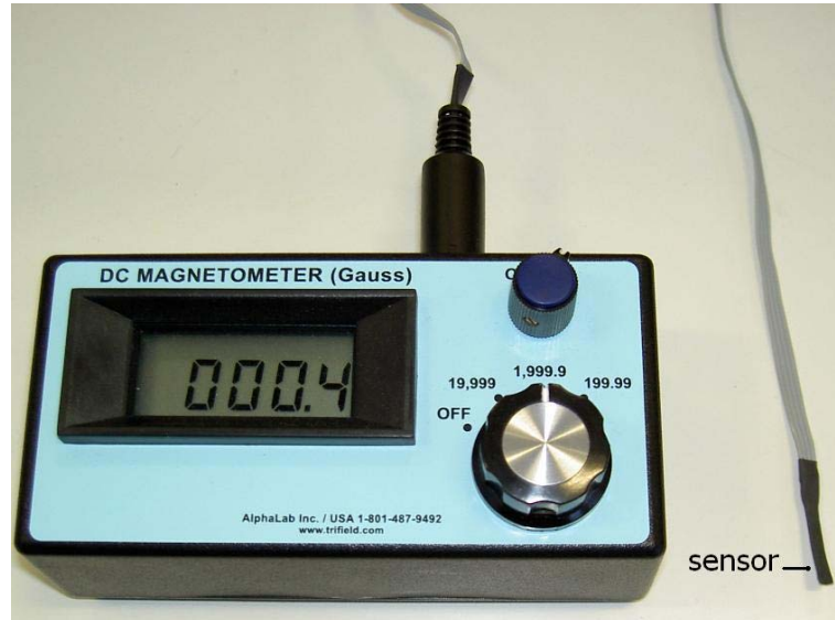
Figure 6.1. A photograph of the magnetometer used in the experiment to measure the magnetic flux density of external coils.
