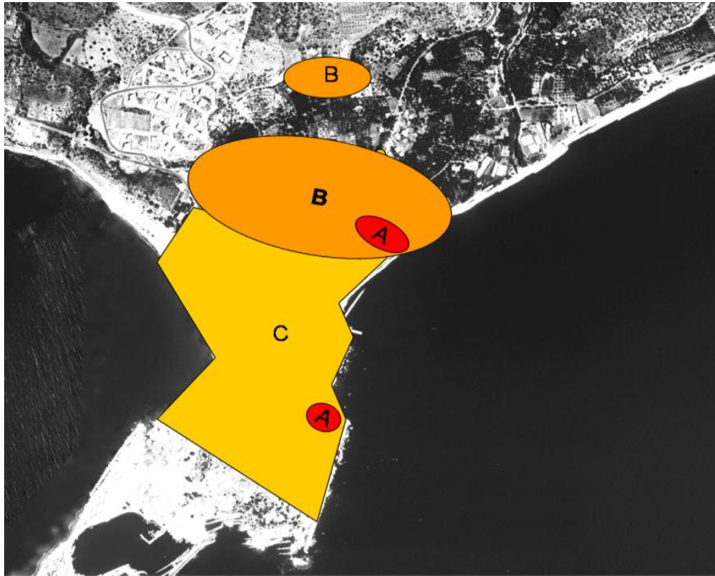
Figure 4.3.5: Ground seismic amplification map in Paleohora basin. The red zones (A) represent sites with the higher amplification (5.68, 5.75). The orange zone (B) represents sites of ground amplification ranging from 3.0-4.66. The yellow area zone (C) represents sites of ground amplification 1.88-3.36.
