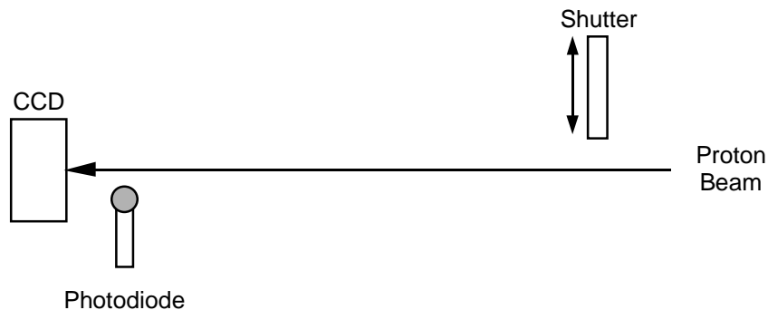
Figure 4.5 A schematic of the Birmingham cyclotron beamline
