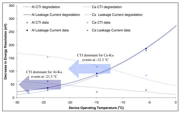
**Figure 6.19:** Decrease in energy resolution resulting from increased CTI and dark current as a function of temperature after  $7.5 \times 10^8$  protons.cm<sup>-2</sup> for Al-K $\alpha$  and Ca-K $\alpha$  X-ray events showing the point at which CTI becomes dominant
