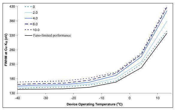
**Figure 4.29:** Measured energy resolution of isolated Cu-K $\alpha$  events found using different threshold multipliers as a function of temperature
