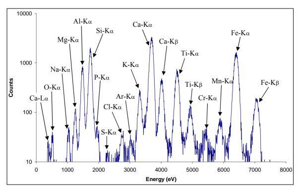
Figure 7.14: Icelandite spectrum recorded over 15 minutes with counts on a logarithmic scale
