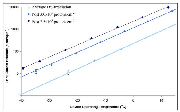
**Figure 6.10:** Estimated dark current as a function of temperature found using the square of the system noise subtracted from the square of the measured noise
