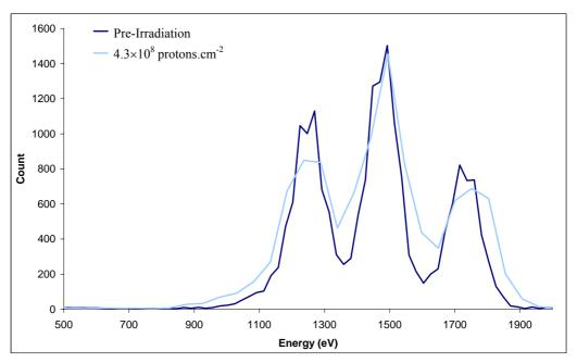
Figure 5.23: X-ray spectra produced using an Mg, Al and Si target between -40.0 °C
