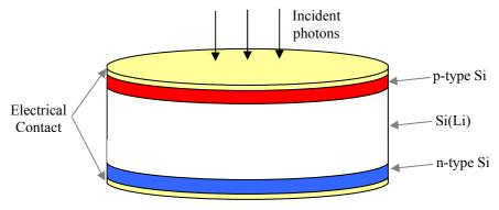
Figure 2.39: Silicon Lithium Detector
