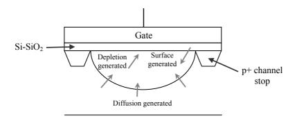
Figure 2.20: Source regions of dark current within a CCD [adapted from Janesick 2001]
