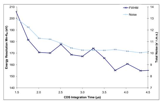
Figure 4.19: FWHM and noise as a function of integration time
