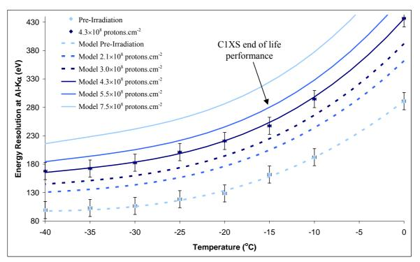
Figure 5.18: Modelled and experimental energy resolution at Al-K $\alpha$  as a function of temperature
