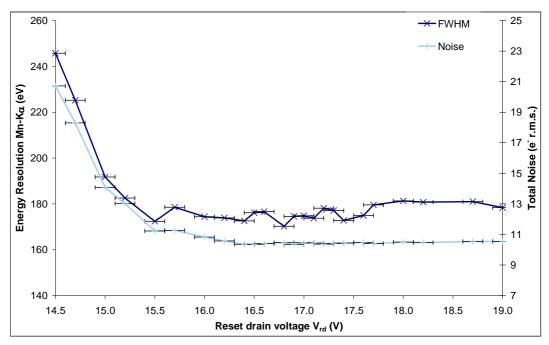
Figure 4.11: FWHM and noise as a function of  $V_{rd}$
