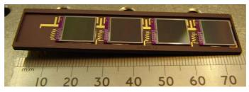
Figure 1.5: SCD module, used in both D-CIXS and C1XS, composed of four CCD54 devices
