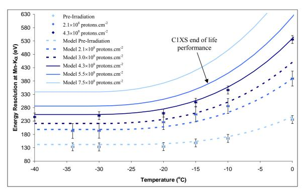
Figure 5.19: Modelled and experimental energy resolution at  $Mn-K\alpha$  as a function of temperature
