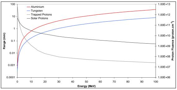
**Figure 3.11:** The range of protons in Al and Ta and the expected C1XS fluence of trapped and solar protons as a function of proton energy
