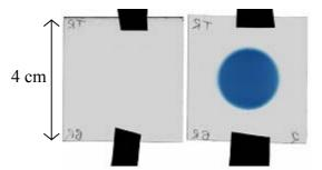
**Figure 6.5:** HD-810 Dosimetric film, showing an un-irradiated sample on the left and one held over the beam exit during an irradiation on the right
