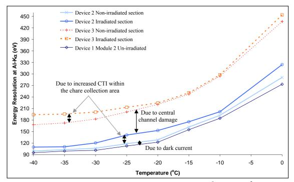
**Figure 5.10:** FWHM of Al-K $\alpha$  X-rays pre-irradiation and post  $4.3 \times 10^8$  protons.cm<sup>-2</sup> of device 2 and 3 as a function of temperature
