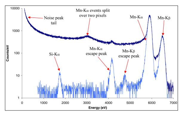
**Figure 2.34:** Calibrated spectrum of all and isolated events produced as a result of Mn-K $\alpha$  and Mn-K $\beta$  X-ray photons, illustrating the noise peak, split events and the Mn-K $\alpha$  escape peak
