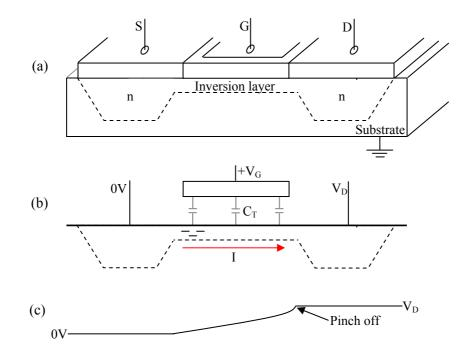
Figure 2.11: The metal-oxide semiconductor field-effect-transistor: (a) Basic structure of a MOSFET, (b) Cross-section showing the direction of electron flow and the FET capacitance  $C_o$ , (c) The potential difference felt by electrons as they move to the drain
