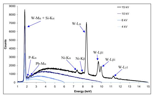
Figure 7.7: Incident X-ray spectra with varying tube potential
