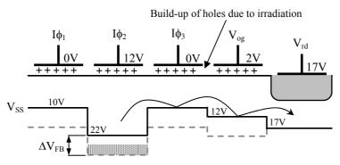
**Figure 3.18:** The result of a radiation induced flat-band voltage shift near the output gate with the potentials marked by solid lines pre-irradiation and dashed post-irradiation
