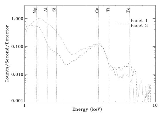
**Figure 1.3:** Instantaneous spectra from facets 1 and 3, showing the emission from Ca, Fe, Mg, Al, and Si obtained over ~2 minutes centred at 06:15 UT. Facet 3 was over the centre of Mare Crisium.
