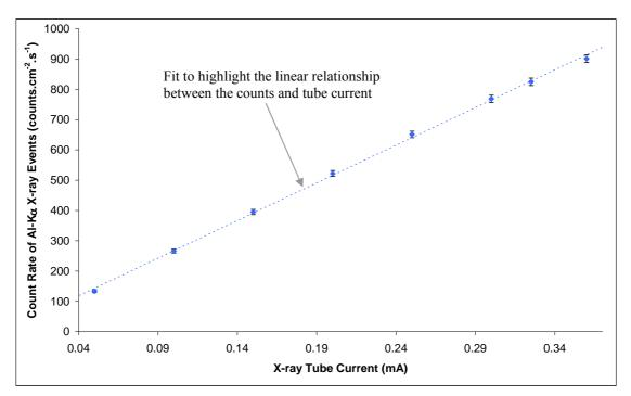
Figure 5.17: Al-K $\alpha$  events as a function of tube current
