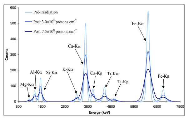
Figure 6.25: Model of Lunar Regolith Simulant spectra at -20 °C pre- and post-irradiation
