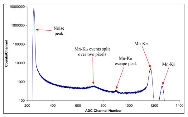
Figure 2.33: Raw spectrum produced as a result of Mn-K $\alpha$  and Mn-K $\beta$  X-ray photons, illustrating the noise peak, split events and the Mn-K $\alpha$  escape peak
