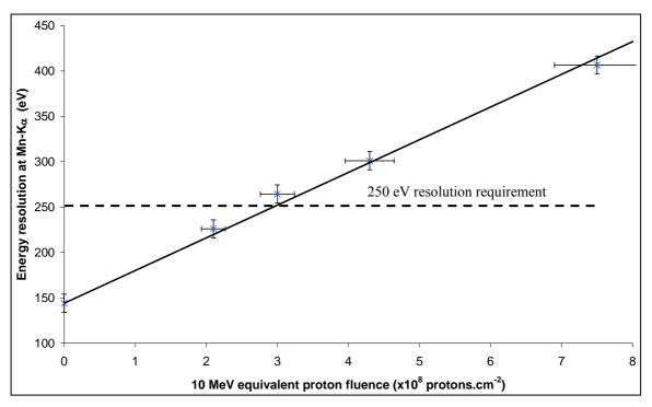
**Figure 6.21:** The measured Mn-K $\alpha$  event resolution at -20.0 °C found using a multiplier of 2 as a function of the 10 MeV equivalent proton fluence delivered to the CCD54
