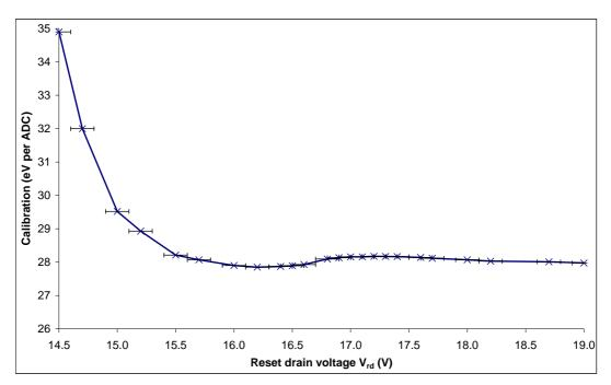
**Figure 4.12:** eV per ADC as a function of  $V_{rd}$
