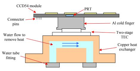
Figure 4.3: A schematic of the CCD54 mounting within the vacuum chamber
