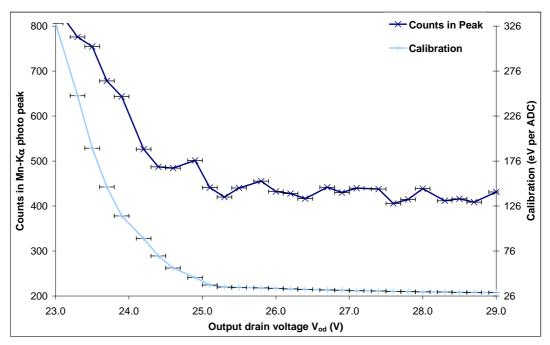
Figure 4.16: Counts in the peak and eV per ADC as a function of  $V_{od}$
