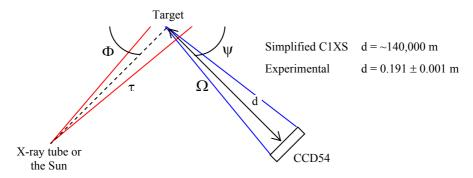
**Figure 7.1:** Geometry of the laboratory experiment with the angle of incidence and angle of emergence at 45°
