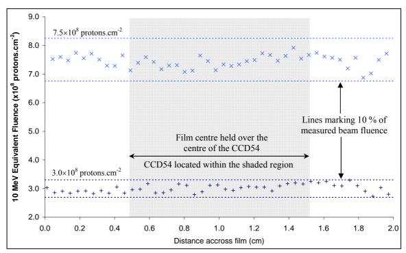
Figure 6.8: Measured proton beam fluence as a function of distance across the target area
