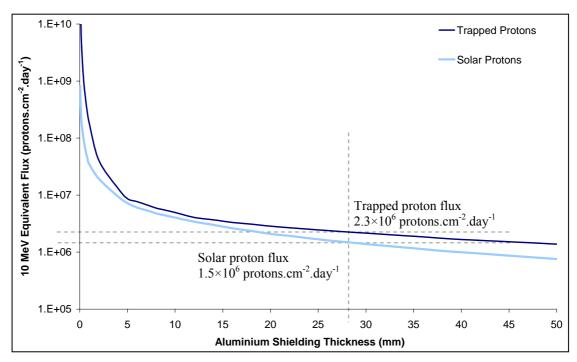
Figure 5.3: 10 MeV proton flux as a function of shielding thickness
