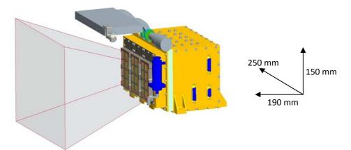
Figure 1.6: CAD image of the C1XS instrument, highlighting the 14° field of view [image courtesy of RAL]
