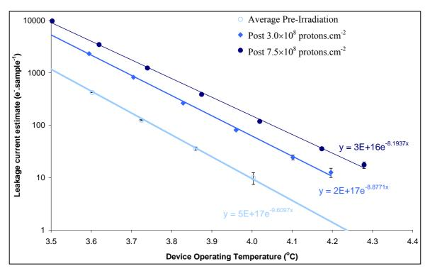
Figure 6.12: Arrhenius plot of dark current as a function of 1000/T for pre-irradiated and devices 3 and 4 irradiated to 3.0 and 7.5×10<sup>8</sup> protons.cm<sup>-2</sup> respectively
