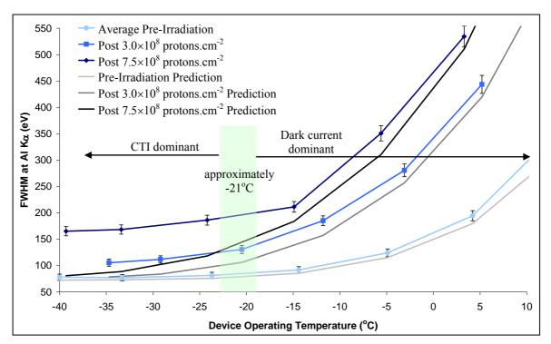
**Figure 6.16:** Measured energy resolution of Al-K $\alpha$  events pre- and post-irradiation as a function of temperature, and the predicted value based on Fano-limited statistics plus the measured read noise
