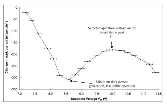
Figure 4.18: Decrease in dark current as a function of  $V_{ss}$
