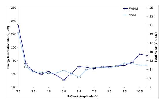
Figure 4.13: FWHM and total noise as a function of Reset-clock voltage
