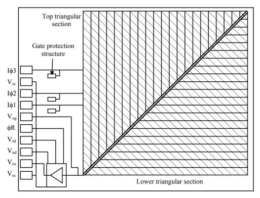
Figure 2.18: Schematic of the SCD. The electrodes are depicted as dashed lines, whilst the charge transport channels are indicated using solid lines
