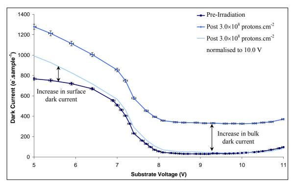
Figure 6.11: Estimated dark current as a function of substrate voltage, device 3 held at -15.0 °C pre- and post-irradiation with  $7.5 \times 10^8$  protons.cm<sup>-2</sup>
