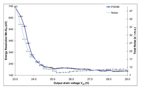
Figure 4.15: FWHM and noise as a function of  $V_{od}$
