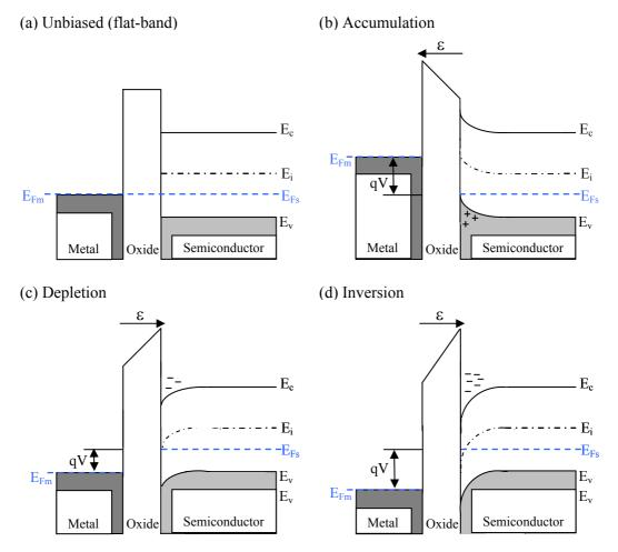
**Figure 2.8:** Band diagrams of MOS structure: (a) unbiased, (b) negative voltage applied causing accumulation, (c) positive voltage applied causing depletion, (d) positive voltage applied causing inversion
