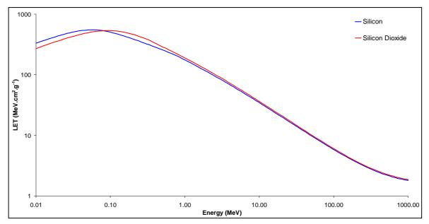
Figure 3.15: Linear energy transfer of Si and SiO<sub>2</sub> as a function of energy
