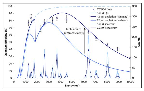
**Figure 4.34:** Measured quantum efficiency of the CCD54 and Si(Li) detector as a function of X-ray photon energy and the results from using Equation 2.47 to find the active depth. The spectra from the CCD54 and Si(Li) detector is also shown
