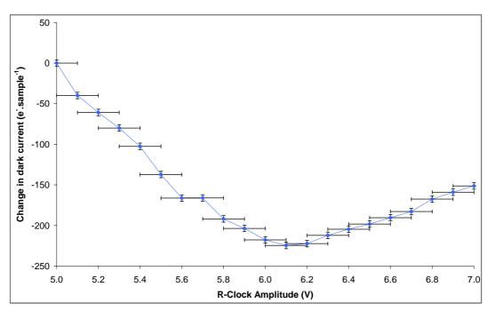
Figure 4.14: Relative change in dark current as a function of Reset-clock voltage
