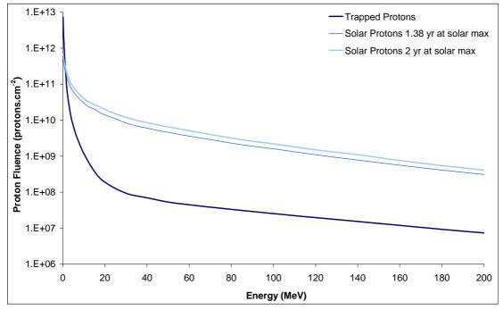
Figure 5.1: Proton fluence as a function of energy
