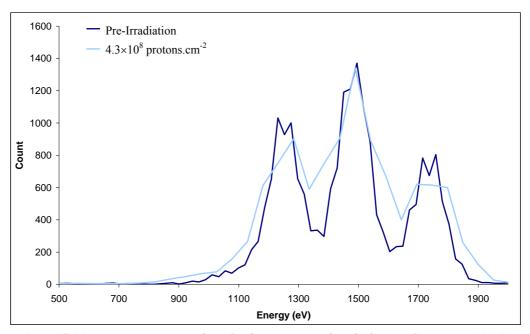
Figure 5.22: X-ray spectra produced using an Mg, Al and Si target between -30.0 °C
