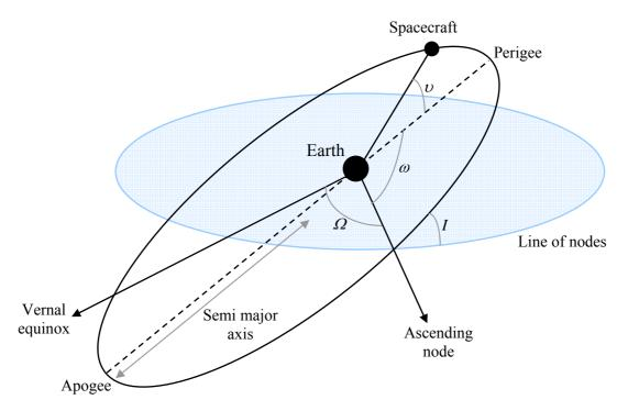
Figure 3.1: The Keplerian elements used to define the orbit of Chandrayaan-1 in SPENVIS
