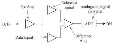
Figure 2.29: Basic CDS circuit
