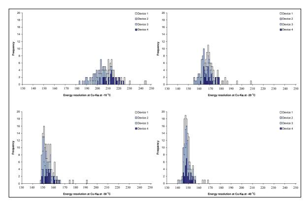
**Figure 4.25:** The FWHM of the Cu-K $\alpha$  X-ray peak from the ten best modules as a function of temperature
