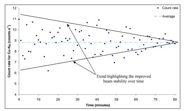
Figure 4.31: Count rate of Cu-Ka X-rays as a function of time over 90 minutes after powering up
