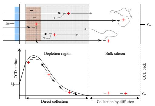
Figure 2.30: Illustration of charge generation and collection for a front side illuminated device
