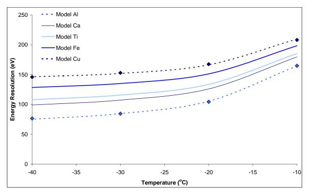
Figure 4.27: Theoretical FWHM as a function of temperature compared with experimental data from a copper and aluminium target
