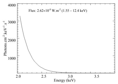
Figure 7.4: Solar spectrum recorded over 240 s using the XSM mounted onboard Chandrayaan-1 on the 10<sup>th</sup> of January 2009 [Alha 2009]
