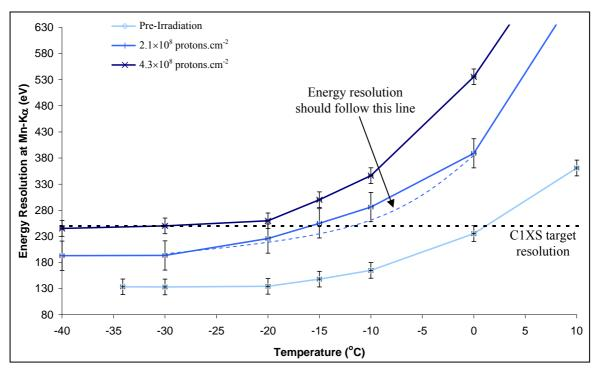
Figure 5.8: FWHM of Mn-Ka X-rays pre- and post-irradiation as a function of temperature
