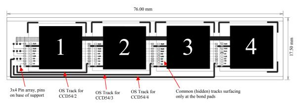
Figure 4.1: Schematic of a C1XS module showing the device number scheme [adapted from Hotston 2000]
