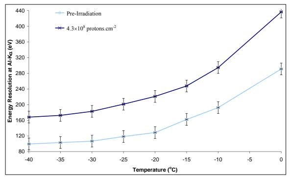
Figure 5.7: FWHM of Al-Ka X-rays pre- and post-irradiation as a function of temperature
