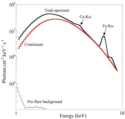
**Figure 7.3:** Solar spectrum from the Si PIN detector onboard MESSENGER, showing the pre-flare background and a solar flare which occurred on the 1<sup>st</sup> of June 2007 [adapted from Dennis 2008]
