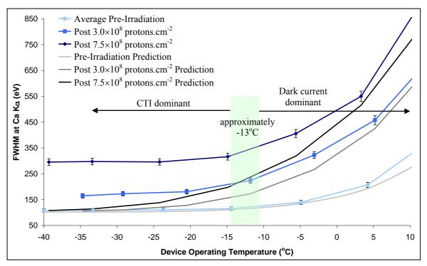
**Figure 6.17:** Measured energy resolution of Ca-K $\alpha$  events pre- and post-irradiation as a function of temperature, and the predicted value based on Fano-limited statistics plus the measured read noise
