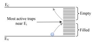
Figure 2.19: Silicon band-gap showing the location of the most active trap sites or defect locations
