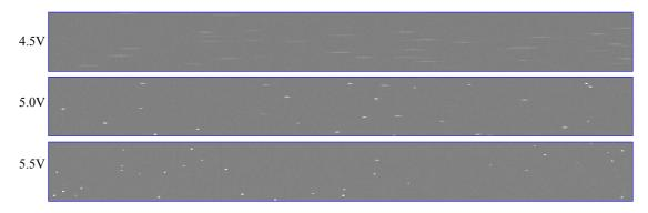
**Figure 4.6:** 100 read-outs of the CCD54 showing the resulting 575 samples taken using an I-clock of 4.5 V, 5.0 V and 5.5 V
