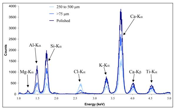
Figure 7.9: Spectra from different Etna basalt targets, with grain sizes between 250 and 500  $\mu$ m, >75  $\mu$ m, and a polished surface
