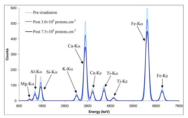
Figure 6.26: Model of Lunar Regolith Simulant spectra at -20 °C pre- and post-irradiation, not including the CTI damage factor
