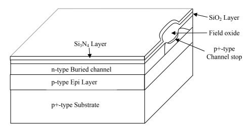
Figure 2.14: Cross section of in initial stages of CCD fabrication showing the substrate and the epitaxial layer
