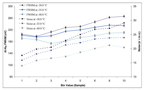
**Figure 5.13:** Energy resolution of Al-K $\alpha$  X-rays and total noise as a function of sample binning
