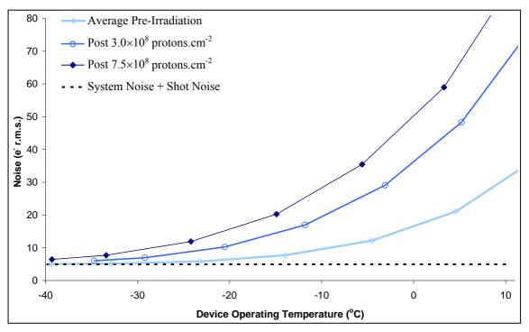
Figure 6.9: Measured noise as a function of temperature for devices 2, 3 and 4
