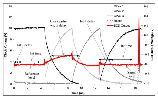
Figure 2.28: The CCD54 output trace before entering the drive box and the clock waveform used to drive the device
