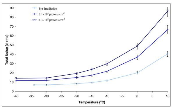
Figure 5.9: Noise pre- and post-irradiation as a function of temperature
