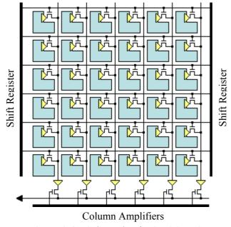
Figure 2.41: Schematic of a CMOS APS
