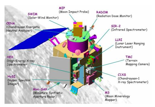
Figure 1.4: Schematic of the Chandraayan-1 spacecraft [ISRO]
