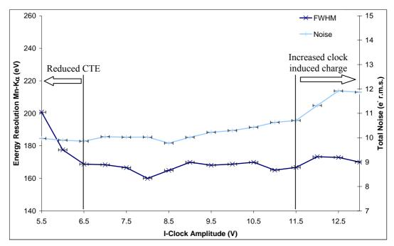
Figure 4.7: FWHM and total noise as a function of I-clock voltage
