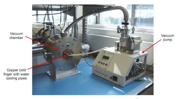
Figure 4.2: A photograph of the SCD test facility while using an <sup>55</sup>Fe source
