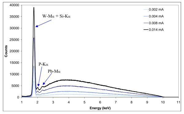
Figure 7.8: Incident X-ray spectra with varying tube current
