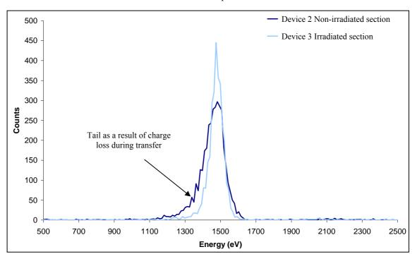
**Figure 5.12:** Spectra of Al-K $\alpha$  X-rays post  $4.3 \times 10^8$  protons.cm<sup>-2</sup> taken using the non-irradiated section of device 2 and irradiated section of device 3 at -25 °C
