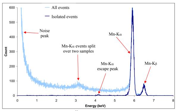
Figure 4.5: Spectrum recorded using the <sup>55</sup>Fe source using all and isolated events with the CCD54 held at -20.0 °C
