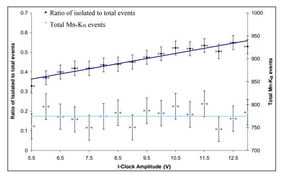
Figure 4.9: Ratio of split and isolated events and the total events as a function of I-clock voltage
