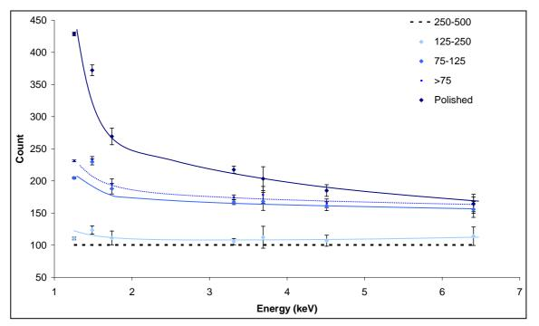
**Figure 7.11:** Counts in the X-ray peaks from different particle sizes of Icelandite, normalised to provide 100 counts from the target with particles between 250 and 500 μm in diameter
