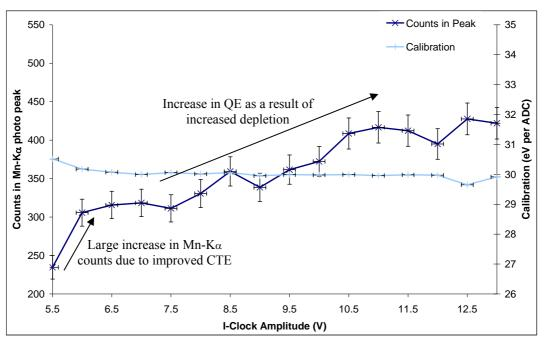
Figure 4.8: Counts in the peak and eV per ADC as a function of I-clock voltage
