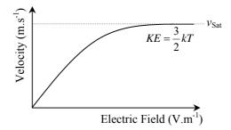
Figure 2.23: Illustration of electric field versus the electron velocity showing the saturation velocity  $v_{Sat}$
