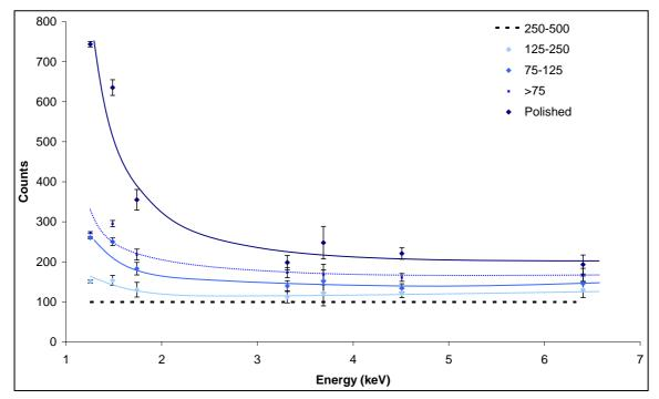
**Figure 7.10:** Counts in the X-ray peaks from different particle sizes of Etna basalt, normalised to provide 100 counts from the target with particles between 250 and 500 μm in diameter
