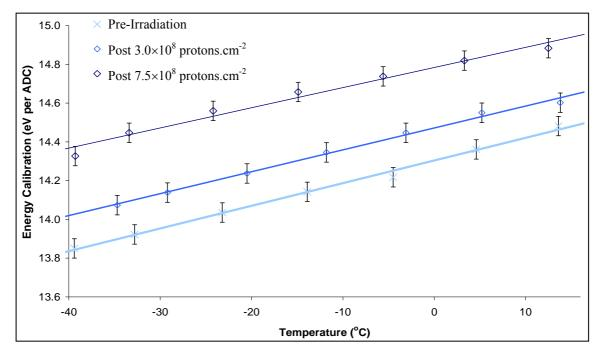
Figure 6.14: Calibration found using Cu-Ka events as a function of temperature
