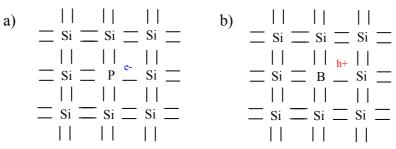
Figure 2.4: The lattice structure within n-type (a) and p-type (b) silicon
