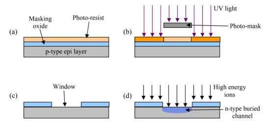
**Figure 2.15:** Illustration of the photolithography process involved in the creation of the n-type buried channel. Negative photo-resist is applied to a masking oxide on the p-type epitaxial layer (a) then exposed to UV light and developed (b). The remaining exposed photo-resist and masking oxide are etched to create a diffusion window (c) through which ion implantation is used (d) to create the n-type buried channel
