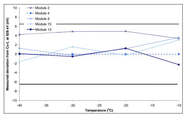
Figure 4.26: Module comparison of measured deviation in Cu-L energy vs. temperature, the lines mark  $\pm 1$  ADC channel ( $\pm 6.5$  eV)
