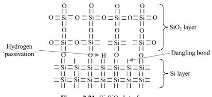
Figure 2.21: Si-SiO<sub>2</sub> Interface
