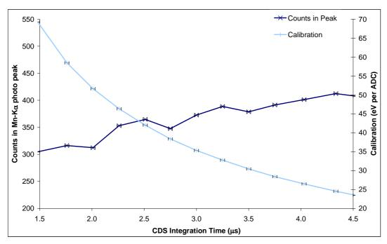
Figure 4.20: Counts in the peak and eV per ADC as a function of integration time
