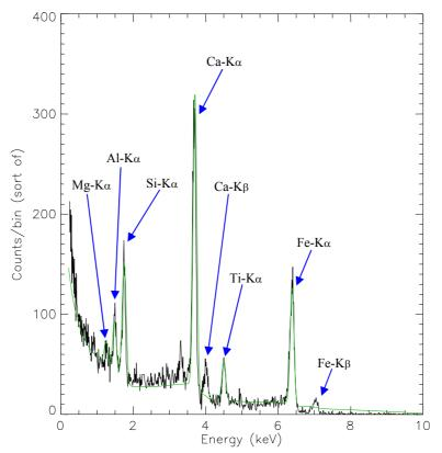
Figure 7.13: Initial results produced using the Swinyard code based on experimental data of the lunar regolith simulant [Swinyard 2008]
