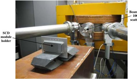
Beam exit with — 100 μm W scattering foil
