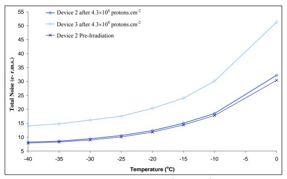
Figure 5.11: Total Noise pre-irradiation and post  $4.3 \times 10^8$  protons.cm<sup>-2</sup> of device 2 and 3 as a function of temperature
