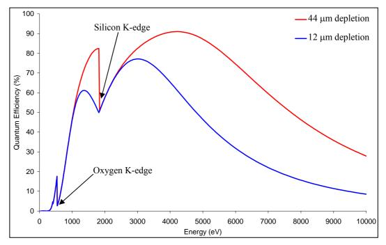
Figure 2.37: Quantum efficiency curve of the CCD54 with an active depth of 12  $\mu$ m and 44  $\mu$ m
