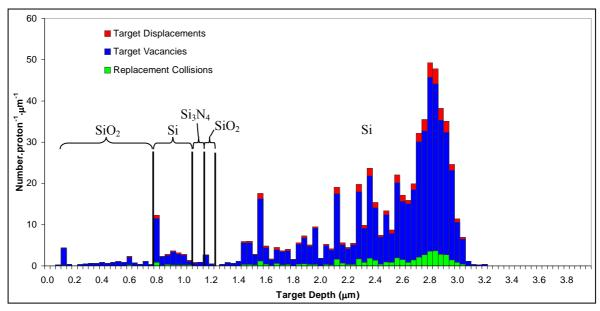
Figure 3.20: Displacement, vacancies and replacement collisions from 300 keV protons as a function of depth into the CCD54
