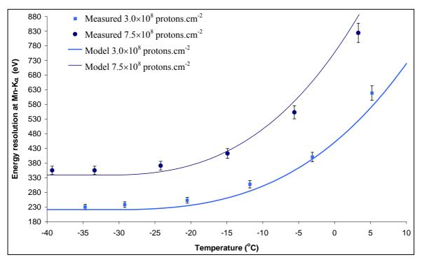
**Figure 6.20:** Comparison of the measured energy resolution found using the XCAM software and the initial model for 10 MeV equivalent proton fluences of  $3.0 \times 10^8$  and  $7.5 \times 10^8$  protons.cm<sup>-2</sup>
