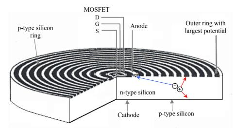
Figure 2.40: Schematic of a Silicon Drift Detector [adapted from Lechner et al. 2004]
