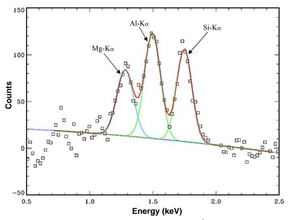
**Figure 7.19:** The first lunar spectrum recorded by C1XS on the 12<sup>th</sup> of December 2008 showing the Mg, Al and Si X-ray peaks fluoresced by an A-class solar flare [Kellet 2008]
