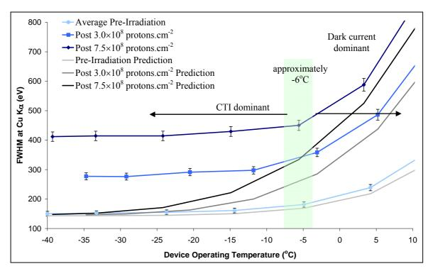
**Figure 6.19:** Measured energy resolution of Cu-K $\alpha$  events pre- and post-irradiation as a function of temperature, and the predicted value based on Fano-limited statistics plus the measured read noise
