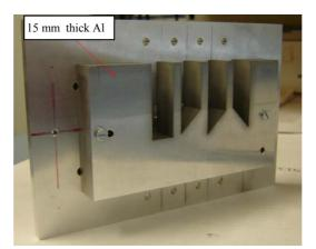
Figure 5.5: Proton irradiation jig and the aluminium shield
