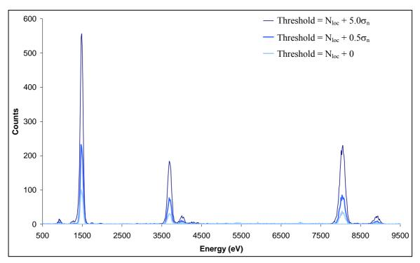
Figure 4.28: Spectra produced from an Al, Ca, and Cu target using different levels of threshold
