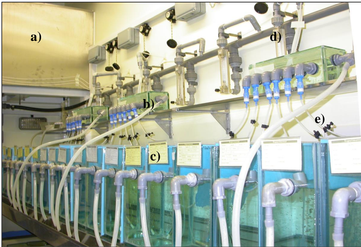
Figure 35. A photograph of one side of the experimental room. a) represents the header tank; b) shows the mixing vessels from which water from the header tank and propranolol from the stock bottles mixed before flowing into the individual fish tanks ( c ); d) indicates one of the flow meters; e) shows one of the clamps used to regulate water flow from the mixing vessel into each tank.
