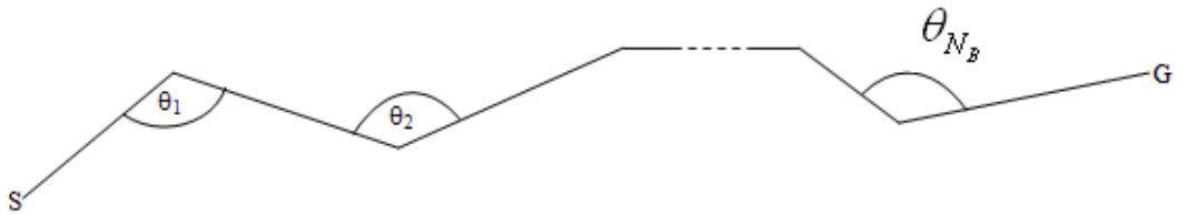
Fig. 5.3 A path between start (S) and end (E) nodes with bend angles
