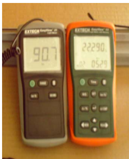
Figure 3.2 – The commercial photometers (illuminance meters) used in this research (a). Picture (b) shows the dome-diffuser detector of the photometers exposed to direct sunlight.
