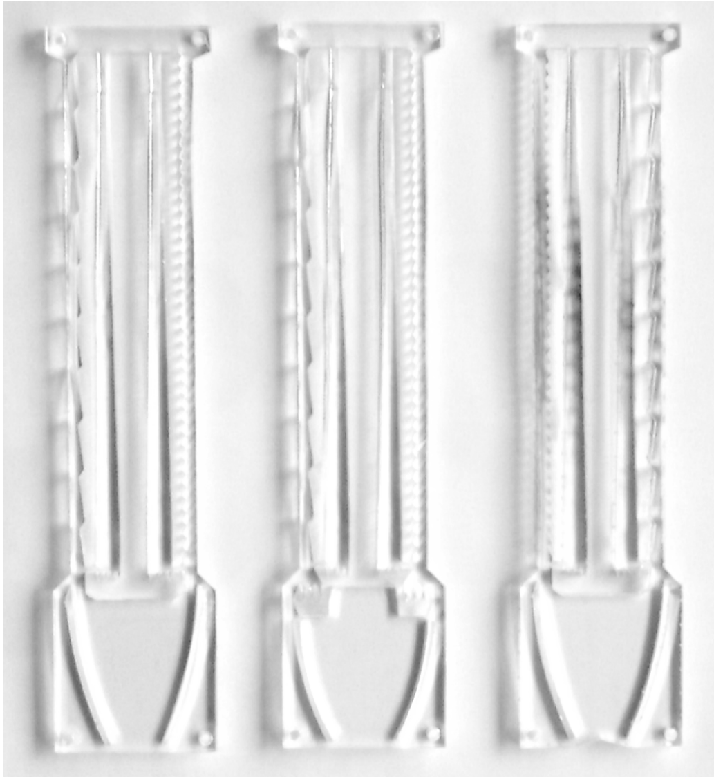
Figure 7.15 – IMPSC-D demonstration prototype sections (with double symmetrical integrated light guide, D-SILG).
